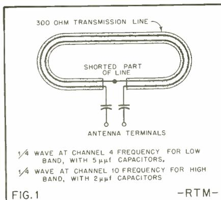
Conversely, when the diameter of the conductors is small, the L-C ratio is increased, with a resultant increase in the Q of the resonant circuit.
