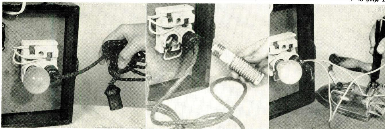
Appliance cord is tested for short circuits, below, left. Twisting and folding the cord will reveal an intermittent short if it is present. When the short contacts, the lamp will light. In the center, a heater unit, which draws about 10 times as much current as the lamp, is inserted
