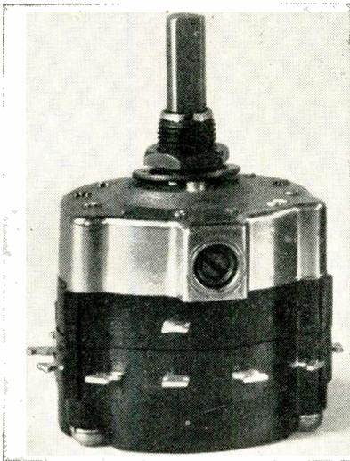
tion, the switch, which is a shorting type, has an adjustable detent, with a screw for setting torque to the exact pressure desired.
