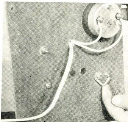
Prongs connected together behind the panel provide a test for appliance cords suspected of open circuits.
