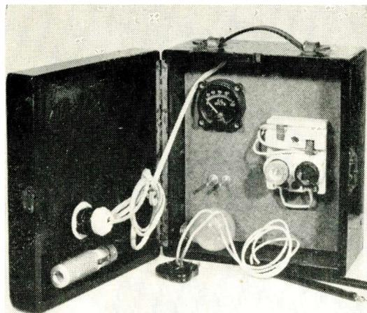
The complete home appliance tester in its case. AC voltmeter is optional, may be replaced with a pilot light to show when the tester is activated. Dummy receptacle in the lid of the case holds power plug when it is not in use.
