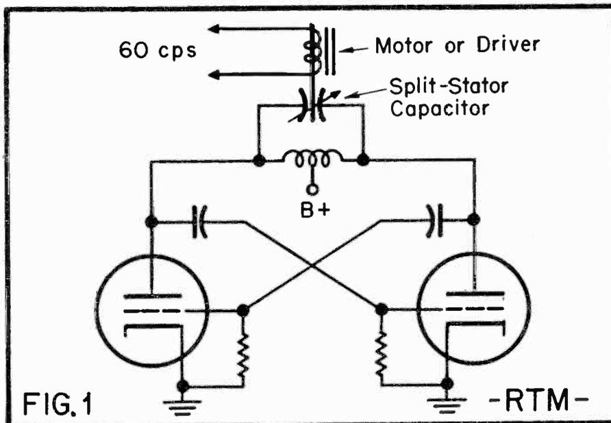
Rotating capacitor method of varying oscillator frequency. The motor, an 1800 or 3600 rpm synchronous type, drives the rotor of a continuously variable condenser. Capacitance varying constantly from minimum to maximum modulates oscillator frequency at 60 cycles.
