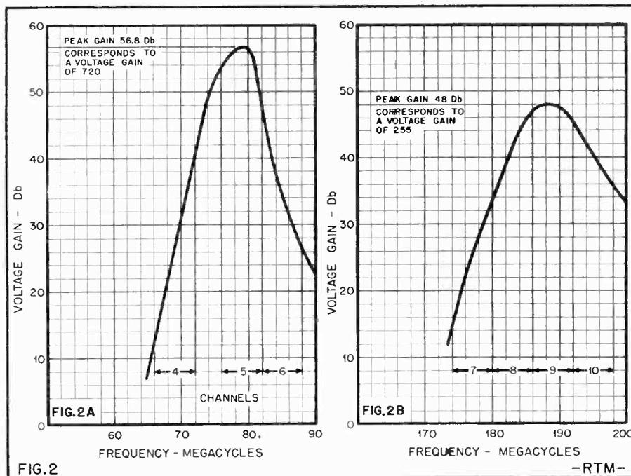
Typical response curves of amplifier strips. Each strip, including 5 6AK5's and a 6J6, is peaked for maximum gain in its channel, with sharp attenuation in neighboring channels.
