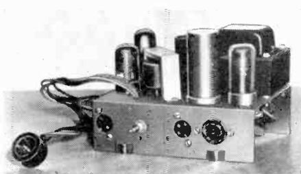
Projection picture tube (above), and auxiliary chassis, containing 7C5 video amplifier, 7Z4 rectifier, 7B6 for automatic biasing, and compensation for additional wiring and switch capacity used in the Duo-Vue system.
