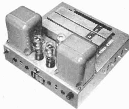
Fig. 1. Top view of control chassis used in the Mul-TV system. Individual channel gain controls are shown on the front of the chassis, output jacks on right side.
