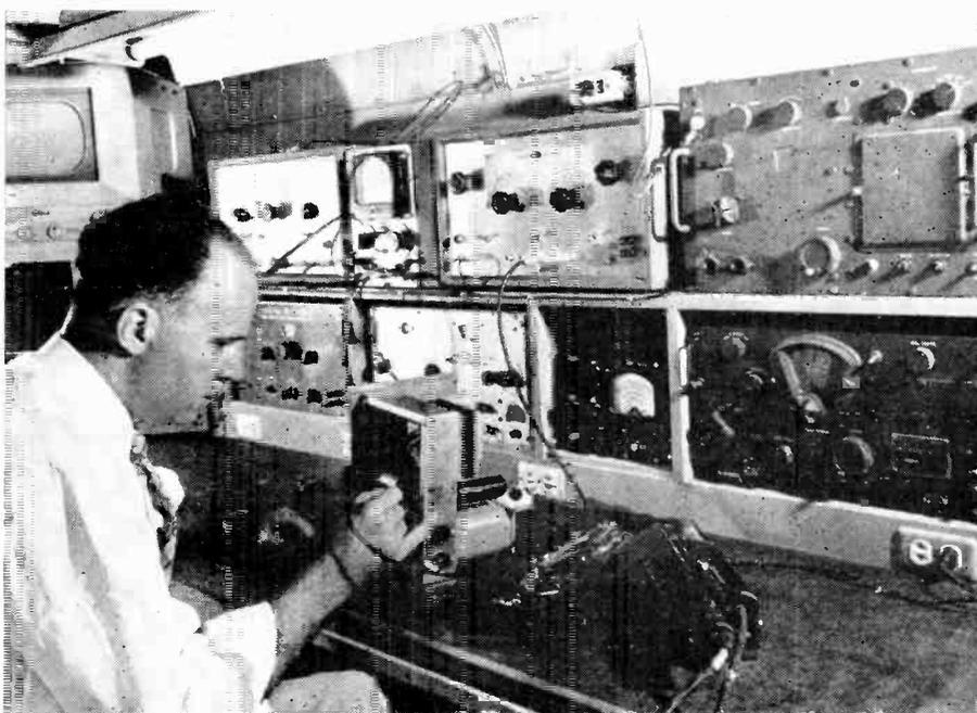
Interior of the rolling service shop. Note TV screen at upper left, 110 v. AC outlets. Power is provided by an auxiliary generator in the truck.
