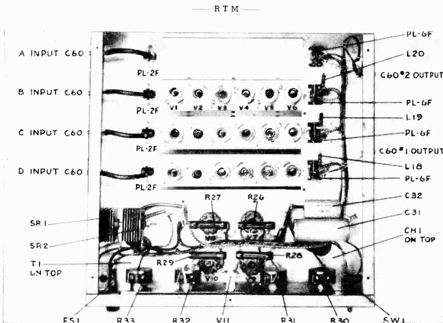
Fig. 4. Under-chassis view of the Mul-TV master control section, with channel amplifier strips plugged in. Gain controls, transformers, rectifiers are at bottom.
