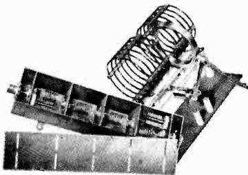
compartments, prevents inductive transfer of unwanted frequencies from section to section. RF bypass condensers in the K sections have resonant frequencies higher than 500 Mc, thus eliminating resonances within the TV bands.
