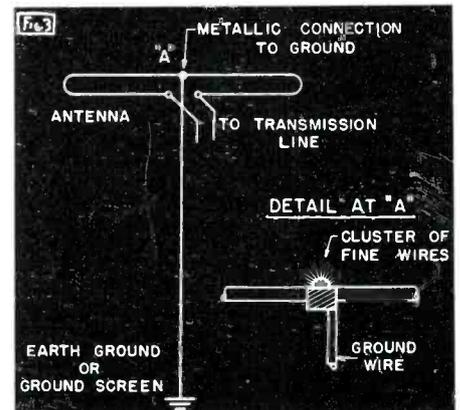
Fig. 3. Method of draining off static charges on metallic antenna structures, originally suggested by A. C. Kadow. Electric charges from the atmosphere may produce audible hiss in the receiver unless an easy conducting ground is provided for d-c energy. In the illustration, the rate of discharge is considerably increased by the cluster of fine wires at point "A".
