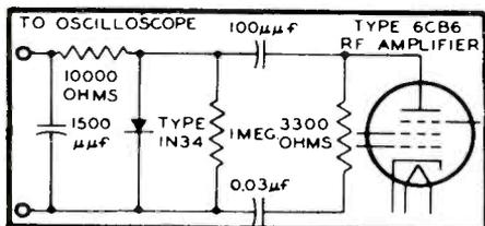
Fig. 2 Crystal-diode circuit used for coupling the oscilloscope to the r-f amplifier.
