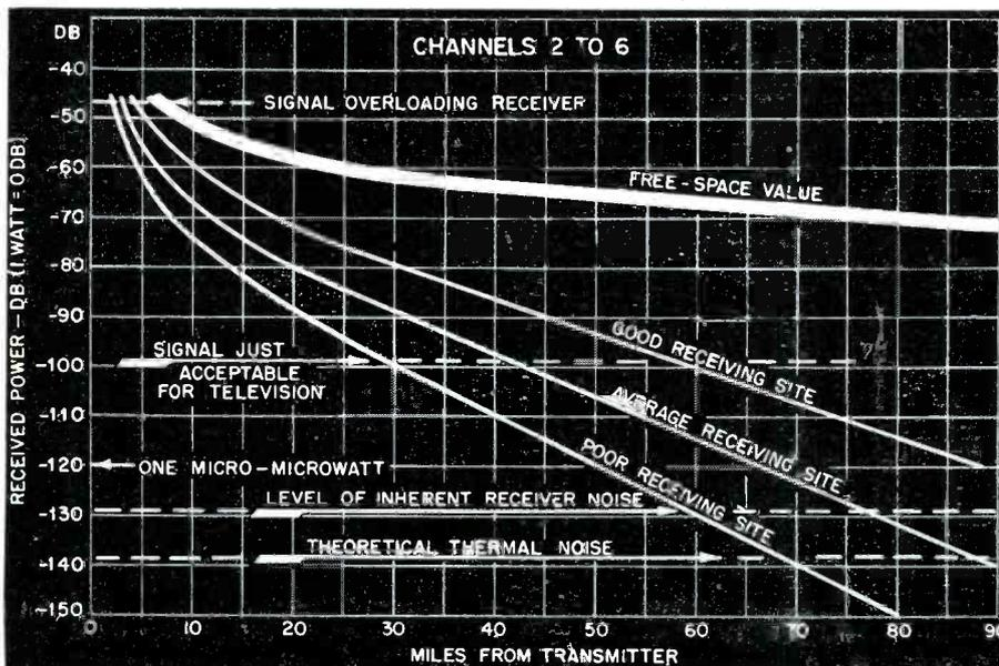
Fig. 2 (left). Relation between signal power received on half-wave dipole and distance from transmitter to receiver site, for channels 2 to 6. The theoretical maximum signal is indicated by the curve marked "Free-Space Value". As distance from the transmitter increases, divergence of expected signal levels for different receiving sites and this theoretical signal increases. These curves are based on large number of actual measurements.
