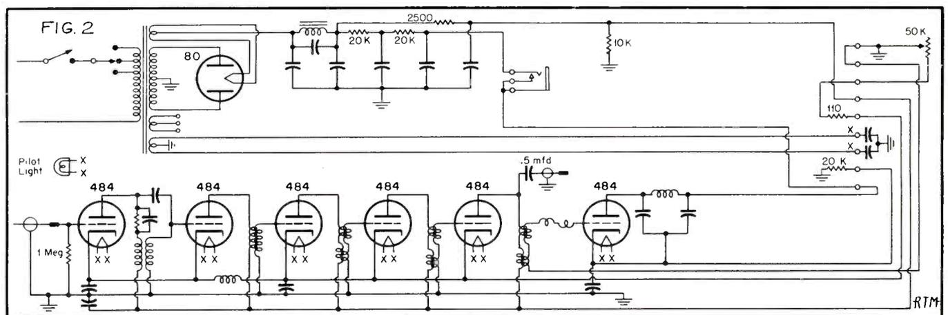
Fig. 1. Circuit diagram of the original Sparton Model 9-30 receiver used by the author for raw material in building his broad-band R.F. Amplifier. Fig. 2. Diagram of circuit as altered. Note absence of original tuning section, audio output section, and loudspeaker, and use of six amplification tubes for R.F. Signal being traced is fed into the grid of the first 484 through input probe.
