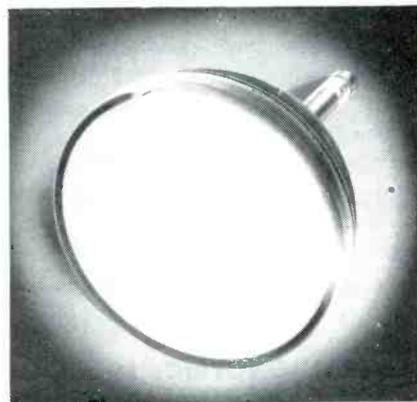
sign has been modified so that it is possible to use either a single or double magnet beam bender, allowing direct interchangeability with all type 12LP4 tubes. Allen B. DuMont Labs., Clifton, N. J.
