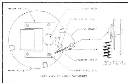
from the front of the radio cabinet, just far enough to permit installation of the booster spring. The accompanying illustration shows the position of the booster spring as viewed from the rear of the clock mechanism. One end of the spring is fastened to the cam stud, the other end to the brass front plate stud.
