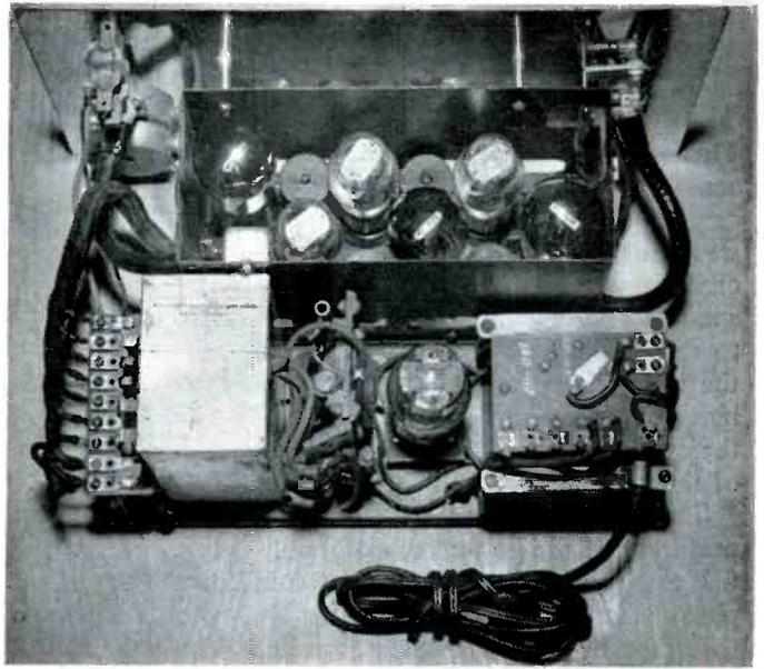
A top view of the unit. Note the .5 mfd., oil-filled condenser mounted inside the case near the filter condenser bank. The co-ax leads going from the panel outlets to the amplifier can be seen. The amplifier cover has been removed.
