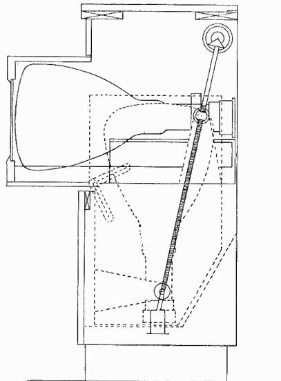
Fig. 6 Lift mechanism for 20" tube.
