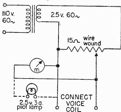
coil of the speaker being tested. Advance the wire wound resistor until the 60 cycle hum is heard in the speaker. This hum should be steady and the bulb should not flicker. Otherwise, an intermittent condition is indicated.
