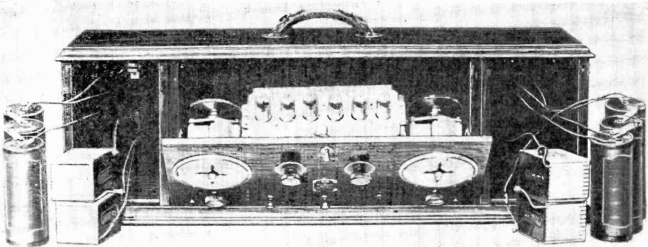
Fig. 6 A definite step forward was marked by the development of this Radiola battery powered superheterodyne.
