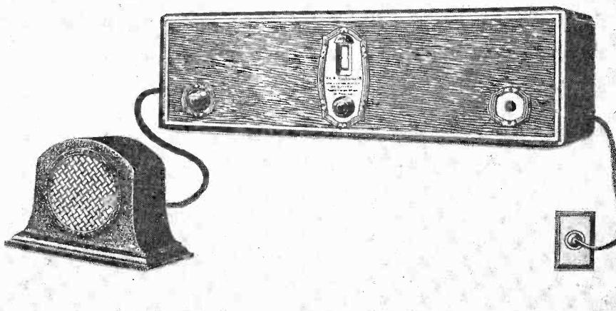
Fig. 8 One of the first "all AC" receivers, the Radiola 18.
