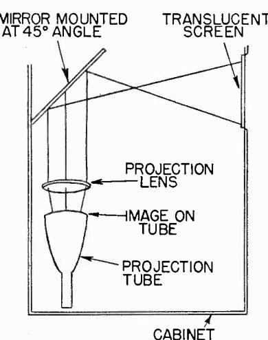
Fig. 10 Projection system using refractive lens.
