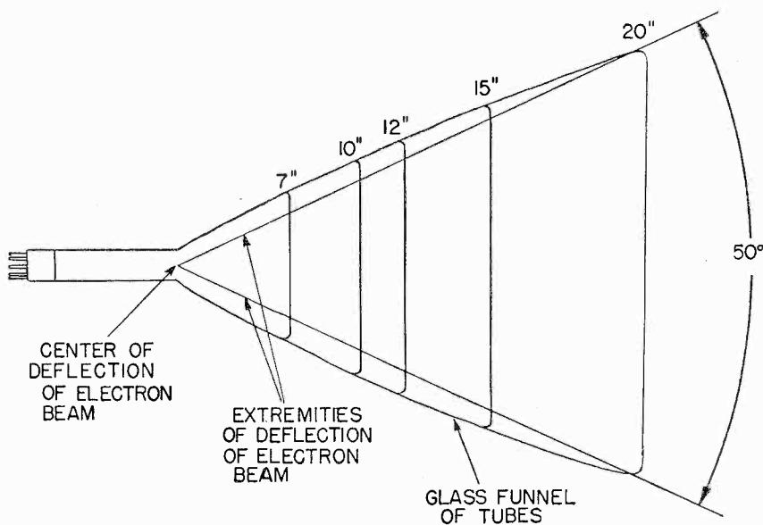
Fig. 9 Relative sizes of magnetic type television tubes.
