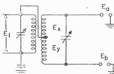
Fig. 4 Showing how two voltages  $E_a$  and  $E_b$  are produced for application to the plates of the diodes.  $E_a$  and  $E_b$  vary in magnitude as the frequency of the input changes.
