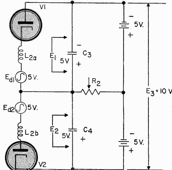
When the input ratios are equal no current flows through  $R_2$  and the output will be zero.
