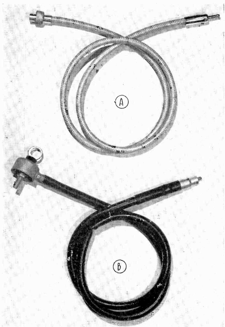
**Fig. 1 Two types of antenna lead-in cable for automobile use: A, Polyethylene insulated type; B, older type using paper loom construction and shield can fitting. Choice of lead-in cable can have an important effect on efficiency of the automobile receiver.**
