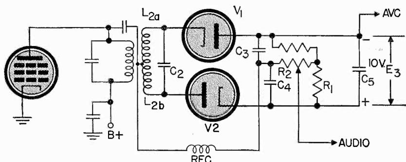
Fig. 8 The ratio discriminator. Below: Schematic diagram, Above: equivalent circuit discussed in the text.
