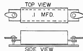
end and a lug for support. This eliminates warped and twisted wire leads and makes it easy to get good contact with test prods.
