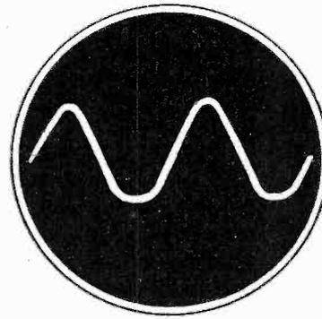
**Fig. 4 The pattern obtained when severe distortion exists. Note the flattening of the bottom of the wave form pattern.**
