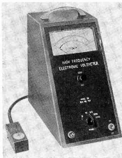
capacity of 5 micro-microfarads or more, the loading and detuning of very high frequency circuits have presented a serious problem, to which Model 32 supplies the answer.
