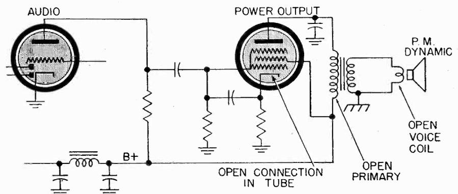
Fig. 1 When there is no sound coming from the speaker of a receiver using a permanent magnet dynamic speaker, the trouble is usually an open at one of the points indicated.
