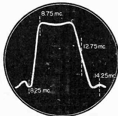
Fig. 9 The sound rejection obtained between 8.25 megacycles and 14.25 megacycles in the video intermediate frequency system of a good quality receiver.
