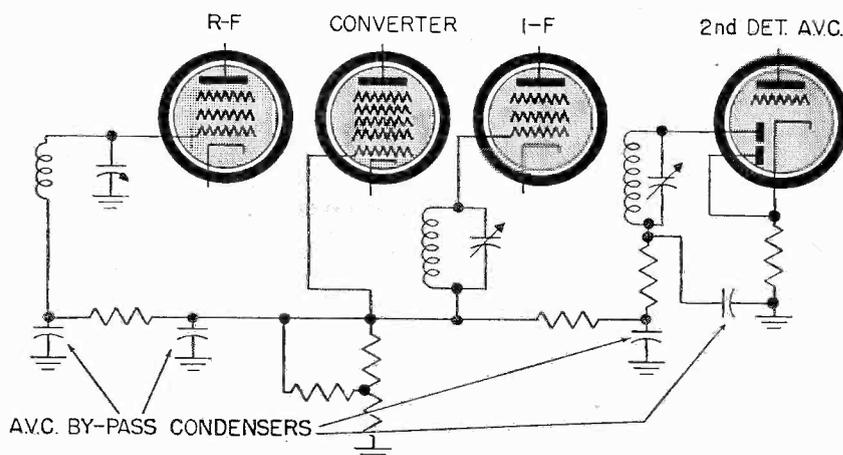
**Fig. 4** If any one of the by-pass condensers indicated above is shorted, the set will distort badly on loud stations but will sound normal on weak stations.
