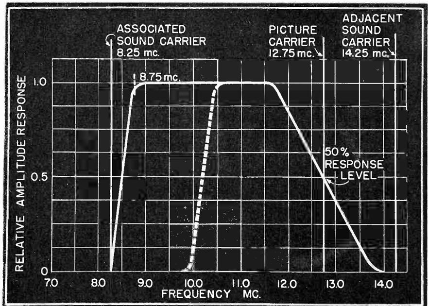
Fig. 3 The ideal picture intermediate frequency amplifier response curve.
