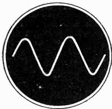
**Fig. 2 The pattern obtained on the oscillograph screen when no distortion is present in the receiver.**
