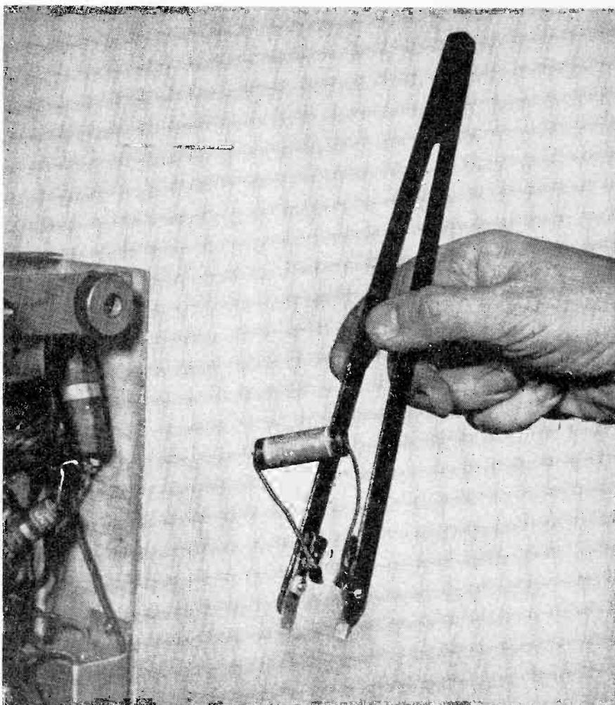
**Fig. 3** A handy gadget for use when bridging by-pass condensers to check for opens. Two battery clips are mounted at the ends of the tongs. The battery clips project past the end of the tongs. The proper size condenser is selected and connected to the two clips. A .1 ufd condenser can usually be used to check all the by-passes on a set.
