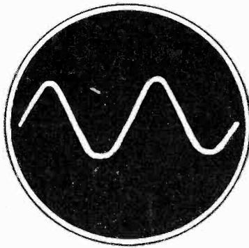
**Fig. 3 The pattern obtained when a slight amount of distortion is present in the receiver. Note the flattening of the bottom of the wave form.**
