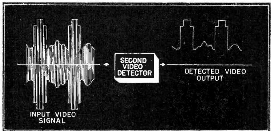
Fig. 4 The input and output signals of the second video detector.
