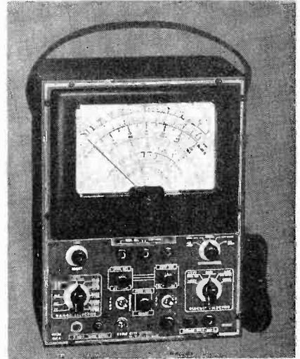
This instrument is 9 3/4" x 12 1/2" x 6" and weighs 13 lbs., complete in metal case with 4 leads.
