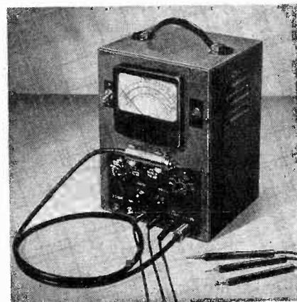
Measurement ranges of the Polymer include: DC volts, 0-1000, in six ranges; AC volts, 0-300, in five ranges. Current measurements are provided for by seven ranges, and resistance by six ranges up to 1000 megohms.
