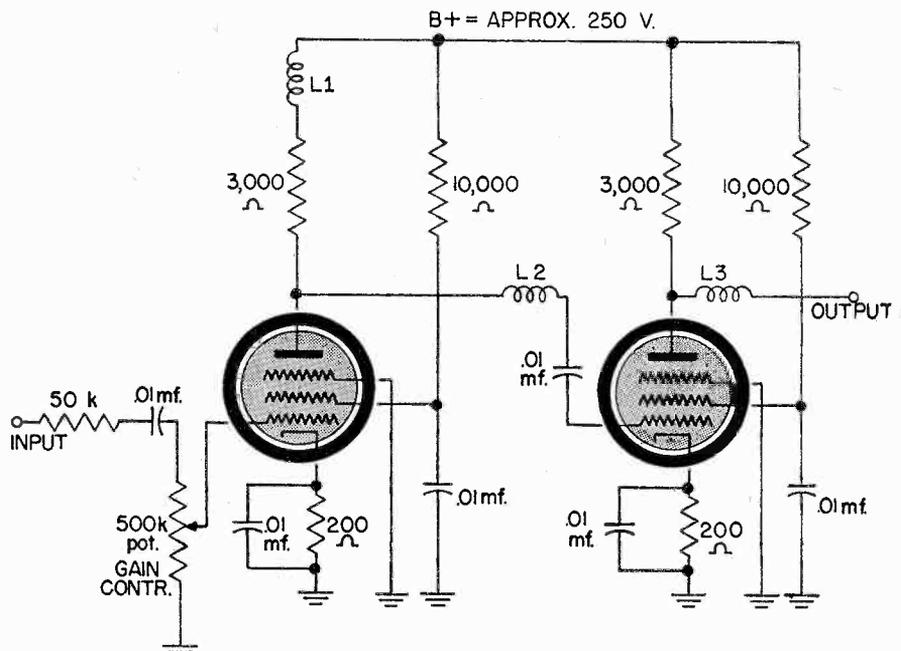
Fig. 6 The circuit diagram of a two-stage video amplifier suitable for use when checking the RF stage of a receiver for distortion.
