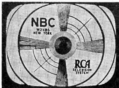
Fig. 6 A normal test pattern.
