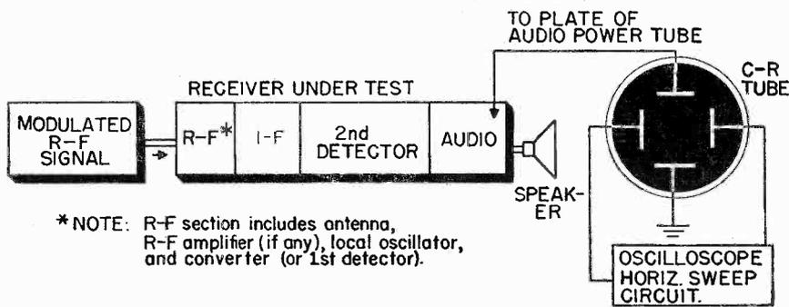
**Fig. 1 Method used to check a receiver for overloading. The RF signal generator is set at a point on the broadcast band and its output is modulated by a 400-1000 cycle audio signal.**
