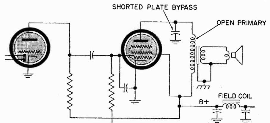
Fig. 2 In a set using a field type speaker, if no stations nor static can be heard but the speaker emits a low hum, the trouble is usually one of those indicated above.
