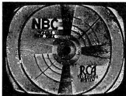
Fig. 7 A test pattern showing the effect of loss of low video frequencies.
