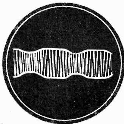
**Fig. 9** The pattern obtained with the test setup of Fig. 7 when distortion is present in the receiver.
