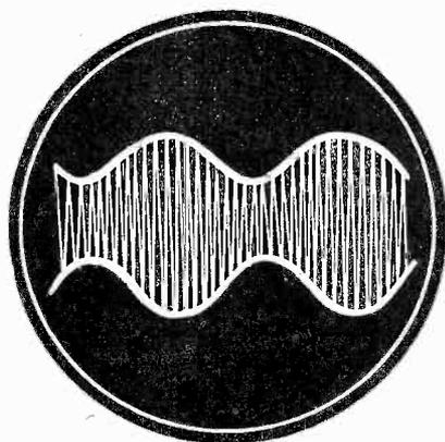
**Fig. 8** The pattern obtained with the test setup of Fig. 7 when no distortion exists.
