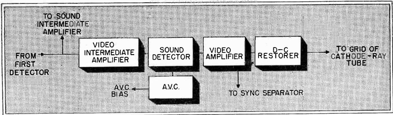
Fig. 1 A block diagram of the video channel of a television receiver.
