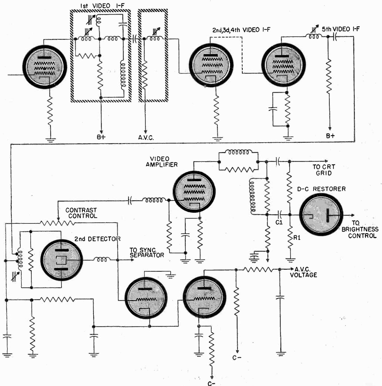
Fig. 2 A simplified schematic diagram of the video channel of a television receiver
