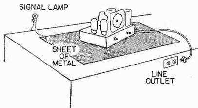
Fig. 1 A plate mounted on the workbench and grounded through a lamp acts as a signal to indicate voltage on the chassis of a set.
