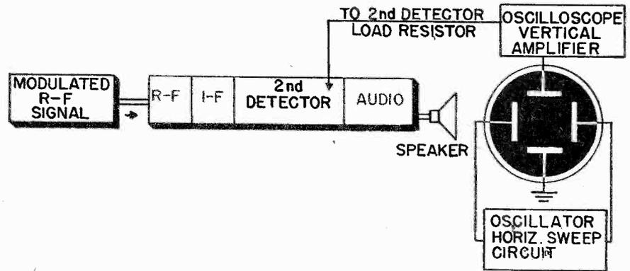
Fig. 5 Method used to check for distortion in the circuits up to and including the second detector.
