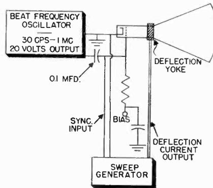
Fig. 10 Method used in checking the linearity and amplitude of the scanning circuits.
