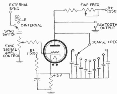
**Fig. 4** Thyatron sweep generator circuit as used in the DuMont 208B oscillograph.
