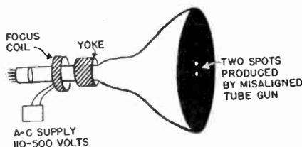
Fig. 4 Alignment of electron gun in magnetically focused tube using the 60-cycle method.
