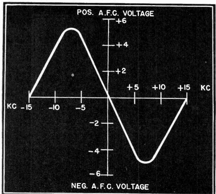
Fig. 4 Typical discriminator output curve.
