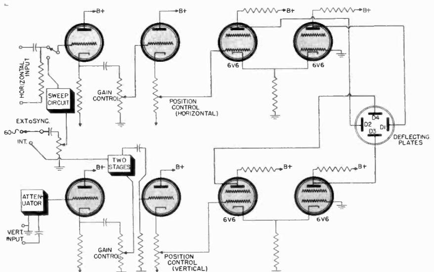
Fig. 7 Simplified schematic diagram of the horizontal and vertical amplifiers used in the DuMont 208B.
