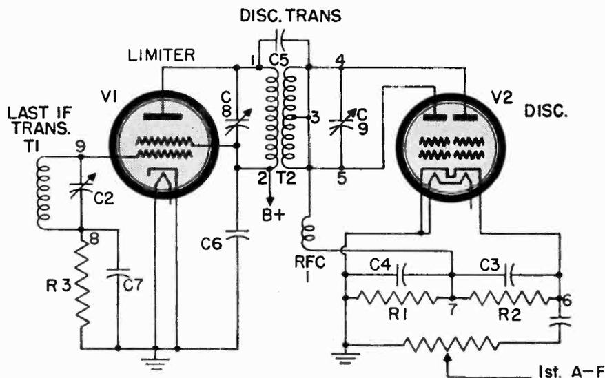
Fig. 4 Partial diagram of a typical limiter and discriminator circuit.
