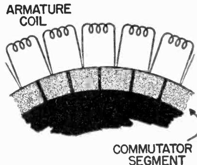
Fig. 4 Armature connections used in some types of phono motors.
