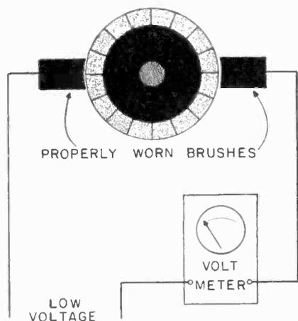
Fig. 1 Connections used for checking the brush contact of a phono motor using a battery and a voltmeter.
