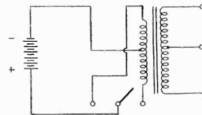
Fig. 4 Switching system used to reverse current flow in a transformer when the primary is tapped.
