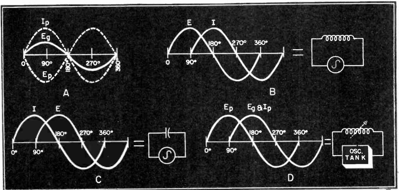
Fig. 2 The voltage and current relationships in an oscillator.
