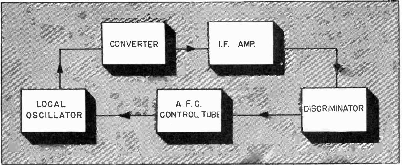
Fig. 1 Block diagram of an AFC system.
