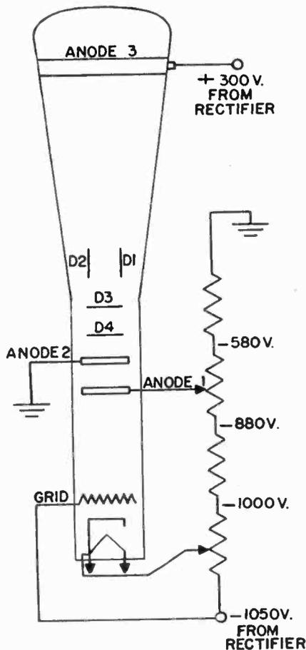
Fig. 8 Typical voltage dividing system used in cathode-ray oscillographs.
