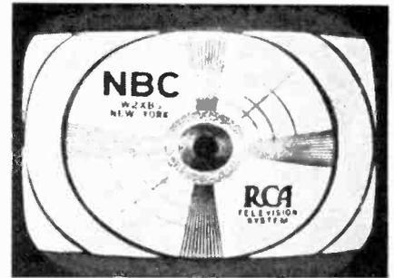
Fig. 11 A test pattern with the vertical height control incorrectly set.
