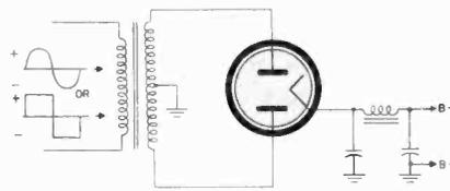
Fig. 2 A conventional plate power supply system.
