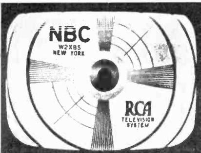
Fig. 16 The fold-over effect caused by improper peaking in the vertical scanning circuit.
