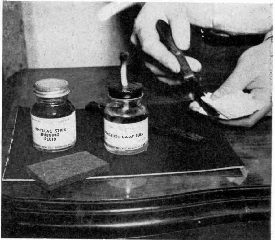
Fig. 3 Wipe the spatula carefully to remove carbon after heating it over the alcohol flames.
