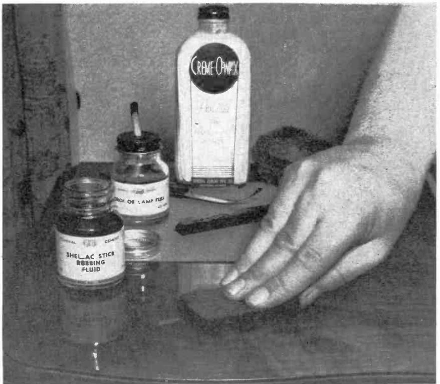
Fig. 6 After removing the excess shellac with a razor blade, smooth the surface with a felt pad soaked in rubbing oil.
