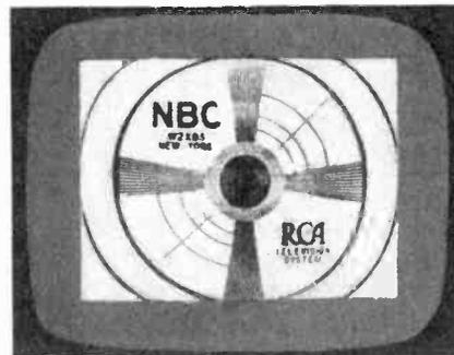
Fig. 8 A test pattern with the horizontal width and vertical height reduced to align the picture parallel to the mask.
