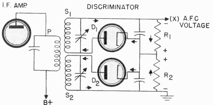
Fig. 3 Simplified diagram of a discriminator circuit.
