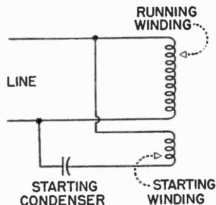
Fig. 3 Circuit used in a split-phase motor. The winding with the condenser in series is the starting winding.
