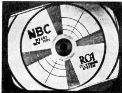
Fig. 7 An incorrectly oriented picture caused by a misaligned deflection yoke or electrostatic tube.
