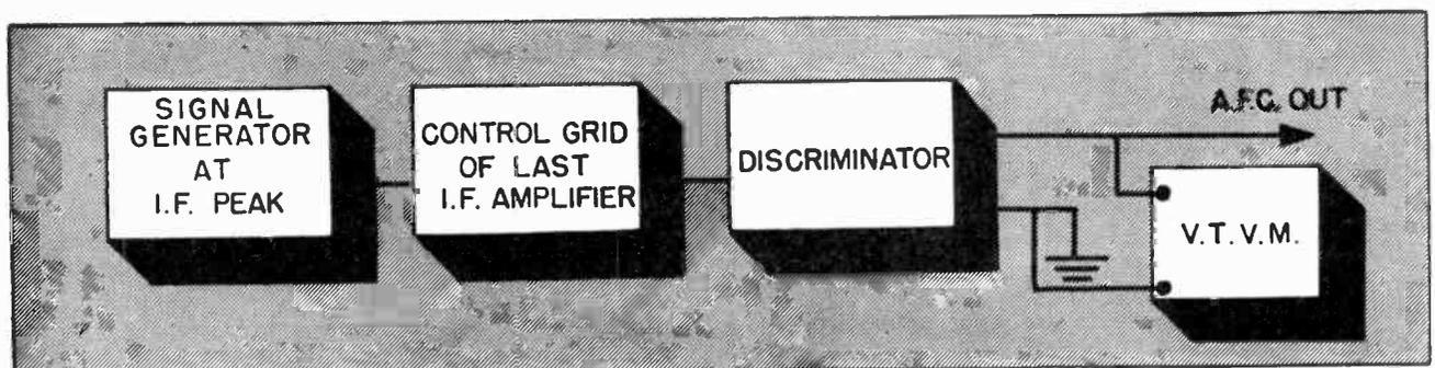
Fig. 6 Connections used for the signal generator and VTVM when adjusting the AFC circuit.
