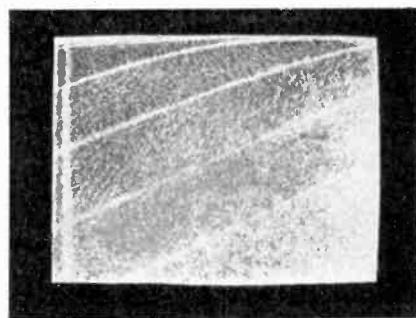
Fig. 6 A correctly oriented scanning raster. Note the angle of the retrace lines.
