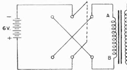
Fig. 3 Switching system used to reverse current flow in a transformer primary.
