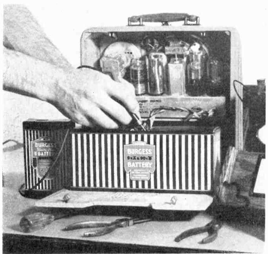
When it is possible, a battery should be given a voltage check in the set while it is in operating condition.
