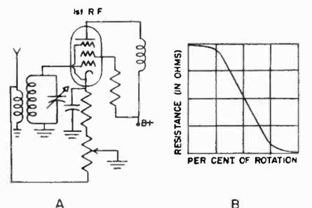
**Fig. 7** Screen voltage method of controlling the output of a receiver.
