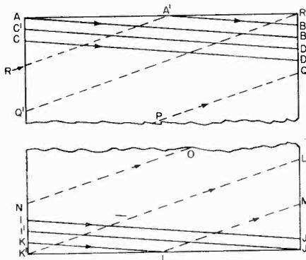
Fig. 7. Diagram of path followed by electron beam in scanning target of camera tube or screen of kinescope.
