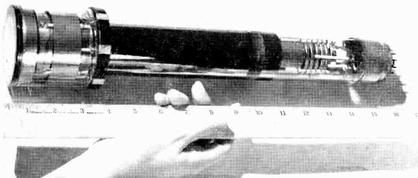
Fig. 5. The RCA Image Orthicon, a super-sensitive camera tube of recent development.
