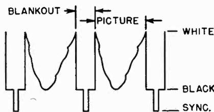
Fig. 9. Waveform of basic video signal.
