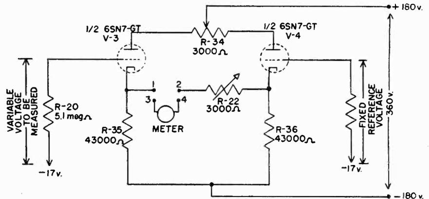
Fig. 6 Simplified diagram of the DC metering circuits.
