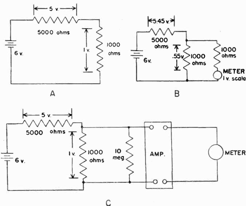
Fig. 1 Simplified diagrams illustrating the effect on circuit conditions caused by connecting a voltmeter to the circuit. 'A' shows circuit conditions before the instrument is introduced. 'B' shows circuit conditions when an ordinary voltmeter is connected to the circuit. 'C' shows how the electronic voltmeter does not disturb the circuit when connected.
