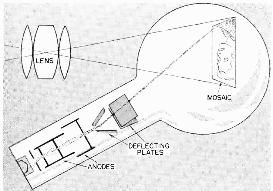
Fig. 2. Diagram of camera tube in television camera.
