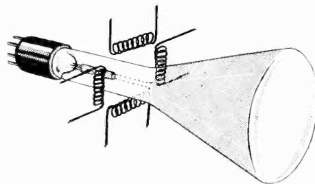
Fig. 8. Cathode ray tube showing position of deflecting coils.
