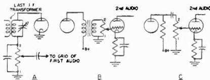
**Fig. 3** Three methods of controlling the output of a receiver in the audio section.
