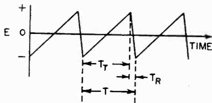
Fig. 6. Saw-tooth scanning voltage, as applied to deflection plates of electrostatic tube.
