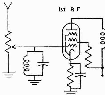
**Fig. 5** Antenna shunt method of controlling the output of a receiver.
