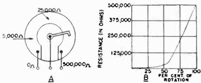
**Fig. 2** A non-linear taper control showing the relation between rotation and resistance change.
