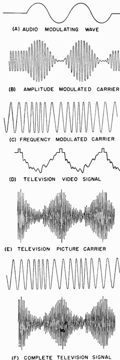
Fig. 10. Sound- and picture-modulated carrier signals.
