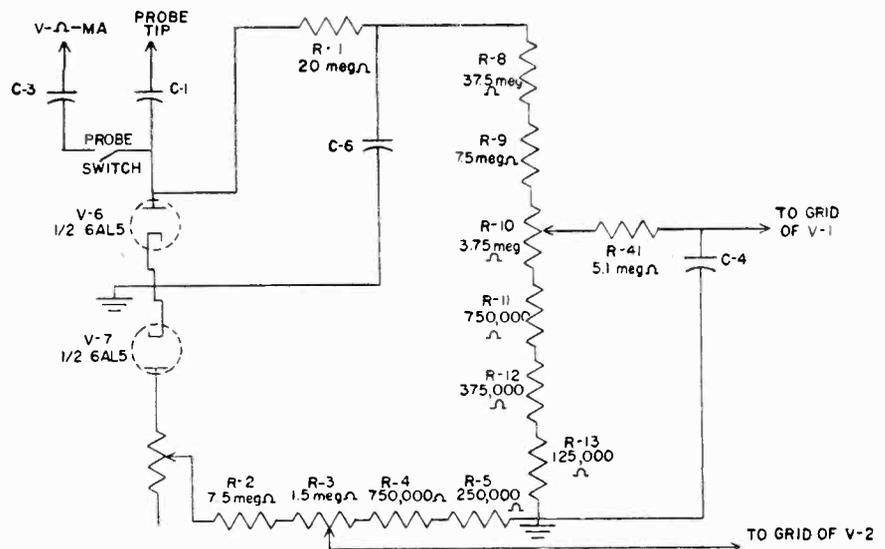
Fig. 7 Simplified diagram of the AC voltmeter input circuit.
