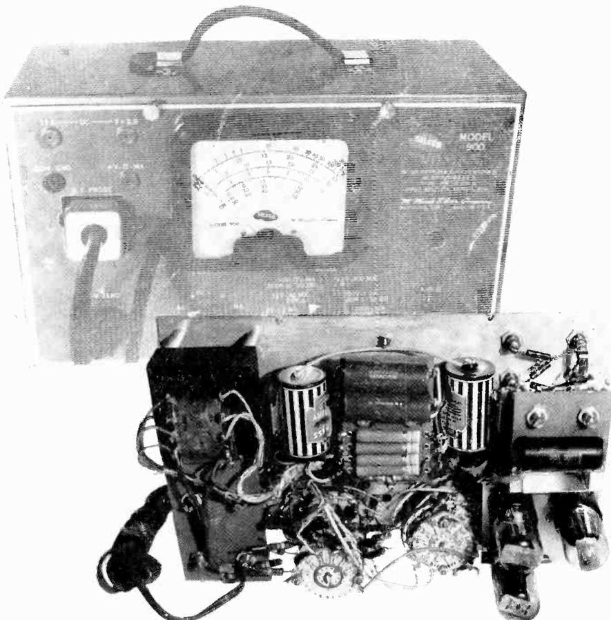
Fig. 2 The Silver Model 900 VOMAX which is used in this article as an example of the electronic volt-ohmmeter.
