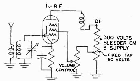
**Fig. 6** Combination antenna shunt and C bias method of volume control.
