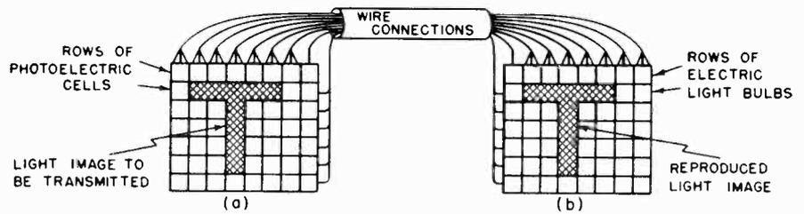
Fig. 1. Elements of the simplest television system. One similar to this is in use at Times Square, New York.
