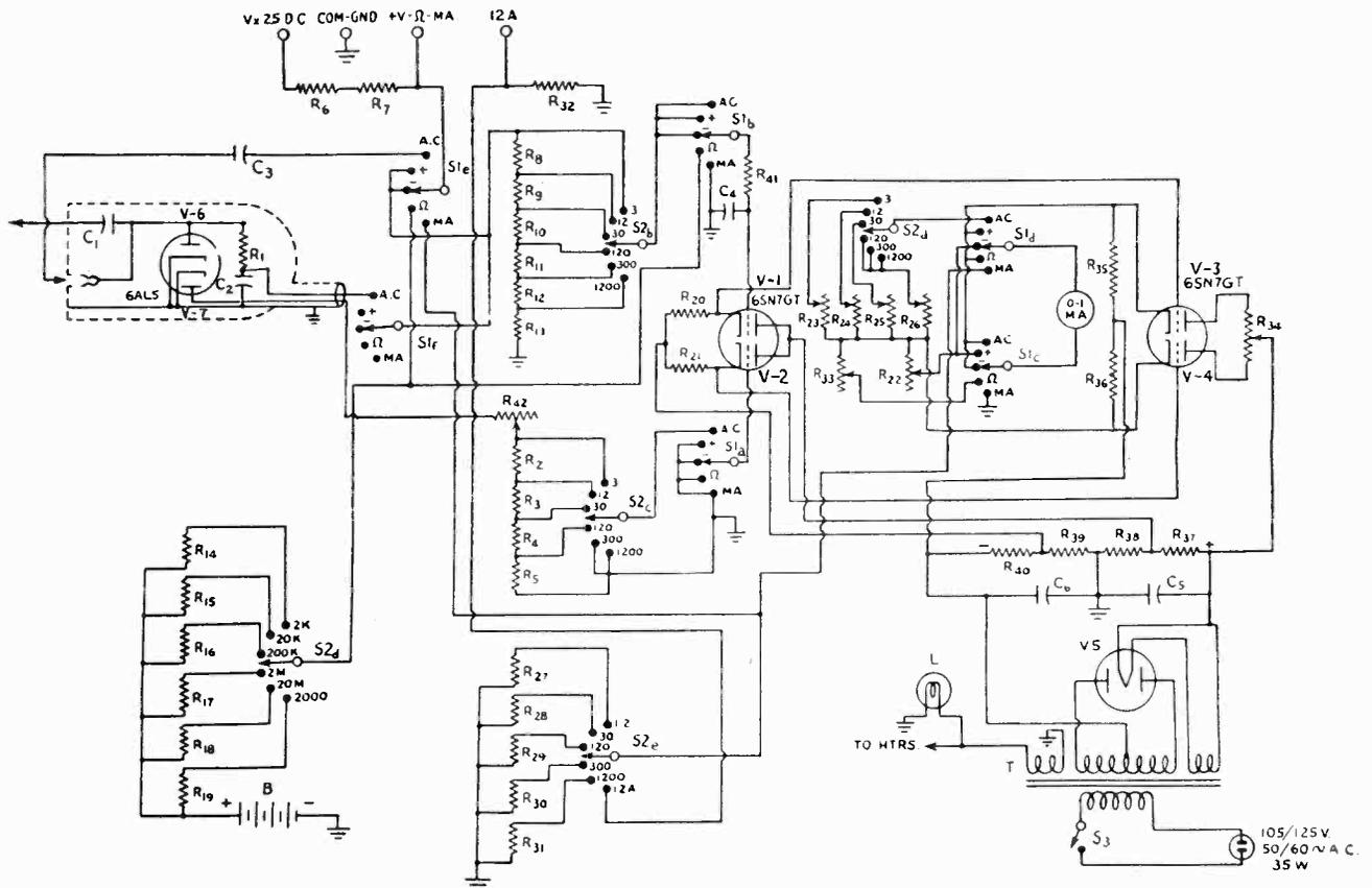
Fig. 5 The circuit used in the VOMAX.
