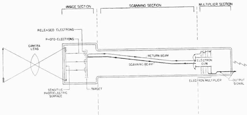
Fig. 4. Diagram of Image Orthicon of Fig. 5, showing functioning of electron beam within the tube. Electron multiplier greatly increases amplitude of output signal.
