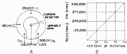
**Fig. 1** Linear taper control showing the relation between rotation and change in resistance.
