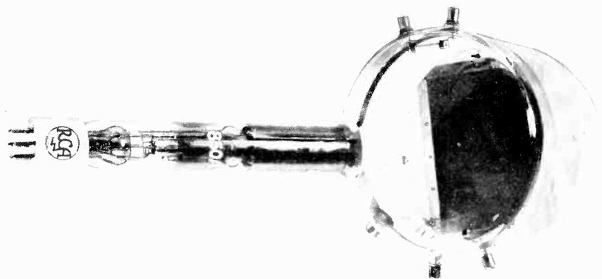
Fig. 3. An RCA Iconoscope (camera tube) of the large studio or professional type.
