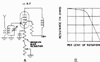
**Fig. 4** Variable C bias method of controlling the output of a receiver.
