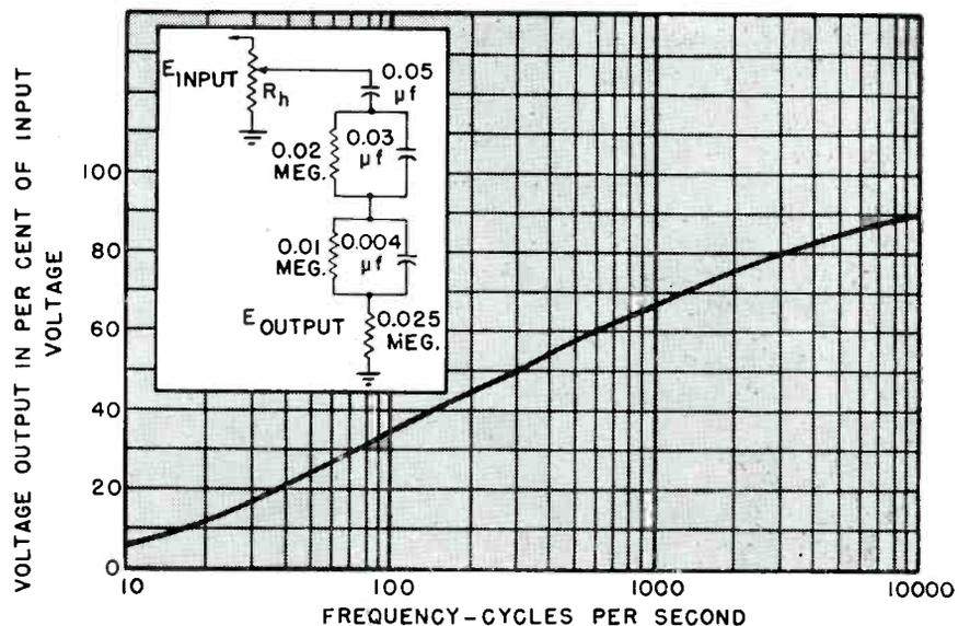
Fig. 4. Curve showing horizontal deflection voltage available from circuit of Fig. 3 as a function of frequency.
