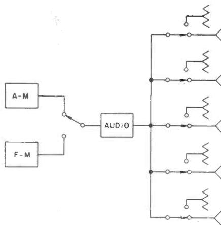
Fig. 1 The simplest system—A-M and F-M radio, with five speakers.
