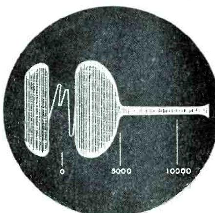
Fig. 8. Showing relatively poor response from receiver with very sharply peaked I-F stages. Attenuation of high frequencies extremely noticeable.
