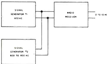
Fig. 2. Method of mixing outputs of two R-F signal generators to obtain modulated signal furnishing audio frequencies from 0 to 10,000 cps.
