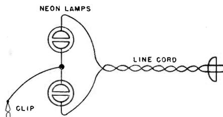
Ground detector composed of two 2-watt neon lamps, a line cord, and a test lead with a clip.
