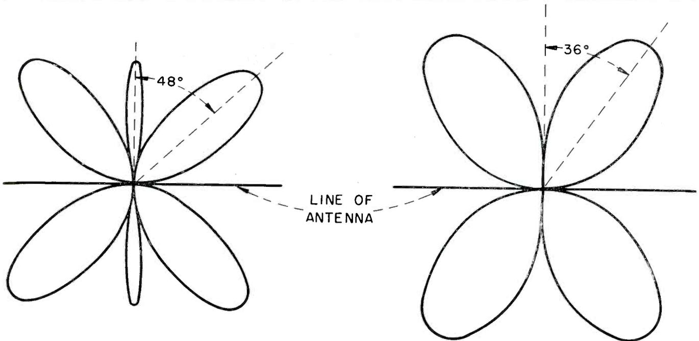
Fig. 4. Directional sensitivity lobes for a 3/2-wavelength antenna (left) and for full-wave antenna (right).
