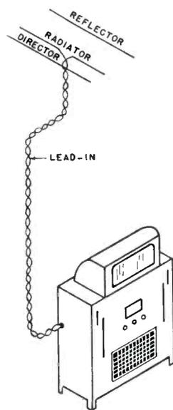
Fig. 1. The elements of an antenna system suitable for F-M and Television, with director and reflector, together with transmission line to set.
