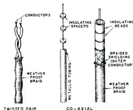
Fig. 3. 73-ohm transmission line — twisted pair, and two types of co-axial cable.
