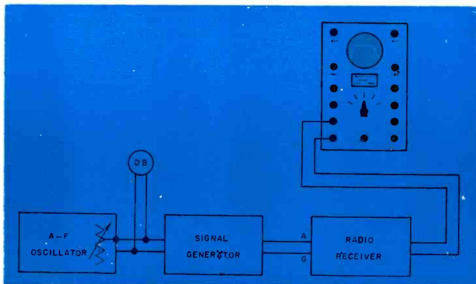
Fig. 1. General method of making overall frequency response measurements, using audio-frequency oscillator, R-F signal generator, and an oscillograph for continuously indicating the output signal.
