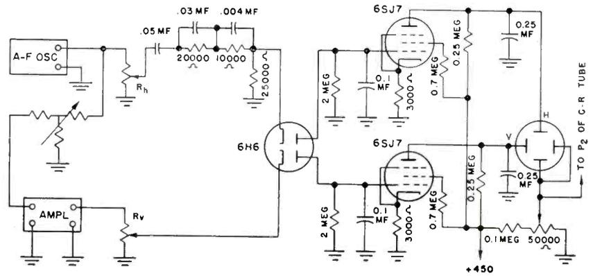
Fig. 3. Schematic of circuit for making curves of audio frequency response. Horizontal deflection is approximately proportional to frequency on a logarithmic scale, and vertical deflection is proportional to voltage output from the amplifier. (Courtesy RCA, from Application Note 76.)
