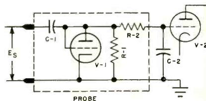
Fig. 2. Simplified input circuit of General Radio 726A vacuum tube voltmeter.
