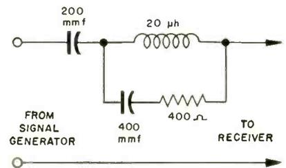
Fig. 8. Circuit of standard dummy antenna.
