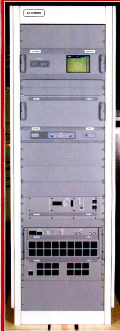
Pictured is a Mini-HD transmitter from Harris Corp. Part of the company's low-power HD Radio FM transmitter line, the Mini-HD is designed for FM radio stations that use space combining to implement HD Radio. Applications include separate antennas, interleaved antennas, dual-port antennas, and FM combiner port injected feeds. Its four models range from 60 watts to 600 watts.
