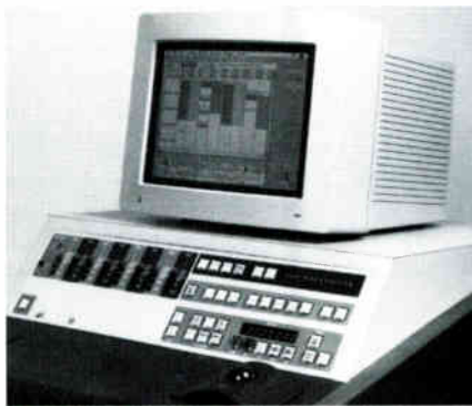
Pacific Recorders' ADX system, an eight-track digital audio workstation.
