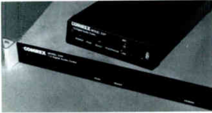
Comrex Corp.'s Digital Audio Coders, DXP (portable) and DXR (rack-mounted).
