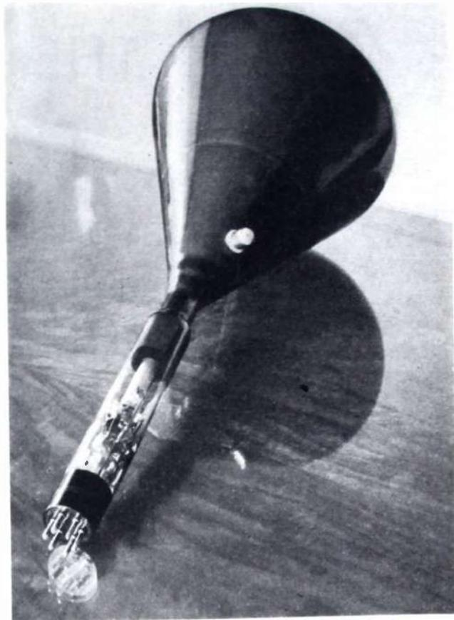
Colloidal graphite deposits serve as a focusing anode in the 903 cathode-ray tube, a high-vacuum electromagnetic type.
