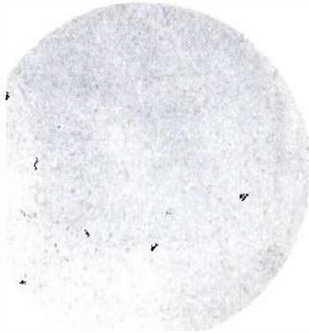
Flat strip of Svea metal for radio: Surface with no polishing or etching (100X unretouched). Note uniformity with freedom from slag, impurities and gas bubbles.
