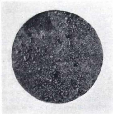
Copper, after 150-hour bath in mercury at room temperature (60X).
