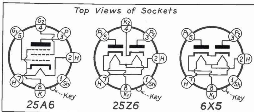
The third new metal tube is the type 6X5, a narrow space, high-vacuum rectifier designed primarily for automobile receiver use.
