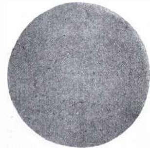
Svea metal, after 150-hour bath in mercury at room temperature (60X).
