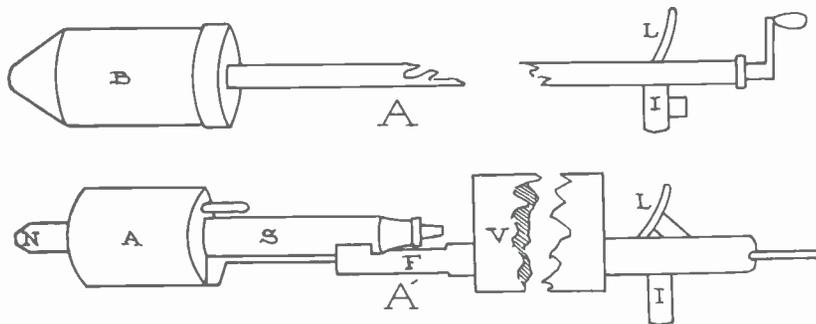
Fig. 3. (A') By pulling the lever L the intake I and the nozzle N open, as the section S moves back and forth on F. The chamber A contains the binder material, while V is a vacuum space. (A) By opening the valve by means of L and rotating the crank slowly, the fluorescent powders in B are forced out by the pressure of  $\frac{1}{2}$  to  $\frac{3}{4}$  atmospheres. Overall length of guns, 12 inches. (Courtesy of Pfaltz & Bauer.)
