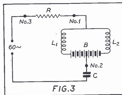
Circuit for measurement of inductance of chokes.
