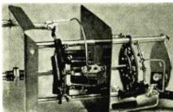
Fig. 8. Showing construction of the switching sections and manner of circuit connections.
