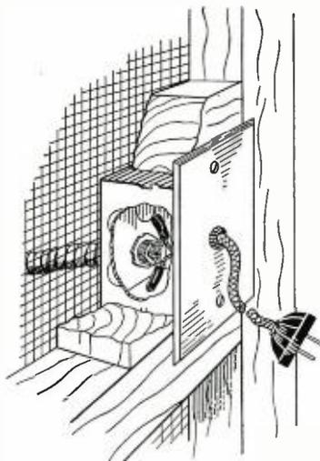
Fig. 2. Method of connecting Tobe Filterette to Diathermy screen.
