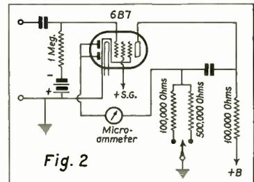
Schematic diagram of the vacuum-tube voltmeter.
