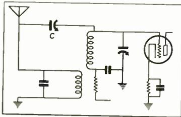
Fig. 3. Circuit of antenna coupling system.
