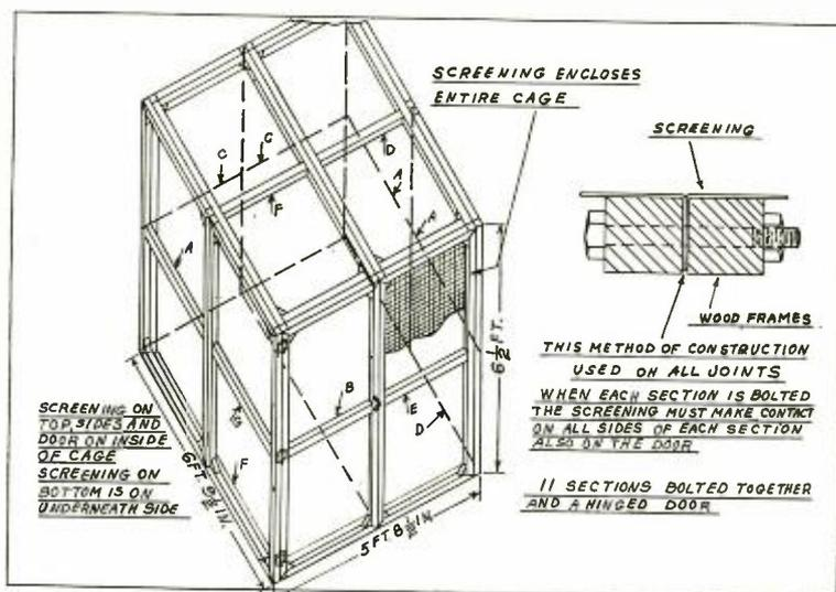
Fig. 1. Assembly drawing showing construction of Diathermy screen.
