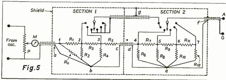
Detailed circuit of attenuator with variable input to the meter.
