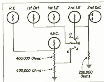
Fig. 7. The avc system in an all-wave receiver, with provisions for controlling the avc functions.
