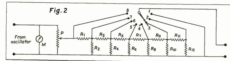
Attenuator with fixed input to the voltage-indicating device, M.
