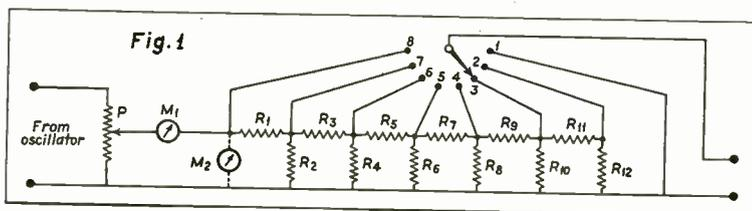
Circuit of attenuator having variable input to the indicating device. A current-measuring device, M1, may be used, or a voltage-measuring device, M2.
