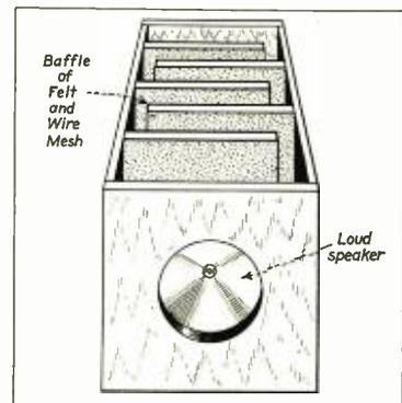
Fig. 9. Speaker with acoustic labyrinth composed of felt pads.
