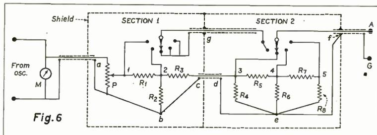
Detailed circuit of attenuator with fixed input to the meter but with the potentiometer remaining in the input leg.
