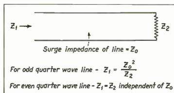
Fig. 1. Functional diagram of quarter-wave line.
