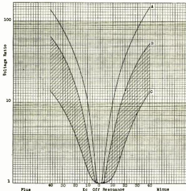
Comparative curves of one i-f stage at 456 kc; using 78 tube with 250 v. plate, 100 v. screen, 3 v. grid. Curve A: Iron-core transformer (1.5 mh at 1,000 cycles, in shield); gain, 263. Curve B: Good air-core transformer, gain, 172. Curve C: Poor air-core transformer, gain, 151.
