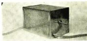
Fig. 9. The complete attenuator, with shielded input and output leads.
