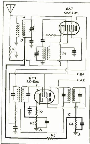
Fig. 8. Circuit, for small receivers, for the purpose of preventing overload.
