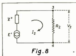
Left: The simple circuit of 7-B having added a resistance  $R_2$  between terminals 3 and 4.
