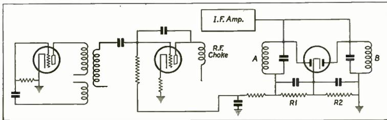
Fig. 5. A unique circuit of the self-seeking type that provides automatic tuning correction.
