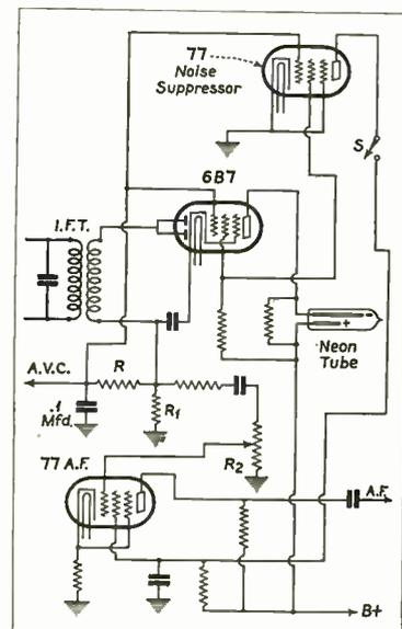
Fig. 4. Circuit of combination tuning indicator and squelch system.
