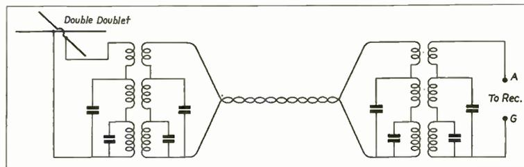
Fig. 2. Circuit of high-efficiency all-wave antenna system.
