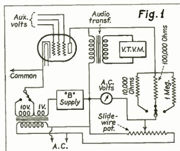
Schematic diagram of the plate-impedance bridge.
