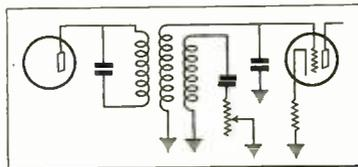
Fig. 6. Circuit of i-f amplifier having variable bandwidth.
