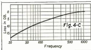
such as microphones and record pickups and reproducing loudspeakers have not been perfected to as great an extent as the audio amplifiers associated with them. The cause of this is apparent when one considers the many mechanical features which enter into both pickup and reproducer operation. Compensation for the defects in these sound source pickups and reproducers is made possible through the use of equalizer networks.
