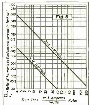
Harmonic content of tank coil current for circuit of Fig. 3.
