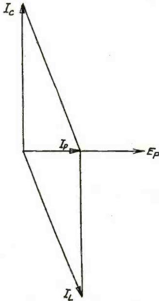
Fig. 4. Vector diagram of tank circuit with unity power factor tuning.
