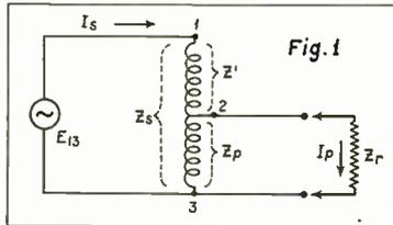
**AUTO-TRANSFORMER WITH GENERATOR AND LOAD CIRCUIT.**
