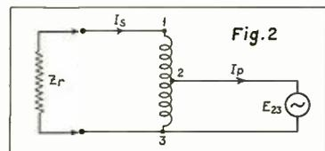
**SAME AS FIG. 1, WITH LOAD AND GENERATOR INTERCHANGED.**
