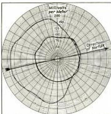
Fig. 4. Field patterns of WMC. Smaller circle is 0.5 kw unreflected. Larger circle is 1.0 kw with reflector operating.
