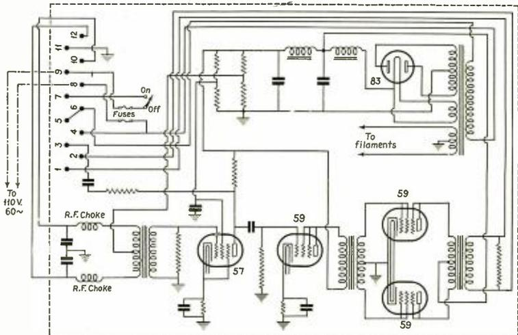
Fig. 3. Circuit of the speech amplifier and Class B modulator, with its individual power-supply unit. The three, type 59 tubes are connected to function as triodes.
