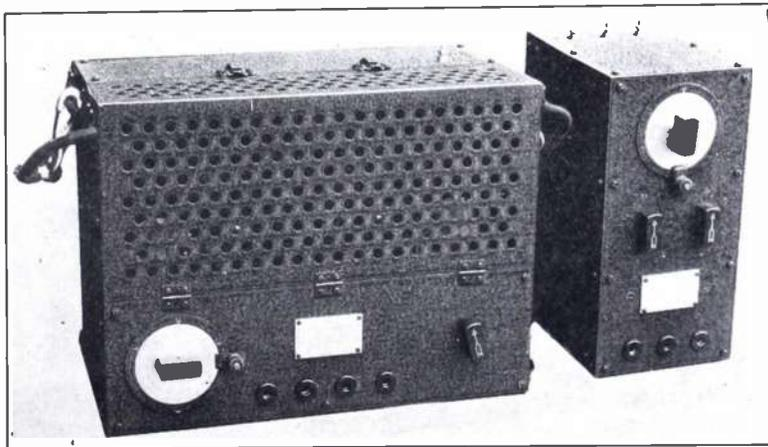
The transmitter and control box of the 100-watt airplane installation.
