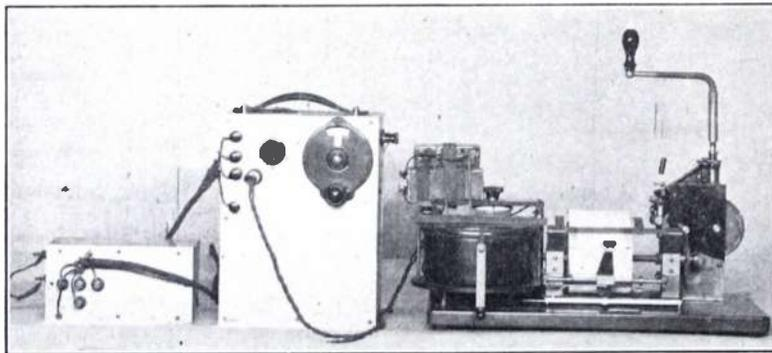
View of the combination receiver-oscillator and mechanically driven tape recorder employed for obtaining altitude readings. The records indicate the altitude of the plane from the surface of the earth rather than the sea level.
