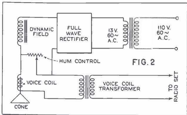
Arrangement employed for electrically counteracting dynamic speaker hum, with the aid of a variable resistance.
