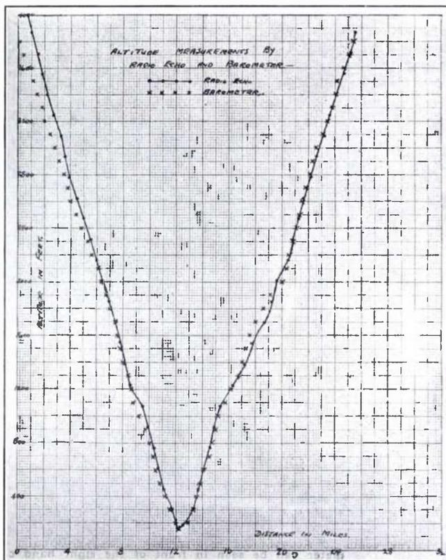
Representative set of altitude readings taken in an airplane equipped with a barometric altimeter and the "radio altimeter" described in this article. Note that the readings differ somewhat at high altitudes.
