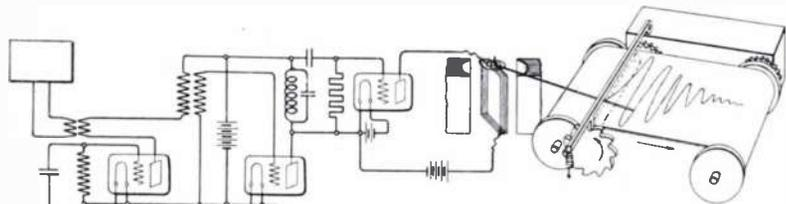
Schematic diagram of the "radio altimeter," which includes a receiver and an oscillator. The variations in the plate current of the last tube operates the galvanometer recorder.
