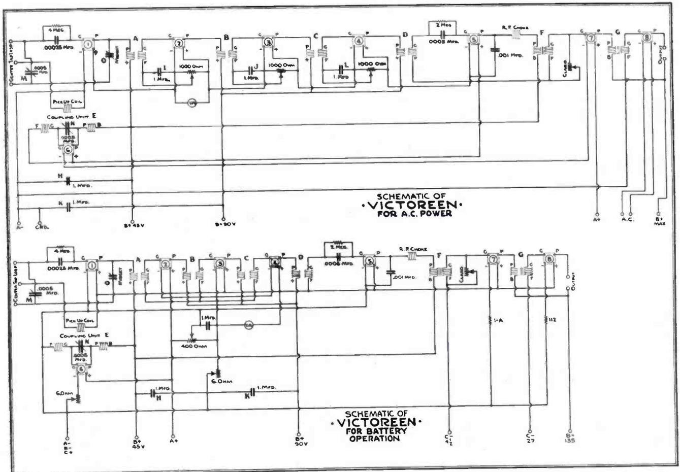
Circuit diagram of the Victoreen wired for operation from an ABC Eliminator, and the standard circuit for battery power
