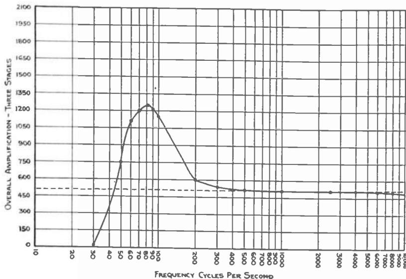
Fig. 6. The frequency characteristic curve of a three stage tuned double impedance amplifier. This will illustrate the rising characteristics of the amplifier at low frequencies
