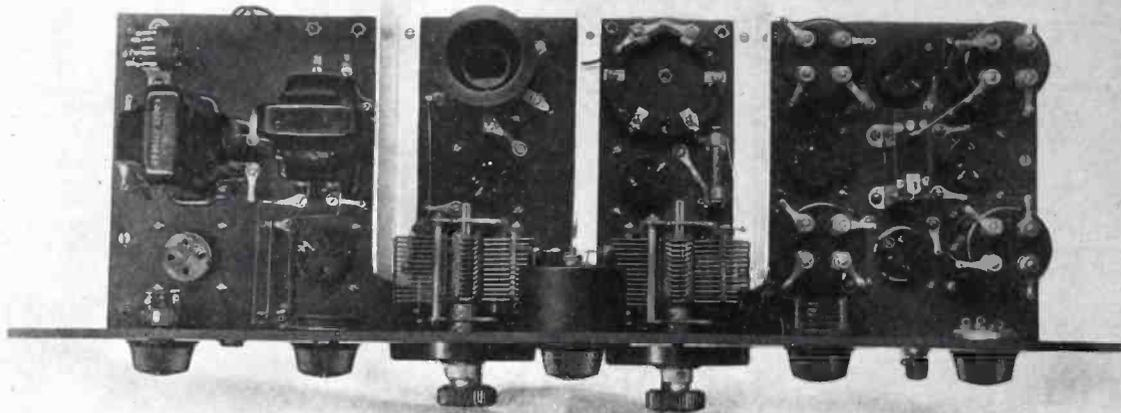
Bird's eye view of the Portable Super, completely wired and ready for installation in its carrying case. Practically every available inch of space is occupied by an efficient and compact grouping of apparatus
