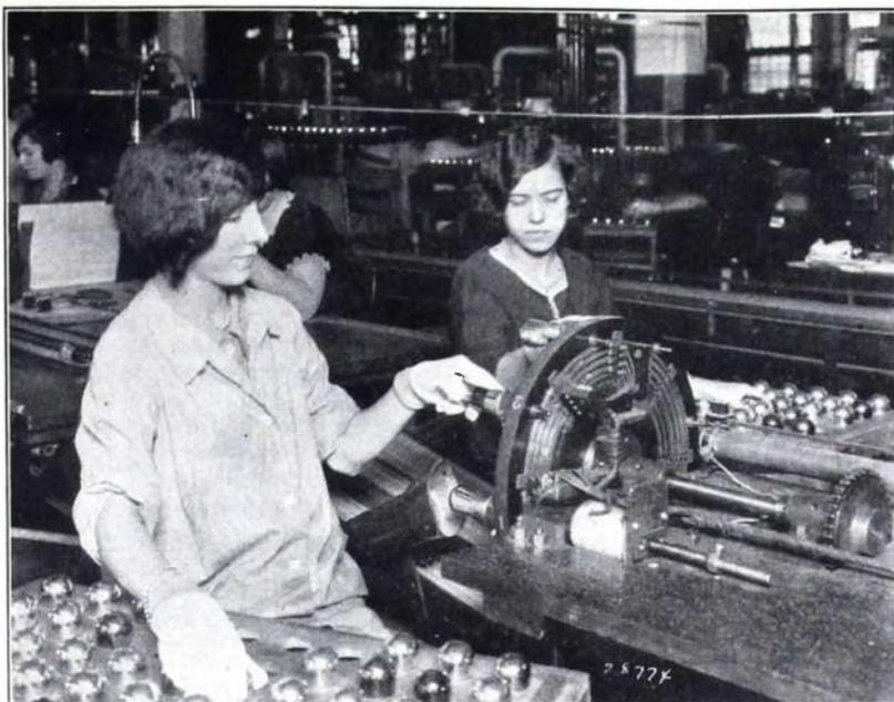
Here is a view of the high speed tube tester, an almost human machine which has a capacity of 30,000 tubes a day
