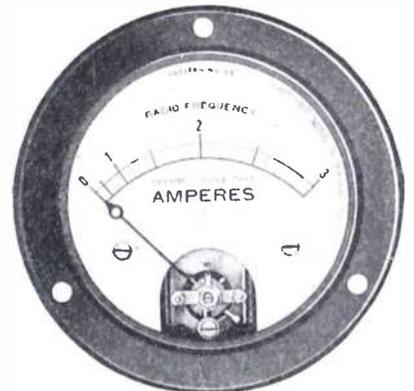
Pattern No. 135—Movement parts are all silvered and the scale is silver etched with black characters. The case diameter is two inches and can be furnished in any desired finish, standard being black enamel. It is equipped with zero adjuster, as are all Jewell moving coil instruments.
