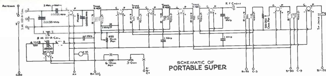
Circuit diagram of the Portable super-heterodyne. Extreme flexibility in the choice of tubes and A power supply is afforded by the fixed resistance and short-circuiting switch. A jack is provided for an external speaker
