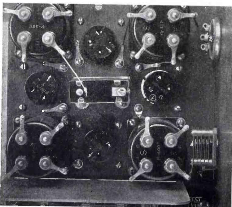
Details of the mounting and connections of the intermediate amplifier. Very short leads are used for all high potential wiring
