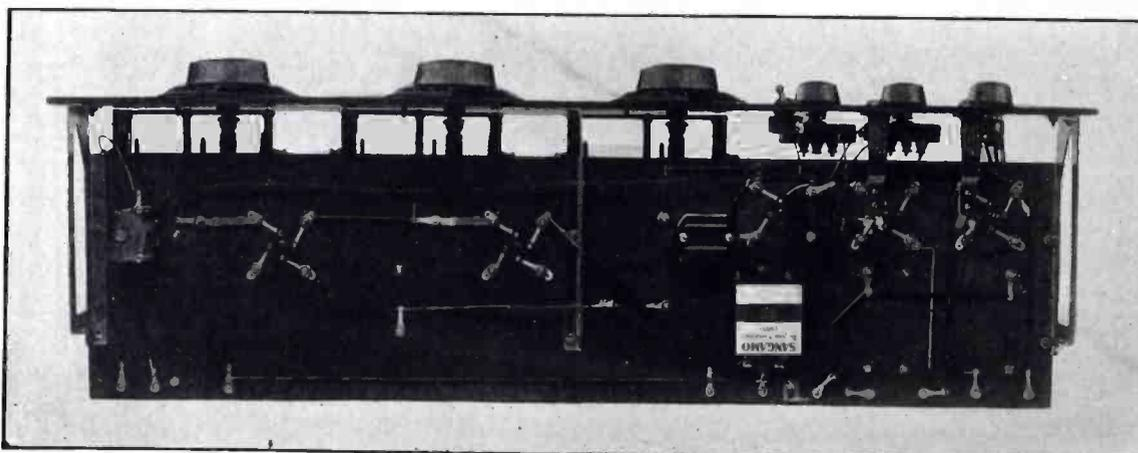
Underneath the sub-panel of the A. C. operated T.R.F. set. Note the fixed resistances, connected to the filament posts of the R.F. sockets, and which are used to provide a negative bias on the R.F. tubes
