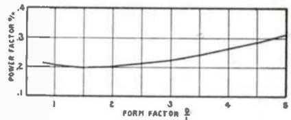
Fig. 3. Showing the desirability of keeping the form factor about 1 to 2.5
