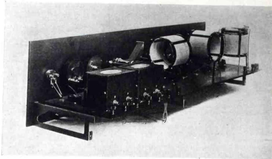
Rear view of the A. C. Aerodyne. The switch at the extreme left end of the panel is in the grid return lead of the detector, and changes this connection from negative to positive, according to the detector used.
