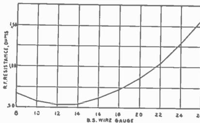
Fig. 2 A curve showing the optimum size of wire for least resistance
