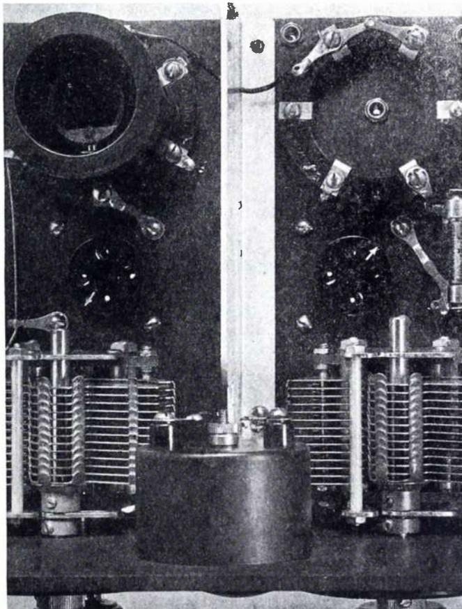
Details of the antenna and oscillator coil mountings, and the interstage shielding. The center shield is cut away slightly to accommodate the voltmeter
