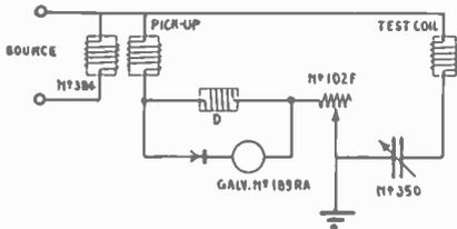
Fig. 1. Circuit diagram of the apparatus used to measure resistance of S. W. Coils
