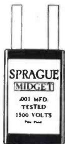
Sprague Specialties Co., Quincy, Mass., are in production on a new line of Midget condensers. Each condenser is tested at 1500 volts and is safe for continuous operation at 1000 volts. D. C. capacity is maintained constant by a special waterproofing process of triple impregnation. An asphalt and paraffin casing prevents short circuiting of leads. They are made from .0007 mfd. to 1. mfd.
