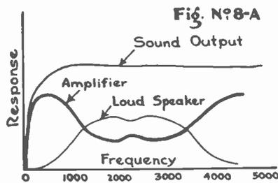
How the amplifier should be designed to compensate for the short comings of the long horn type of speaker
