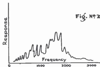
A reduction of the resonance peak by the development of the "gooseneck" speaker
