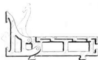
Bruno Radio Corp., Long Is. Cy., N. Y. is in production on a new adjustable bracket. The adjustable feature allows the front panel to be sloped at any angle desired. The material used is die cast aluminum.
