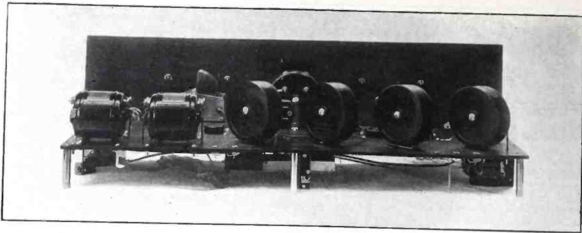
Rear view of the revised Victoreen. The oscillator coupler is mounted in the exact center. All of the bypass condensers are fastened under the sub-panel, and are grounded to the brackets, which are in turn grounded to the minus A.
