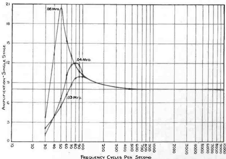
Fig. 5. The plotted curves of three stages of tuned double impedance amplification using different values of coupling capacities
