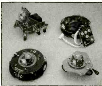
**602A "Blinky" Pathfinder Robot** Follows path made with a marker pen or tape. Red/green LEDs react to steering changes, adding fun and interest. 28 page Book. Infrared emitter/detectors.
