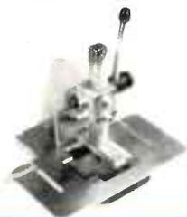
The Panavise PV505 1/4 ton manual IDC bench assembly press is a rugged, practical installation tool designed for low volume, mass termination of various IDC connectors on flat ribbon cable.
