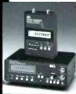
Universal Handi-Counter™ Model 3000, \$375. and Bench Model 8030, \$579. Both offer frequency, period, ratio and time interval.
