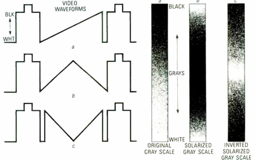
**FIG. 7—SOLARIZATION FOLDS THE SIGNAL back on itself so that white remains white, gray becomes black, and black becomes white, or vice versa. The original signal is shown in a. The solarized signal is shown in b. An inverted solarized signal is shown in c. The original waveform for each condition is shown in d.**
