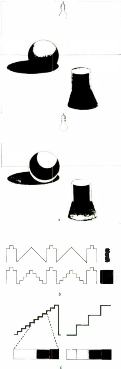
**FIG. 5—POSTERIZATION CHANGES GRADUAL shading to discrete transitions (a). In b we see how the normal video signal, which originally represented increasing and decreasing ramps, is changed to a staircase. In c we see how posterization creates grain at each transition. The grain isn't necessarily a problem because it's often used as a special video effect.**
