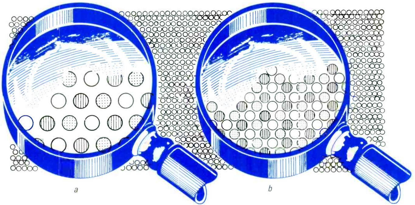
**FIG. 5—RESOLUTION** is determined by the number of dots, their size, and their spacing. Inexpensive monitors have relatively large dots spaced far apart (a). High-res monitors decrease dot size and spacing (b).
