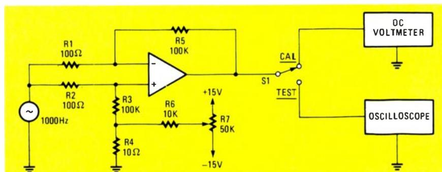
**FIG. 6—TO MEASURE CMRR,** use this test setup. With the 1000-Hz source off, adjust R7 for zero volts DC. Next, apply the test signal and measure the output with the oscilloscope. Last, calculate CMRR as discussed in the text.
