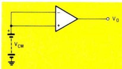
**FIG. 5—SLIGHT GAIN DIFFERENCES** between the inverting and the non-inverting inputs produce an erroneous output voltage. The ratio of the output voltage to the common-mode input voltage is the common-mode rejection ratio.
