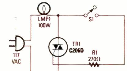
FIG. 15—SIMPLEST TRIAC CIRCUIT is composed of a switch, a resistor, and a Triac.
