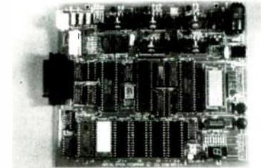
**BUILD STEVE CIARCIA'S INTELLIGENT SERIAL EPROM PROGRAMMER.** • Use Standalone or with Computer/Terminal; • Programs Standard or Fast Algorithm Mode; • Menu Selectable, No Configuration Jumpers; • Programs All 5V 27XXX EPROMs from 2716 to 27512. Includes CMOS and 12.5V Vpp; • Read, Copy, Verify after Write; • Intel Hex File Upload/Download. Full Programmer Kit **\$199.00,** Power Supply add **\$19.00.** S&H **\$5** in USA. CCI, 4 Park St., Suite 12, Vernon, CT 06066. (203) 875-2751.
