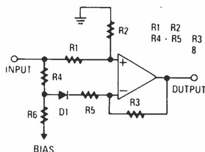
FIG. 9—BY VARYING THE FEEDBACK characteristics of an op-amp, a single stage of amplification can be made to function as a solarizer.
