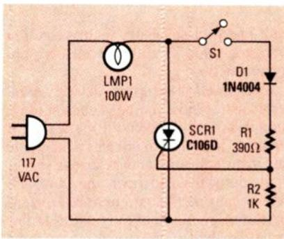
**FIG. 9—AC POWER-CONTROL CIRCUIT:** Close S1 to apply power to the load. After opening S1, the circuit will de-energize at the next zero crossing of the AC signal. Power is only delivered to the load during positive half-cycles.
