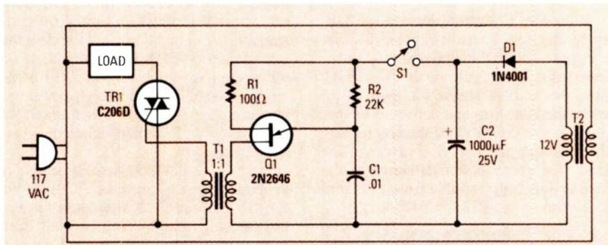
FIG. 14—THE CONTROL CIRCUIT connected to the secondary of T2 causes UJT Q1 to oscillate at about 50 Hz. The secondary circuit is isolated from the primary circuit here, unlike the previous figure.
