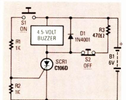
FIG. 7—ADDING A RESISTOR (R3) to the previous circuit allows you it to latch on. Turn it off by pressing S2.
