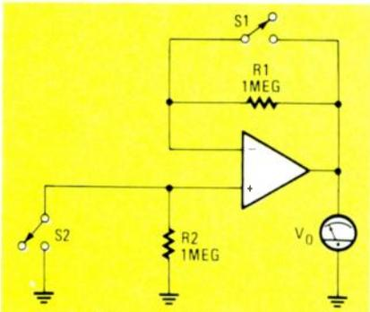
**FIG. 3—OFFSET VOLTAGE AND CURRENTS** may be measured with this circuit, depending on the state of S1 and S2.
