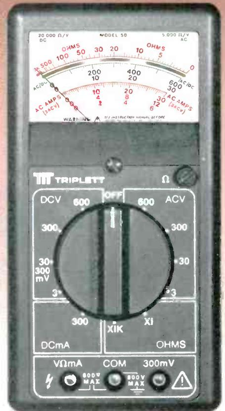
1. Rugged 12 range V-O-M; single range switch for convenience and minimizes error.
