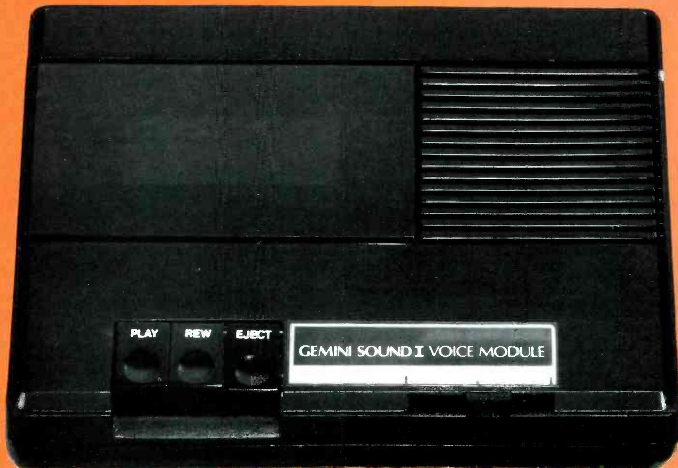
COLECO ADDS VOICE to the Atari 2600 with the Gemini module that uses special cartridges & tapes.
