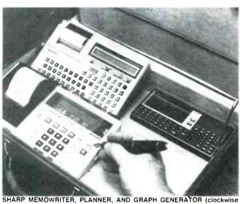
SHARP MEMOWRITER, PLANNER, AND GRAPH GENERATOR (clockwise from upper left) can indeed fit in an attache case, with room for some extra memo paper.
