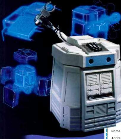
HERO 1 is a computer on wheels. HERO 1 uses a 6808 microprocessor that controls 13 functions and sense boards. Its on-board processor can take it through complex maneuvers. The programming process is straightforward with provision for step-by-step debugging, enhancement and other corrections.
