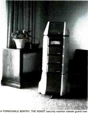
the home. For that purpose it is equipped with microwave, passive infrared, and audio discrimination detectors. The robot is made by Robotics International Corp. of Jackson, MI.
