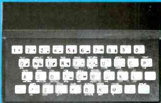
FIG. 4—A MEMBRANE KEYBOARD such as this one used on the TI new Sinclair 1000 (Sinclair ZX81) has character, graphics, and BASIC key functions imprinted directly on the membrane—there are no "real" typewriter keys.
