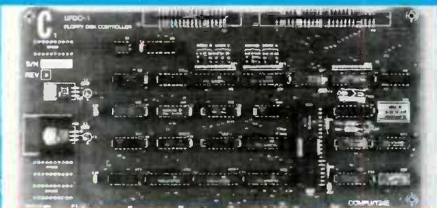
FLOPPY DISK CONTROLLER model UFDC-1 from CSR Computers, is capable of connecting up to four floppy-disk drives to an S-100 system.
