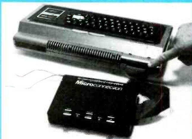
FIG. 3—THIS SPECIAL MODEL of the *Microconnection*, the model UMI from the Microperipheral Corporation, works with the Radio Shack TRS-80 Model I and eliminates the need for the RS-232 expansion interface.
