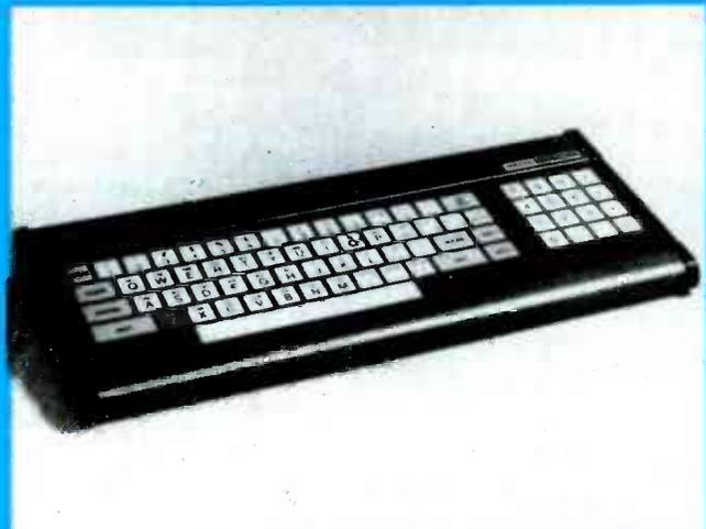
FIG. 3—The RCA VP3501 Videotex Data Terminal includes, among other features, a built in modem and built in tone and white-noise generators.
