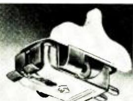
tridge in its special holder, which may be installed in almost any standard arm. The arm should be lightened for a 6-gram stylus force. Output is 1 volt at 1,000 cycles from the RD90 test record.
