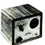
An ideal way to learn radio. This kit is complete ready to assemble, with tubes and all other parts. Operates from 110 V. AC. Simple, clear detailed instructions make this a good radio training course. Covers regular broadcasts and short wave bands. Plug-in coils. Regenerative circuit. Operates loud speaker. Shipping Wt., 3 lbs.
