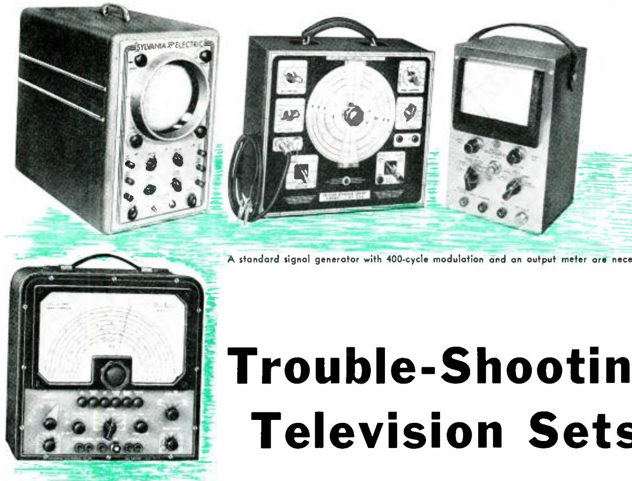
A standard signal generator with 400-cycle modulation and an output meter are necessities.
