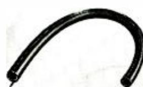
conductors. The new tubular 300-ohm Twin-Lead made especially for reception (like the tubular transmitting lines introduced by the company last year) has the conductors separated mainly by the enclosed air space within the tube. Thus dirt collecting on the outside of the tube does not lie between the conductors and has little effect on electrical characteristics. Additional features are lower wind resistance and greater strength.
