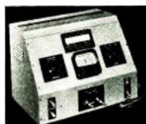
and grading capacitors. It may be used by non-technical personnel to obtain results within 0.2%. The range of the reading is 10  $\mu$ uf to 1,000  $\mu$ uf. The meter is a 4-inch direct-current D'Arsonval type.
