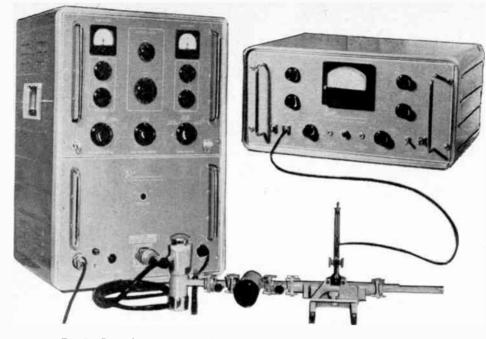
Fig. 5. Setup for measuring VSWR with modulated signal generator system.
