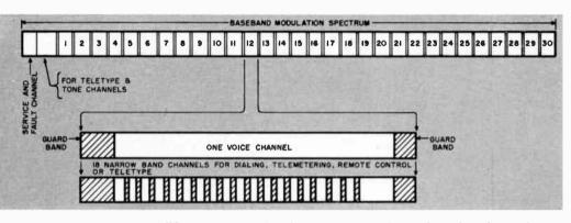
Fig. 4. The MM-26 system provides 30 voice channels, 20 tone channels and a service channel. Each voice channel can be further subdivided into 18 narrow-band channels.
