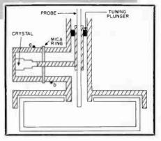
Fig. 2. Standing-wave crystal detector.
