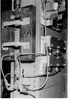
Fig. 6. Close-up of duplexer-coaxial switch assembly on the end of the rack.
