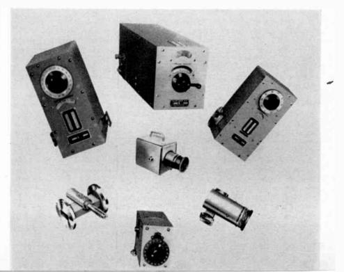
They can be operated either wide-band or selective. Selective operation is most sensitive and allows the exclusion of noise interference. The amplifier output meter scale is calibrated to read directly in VSWR when the amplifier is fed by a square-law detector such as a crystal diode.
