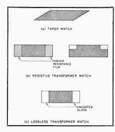
Fig. 12. Methods of matching resistive elements in wave guide attenuators.
