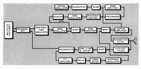
Fig. 3. Diagram of terminal station, including receiver, transmitter and a.f.c. unit.
