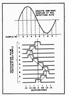
Fig. 7. A simplified drawing of the waveforms as used in PPM modulation.
