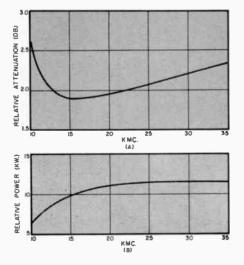
Bandwidth is greater and cutoff frequency lower than for comparable nonridge guide.
