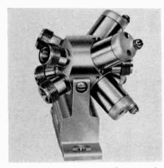
with coaxial switches. Performance is said to be excellent for frequencies up through X band.
