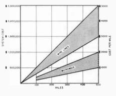
Fig. 2. The estimated initial cost of microwave and wire line installations.
