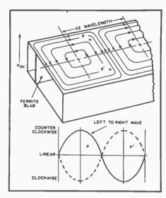
Fig. 6. Magnetic field contours in planes parallel to broad face of wave guide and resultant polarizations.
