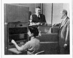
eration at the General Electric Company, Schenectady, N. Y. Capable of remembering up to 2000 ten-digit numbers and locating any one of them in three-thousandths of a second, it fills the gap between superspeed electronic computers and standard punch-card type equipment.
