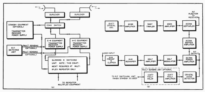
Fig. 3. Block diagrams of (A) the multiplexed repeater assemblies and (B) the various transmitter stages.
