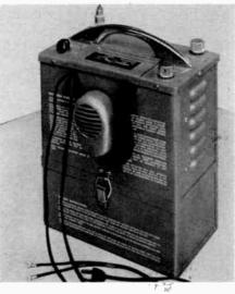
automatically switches off, the powerconsuming radio tubes if no incoming signal is present. Clear FM voice signals are reproduced on the built-in loudspeaker.
