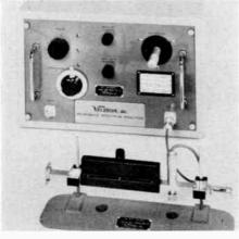
microwave tuning units including r.f. assembly and K-band mixer. They were specifically designed for use with the SA25 microwave spectrum analyzer, but other analyzers can be modified or adapted to use these assemblies.
