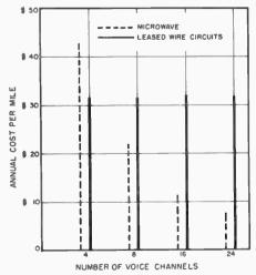
can be easily determined. In short systems, a dollars-per-mile rule-of-thumb figure doesn't work readily because of widely varying tower costs. However, in long systems, tower costs generally balance each other out so that a rough dollars-per-mile figure can be computed. This works out to about \$1000 to \$2000 per mile in most instances and is determined by the complexity of the system. The cost per mile of a microwave system generally decreases with length.
