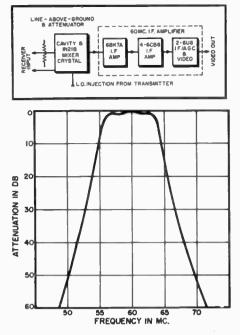
Fig. 5. Block diagram (top) and selectivity curve (bottom) of receiver.
