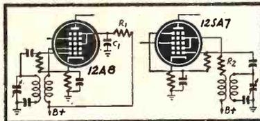
3—Using the 12SA7 suppressor as a screen is not satisfactory because of possible secondary emission. Oscillation and low gain might result in some cases.
