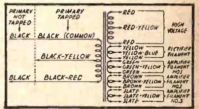
There are still old sets in use which follow other codes. Replacement parts for these may follow the original coding. The Serviceman is warned to be sure that the coding of a part is standard before taking it for granted. Green usually runs to grid and black to ground, when other leads are non-standard.
