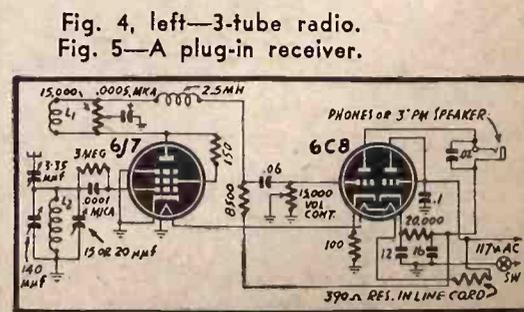
Fig. 4, left—3-tube radio.
