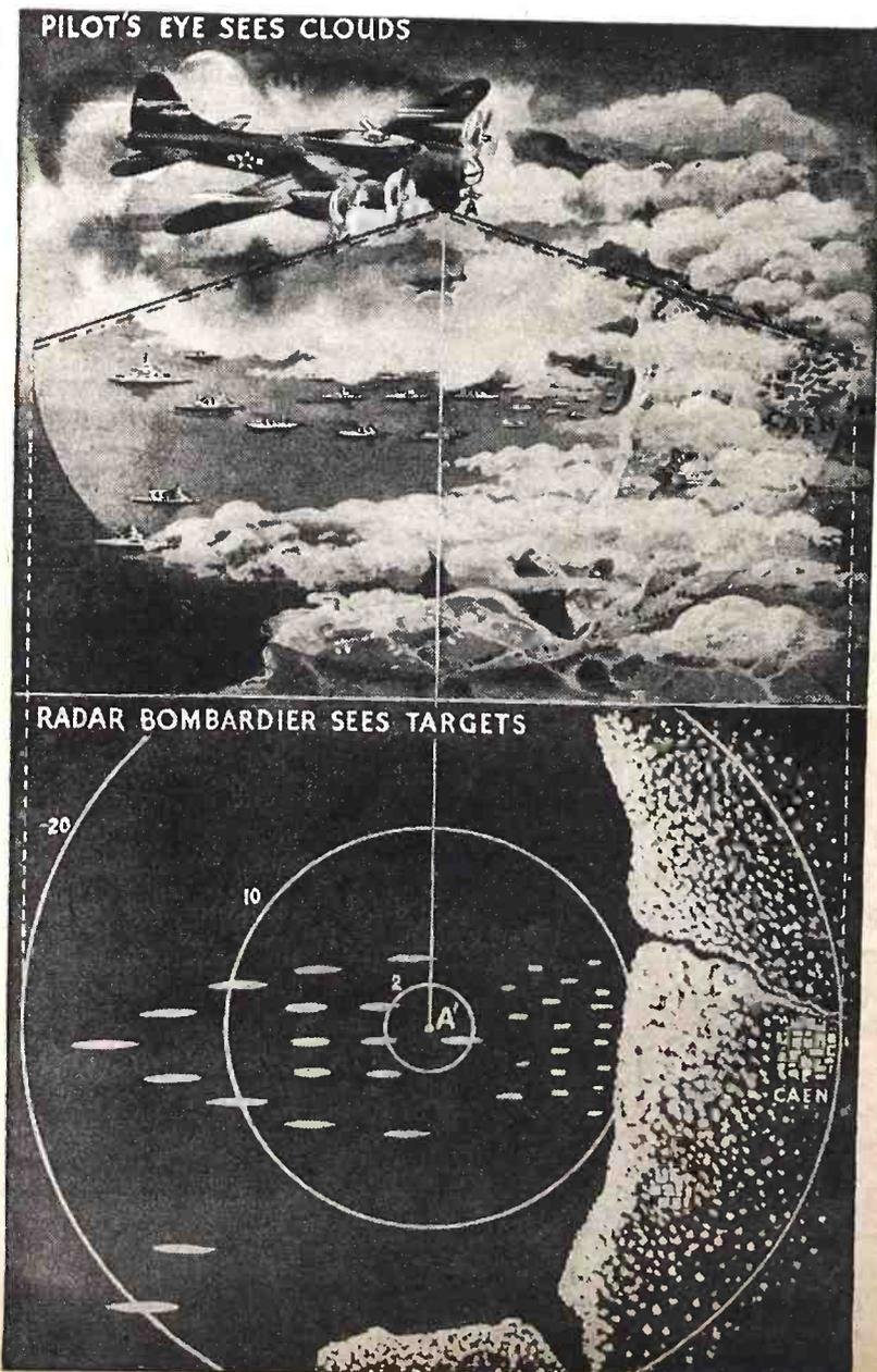
This drawing, released by Philco Radio Corp. last month, shows bomber equipped with radar bombsight flying above the Normandy coast 30 minutes before invasion landings. The scene below is the image on the cathode-ray tube screen. The eye of radar sees a clear picture of territory beneath, invisible to the men in the plane. It was due to radar-controlled bombing that the Normandy coast defenses were knocked out entirely before our men landed.
