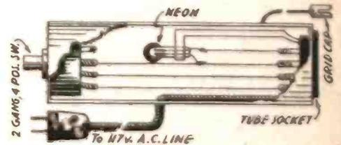
Internal construction of the pocket tester.
