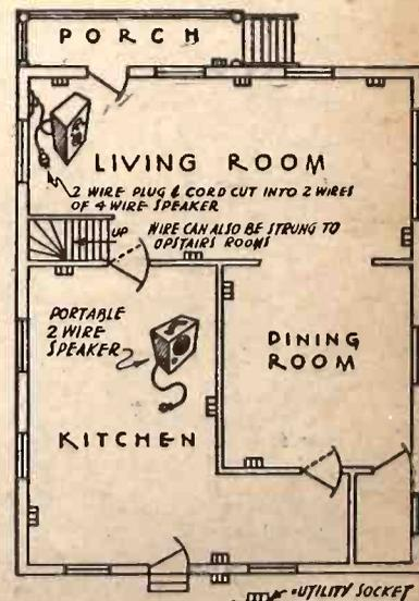
wires throughout the house terminating in each room with a utility plug. I have a small PM speaker which I can carry anywhere and plug into a socket in any room I happen to be in. A small volume control and switch is built into the housing of each speaker.
