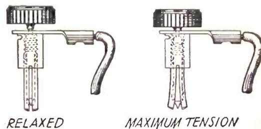
Fig. 1—This connector is absolutely secure in position once inserted and screwed down tight. The shell is crimped in near the top (see notch) thus making impossible removal of center screw.
