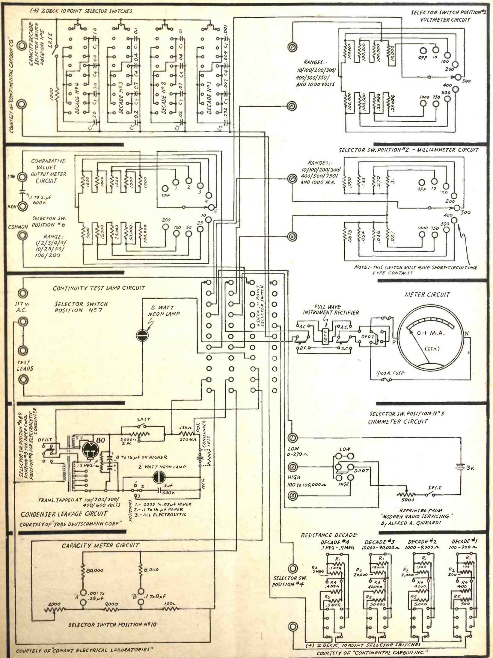
A voltmeter, milliammeter for A.C. and D.C., multi-range ohmmeter, decade boxes for resistance and capacity, an output meter, leakage testers for paper and electrolytic condensers, a lamp unit for continuity checking and a capacity analyzer are contained in this unit.
