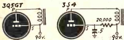
Fig. 3—How screen voltages may be lowered.
