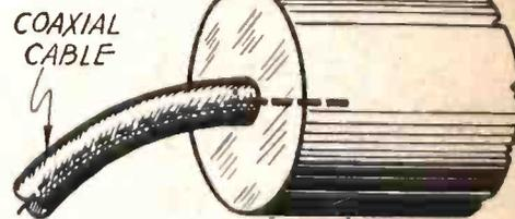
Fig. 6—Cylindrical waveguide with end feed.
