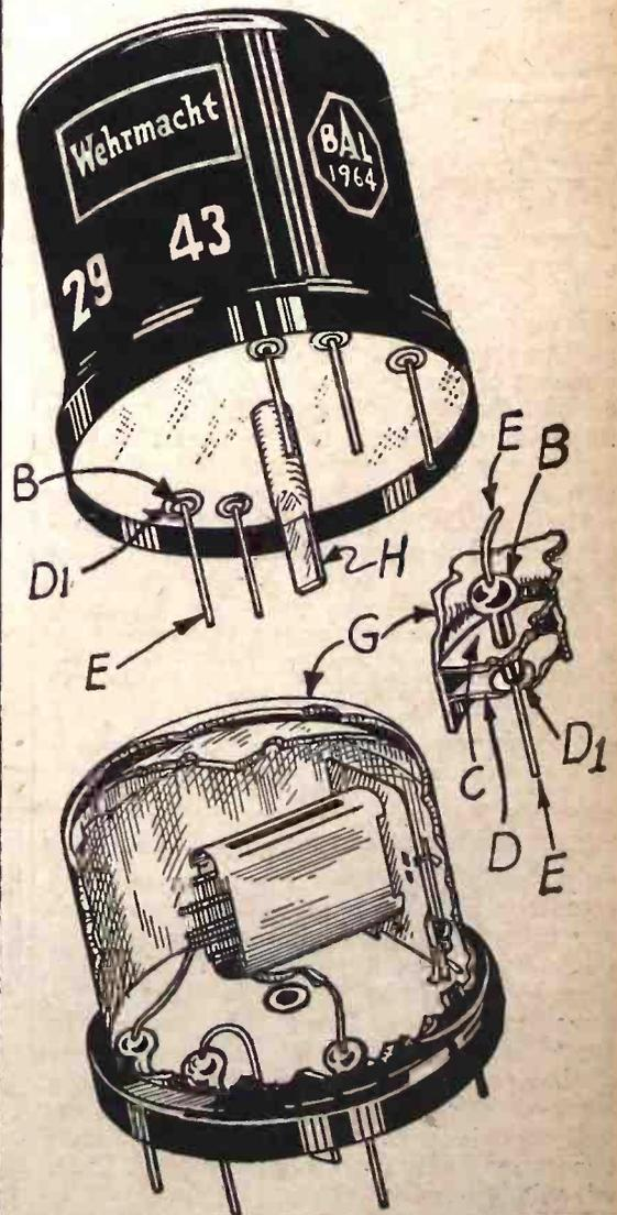
Fig. 2—Wehrmacht tube. B—Glass insulating bead. C—Upper platform. D—Lower platform. D1—Metal-to-glass header ring. E—Lead to interior elements. G—Shell. H—Copper tube shown crimped after sealing-off.
