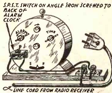
Merely set the clock to ring at the end of your favorite program. When it goes off, the wing nut turns the switch to "off" automatically.
