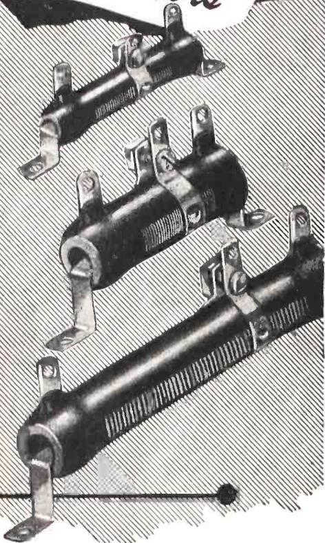
Ohmite "Dividohms" make ideal voltage dividers by the use of one or more adjustable lugs. Also handy for obtaining odd resistance values, for adjusting circuits, and for use on equipment which must be set to meet various line voltages.
