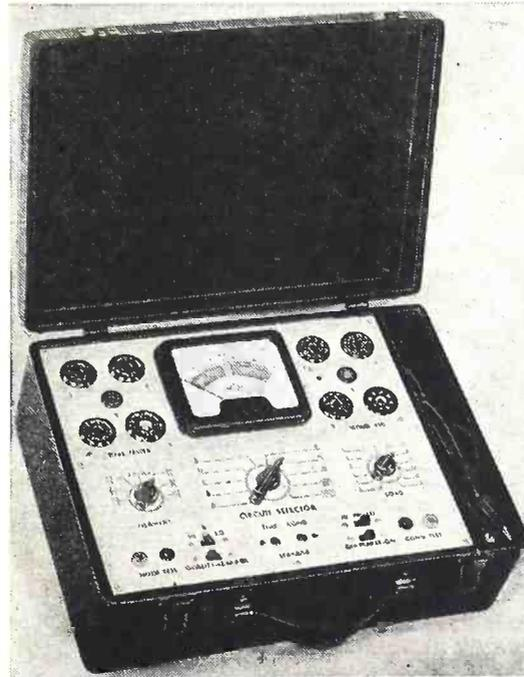
EXTRA SERVICE—The Model 450 may be used as an extremely sensitive Condenser Leakage Checker. A relaxation type oscillator incorporated in this model will detect leakages even when the frequency is one per minute.
