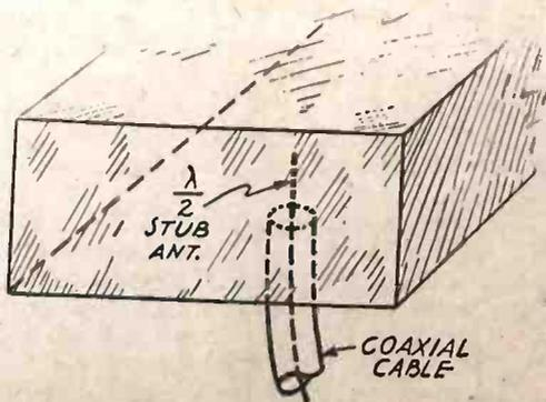
Fig. 5—A square waveguide with lateral feed.
