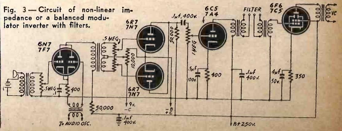
Fig. 3—Circuit of non-linear impedance or a balanced modulator inverter with filters.
