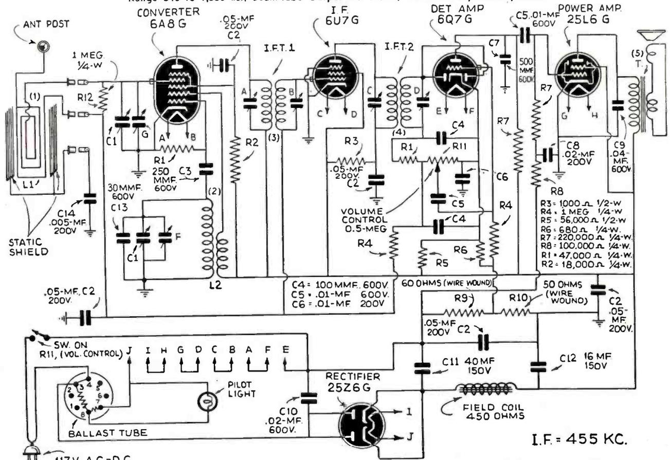
117V. A.C.-D.C. Diagram of the A.C.-D.C. portable loop receiver. Ideal for hotels, hospitals, offices and apartments, in fact any type of home.
