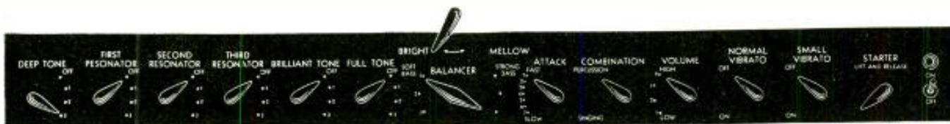
Fig. 1. Here are the "voice" controls, of the Novachord, which convert an otherwise string-less "piano" into an entirely new electronic musical instrument.
