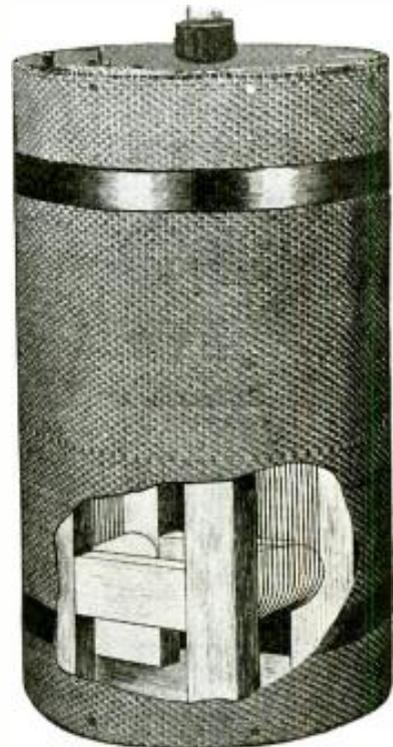
A shield around the loop stops static.
