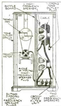
Fig. 3. Cross-section of the Tone Chamber showing 2 of its 3 speakers and the motor-driven sound shutter for producing tremolo effects. A similar chamber with a self-contained amplifier is called a Booster Tone Chamber.
