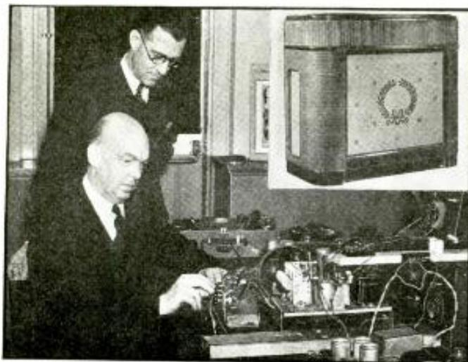
← Major Edwin H. Armstrong (seated) and Dr. W. R. G. Baker double-check the laboratory performance of the new General Electric experimental-type frequency modulation receiver; inset—the completed 11-tube receiver.
