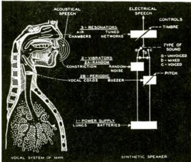
cavity; that is the way in which are made all the sounds of speech when one whispers, and such sounds as *s*, *th* and *f*. In the Voder there is an electrical hiss, and with some of the keys the operator can control its quality so as to make those sounds. Other keys make the "stop consonants" like *d*, *k*, and *p*.
