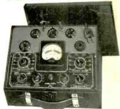
A really modern tube tester conforming to all standards of good engineering practice. Utilizes a 3" d'Arsonval type meter with calibrated scale. Furnished in a sturdy black case with sloping panel for easy operation. Removable cover and carrying handle for either portable or counter use.
