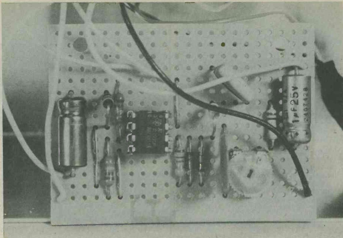
Component layout on the Veroboard panel
