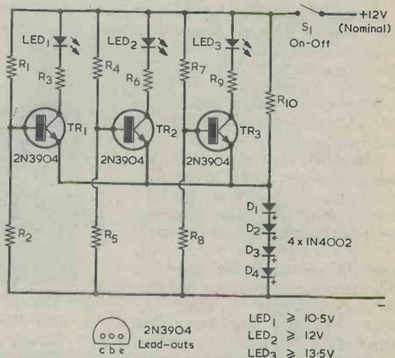
The circuit of the battery voltage monitor. Voltage is indicated by the number of l.e.d.'s which are alight.
