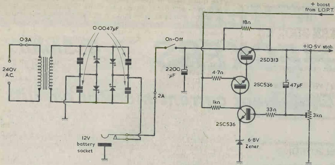
Fig. 4. The circuit of the power supply section of the television receiver. The rectified voltage from the bridge rectifier passes through a normally closed contact on the battery socket to the receiver on-off switch, and thence to the 3-transistor voltage regulator. This circuit is employed in the Sanyo Model 12-T280.
