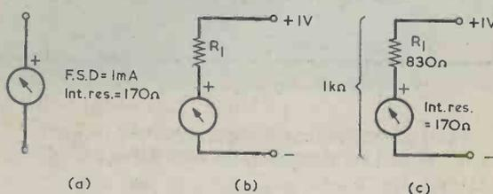
Fig. 1(a). A 0–1mA moving-coil meter movement. This can, typically, have an internal resistance of  $170\Omega$
