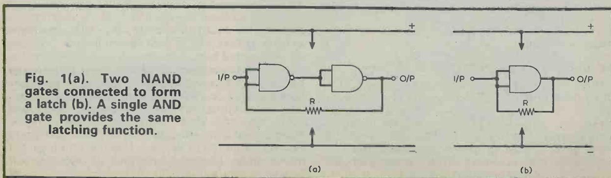
Fig. 1(a). Two NAND gates connected to form a latch (b). A single AND gate provides the same latching function.
