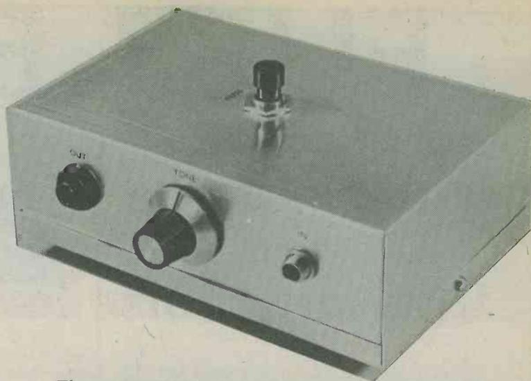
The completed fuzz unit in its aluminium case. The successional action foot operated switch on the top panel switches the fuzz effect in and out.
