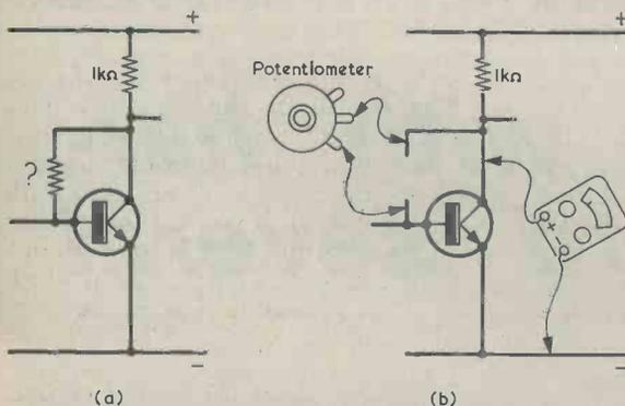
**Fig. 2(a).** In an experimental circuit the bias resistor, whose value is unknown, is required to have a value which causes the transistor collector to be at mid-supply potential.
