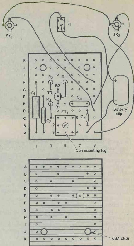
Fig. 2. The wiring on and around the Veroboard. IFT1 is soldered in place first, using a procedure which is described in the text
