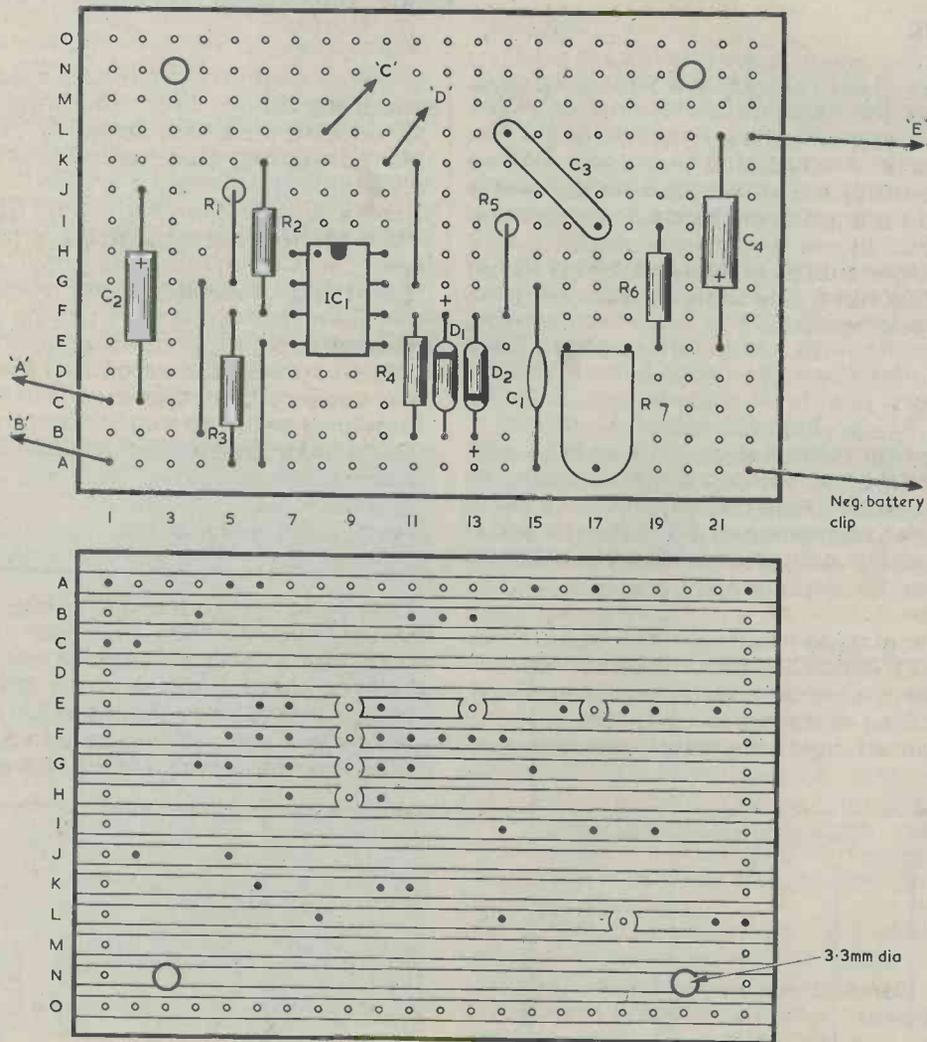
Fig. 3. The component and copper sides of the Veroboard panel. The wires designated "A" to "E" connect to the similarly identified points in Fig. 4.
