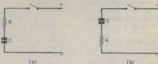
Fig. 1(a). When the switch is closed the voltage across the capacitor rises and reaches 63% of the supply voltage after a period equal to the time constant of the resistor and the capacitor (b). With this circuit the voltage across the capacitor increases in the same way after the switch closes, but the voltage on the lower plate is now negative-going
