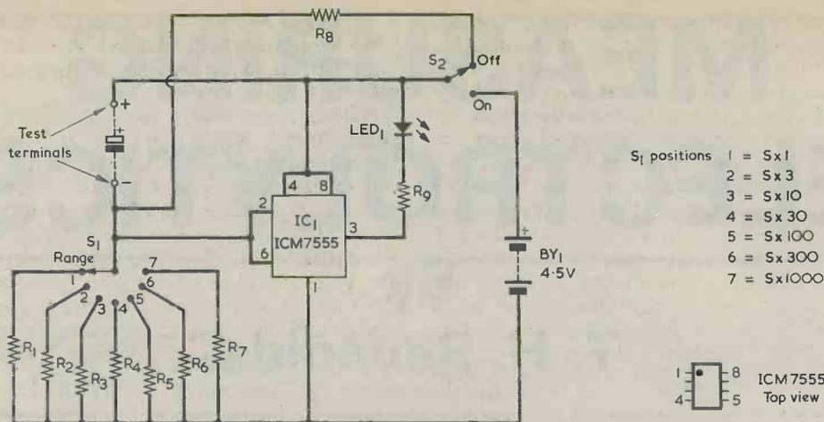
**Fig. 2. The circuit of the capacitance measuring instrument. The test capacitance, in microfarads, is equal to the number of seconds the l.e.d. is alight multiplied by the appropriate figure for the setting of Range switch S1**
