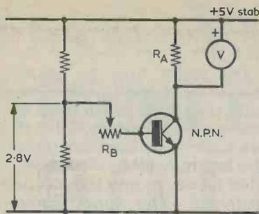
**Fig. 2.** This circuit can be used to measure the base-to-collector gain of a silicon n.p.n. transistor. RB is adjusted for an indication of 2.2 volts in the voltmeter, and this voltage also appears across RB.
