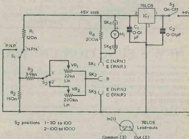
**Fig. 3.** The complete circuit of the transistor gain meter. C1 and C2 ensure stability in IC1, and should be positioned close to its lead-outs.
