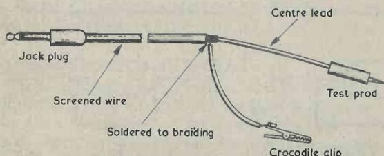
Fig. 3. Making up the test lead. This is plugged into SK1 or SK2 according to the function required
