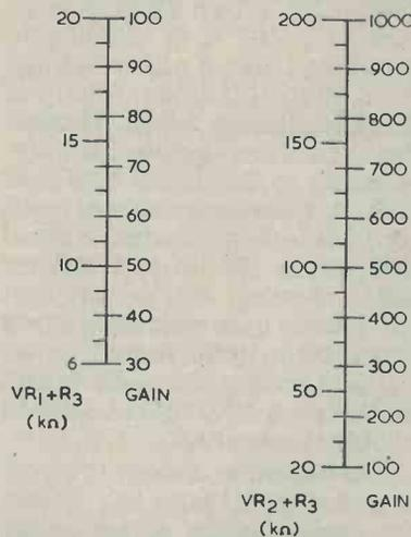
**Fig. 5.** Charts showing resistance in the series combinations of R3 and VR1, and of R3 and VR2, with the corresponding gain figures.
