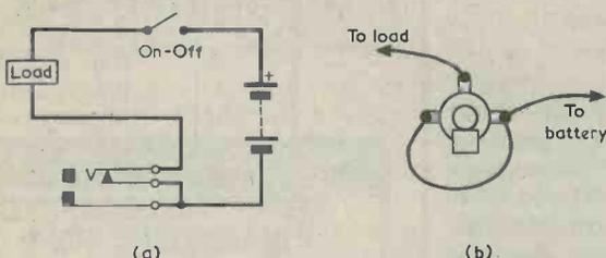
Fig. 1(a). Connecting a jack socket in series with the negative supply in an item of battery operated equipment. Current readings are obtained by inserting a jack plug connected to a testmeter which is switched to a suitable current range.
