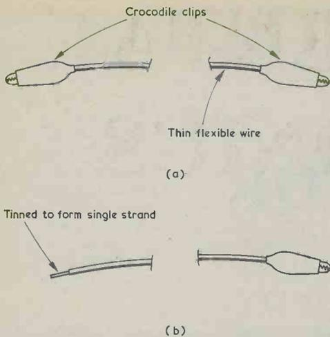
**Fig. 1(a).** Very useful for experimental work are crocodile clip leads. A range can be made up with wire lengths varying from some 4 to 7in.
