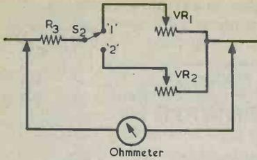
**Fig. 4.** VR1 and VR2 are calibrated for gain figures by connecting an ohmmeter in the manner illustrated here.
