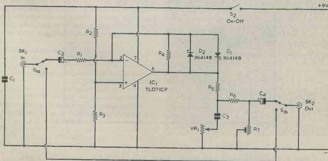
Fig. 2. The circuit of the fuzz box. Clipping is achieved by the two diodes in the feedback loop around IC1.
