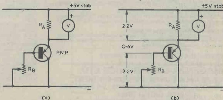
Fig. 1(a). A circuit which is capable of evaluating the base-to-emitter current gain of a p.n.p. silicon transistor.
