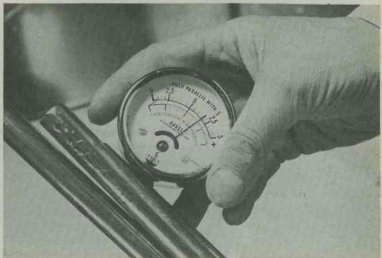
A pocket magnetometer available from Leavers-Rich Equipment Limited. This measures from -5 to +5 gauss in 0.5 gauss stages.
