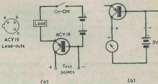
Fig. 2(a). A more unusual approach. The base-emitter junction of a p.n.p. transistor is permanently connected in the negative supply line.
