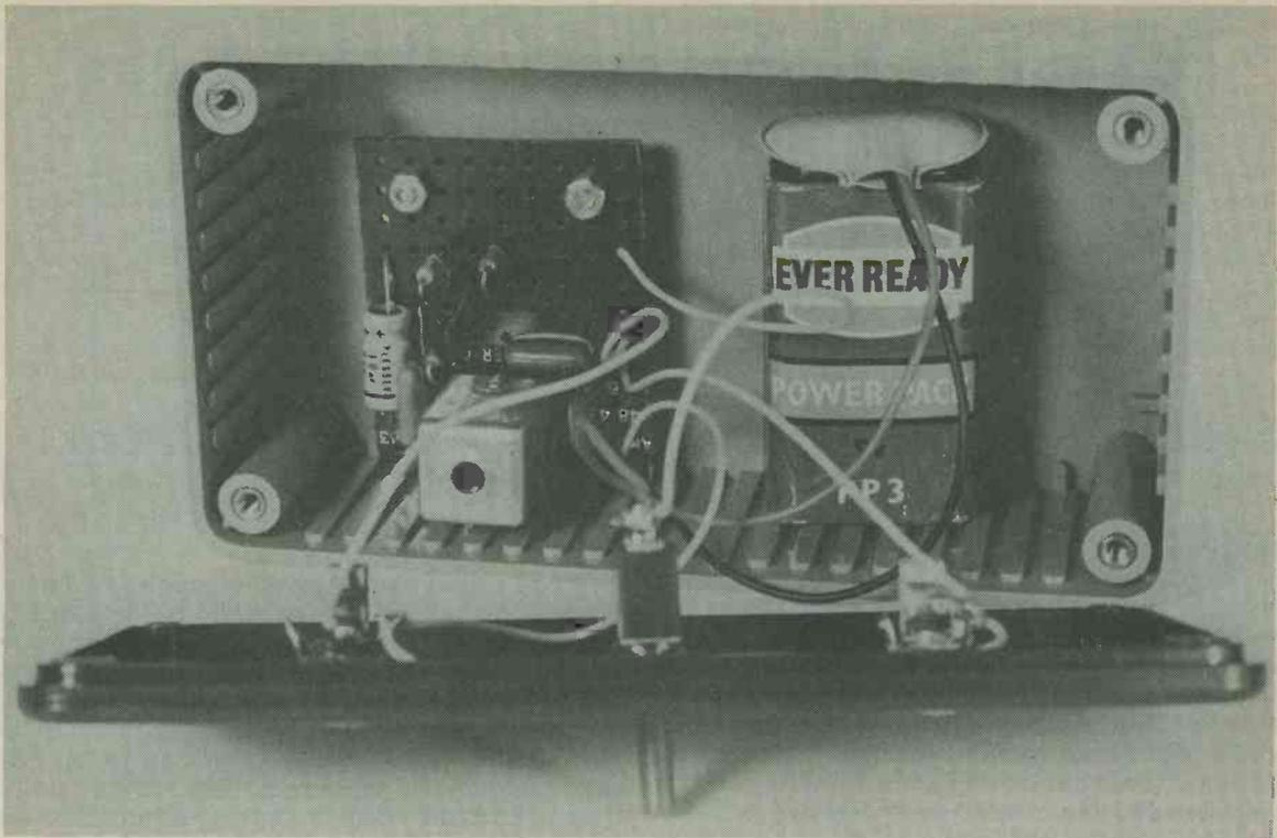
The Veroboard assembly is secured to the rear panel at the left, with the battery to the right
