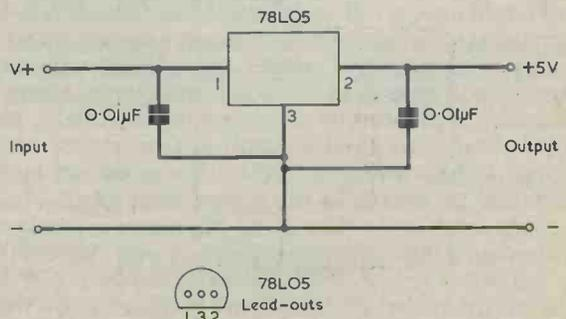
Fig. 1. The normal circuit in which the 78L05 voltage regulator is employed.
