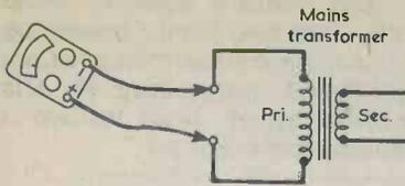
Fig. 3. Smithy used a mains transformer with no connection made to its secondary to demonstrate the types of resistance reading which can be obtained at the primary.
