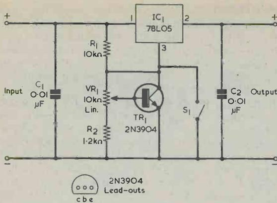
**Fig. 2.** With this circuit the stabilized output voltage may be varied from about 5.6 to slightly more than 10 volts by adjusting VR1. Closing S1 produces a 5 volt stabilized output.
