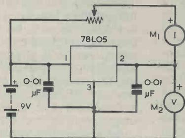
**Fig. 3.** An experimental circuit in which current is drawn from the regulator output in the opposite direction to normal.
