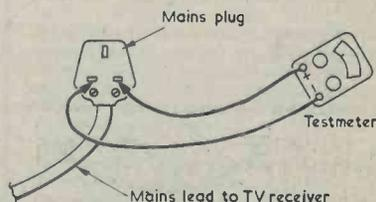
Fig. 1. Dick applied the leads of his testmeter, switched to a low ohms range, to the live and neutral pins of the mains plug connected to the television receiver he was examining.
