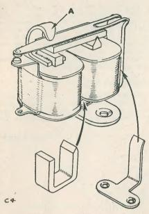
Fig. 4. Secondary relay
