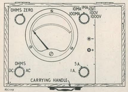
Fig. 2. Layout of panel and controls
