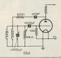
Fig. 1 shows a useful modification to the reaction circuit, which just consists of a resistor joined between the reaction condenser and the reaction coil. The effect is to alter the phase angle instead of the amplitude of the feedback. The result is very much the same, but is very much smoother. The value of the resistor can be almost anything between 100 and  $5{,}000~\Omega$ ; if it is too high the reaction
