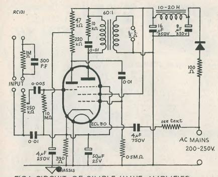
FIG.I CIRCUIT OF SIMPLE VALVE AMPLIFIER
