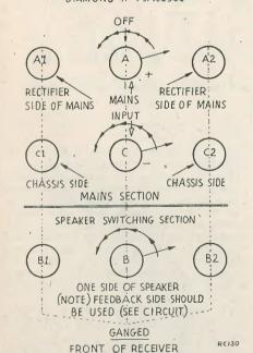
NOTE: The contact positions of this switch are at 45°, as against the 30° of ordinary Yaxley types. To suit the markings on the specified knob, the mains output from switch to radio receiver should come from A1-C1, and speaker connection from B1.
