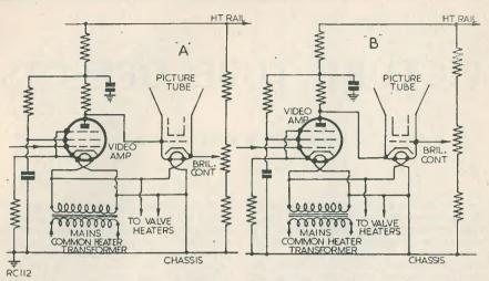
Fig. 1. Methods of modulating a picture tube:
