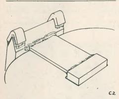
Fig. 2. Pole pieces of sensitive relay
