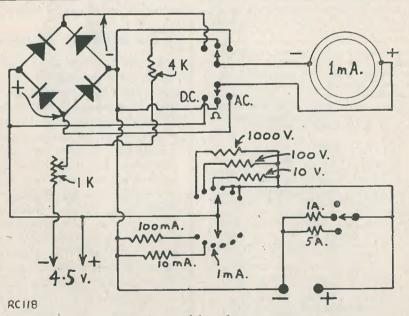
Fig. 1 Circuit of the multi-range meter
