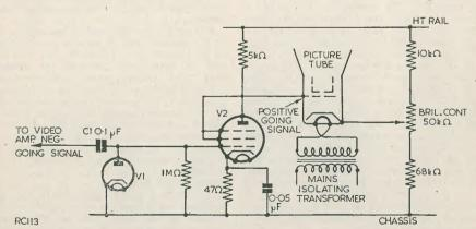
Fig. 2. Circuit changed to grid modulation enabling a faulty tube to be used
