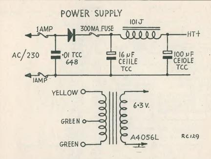
NOTE: The mains (230V AC) are connected to the two green leads of the heater transformer. The single yellow lead is ignored.
