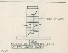
4 coils to a length of  $\frac{2}{3}$ ". This slight spacing of the turns increases the Q of the coil considerably.
