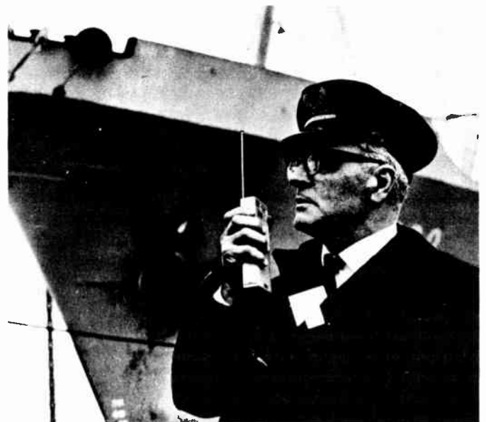
1964. This modern u.h.f. radio, the Pye Pocketphone, represented a breakthrough in police portable radio.
