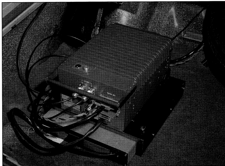
Figures 4. "Equipment Test" ET 3 piece Cellular Radio, Logic Unit shown here in the trunk of a 1978 Oldsmobile.
