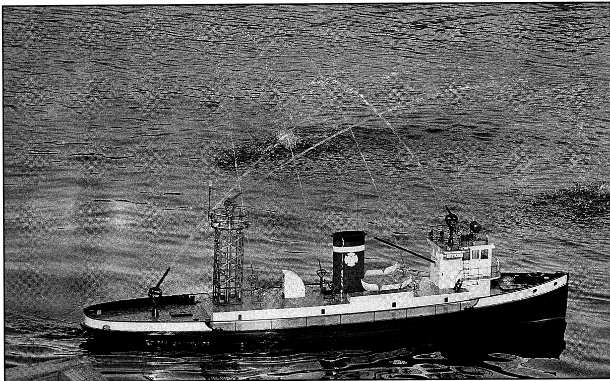
Photo 5. Model fire boat with all hoses working and controlled by the WSR. Courtesy of F.D. Reynolds.
