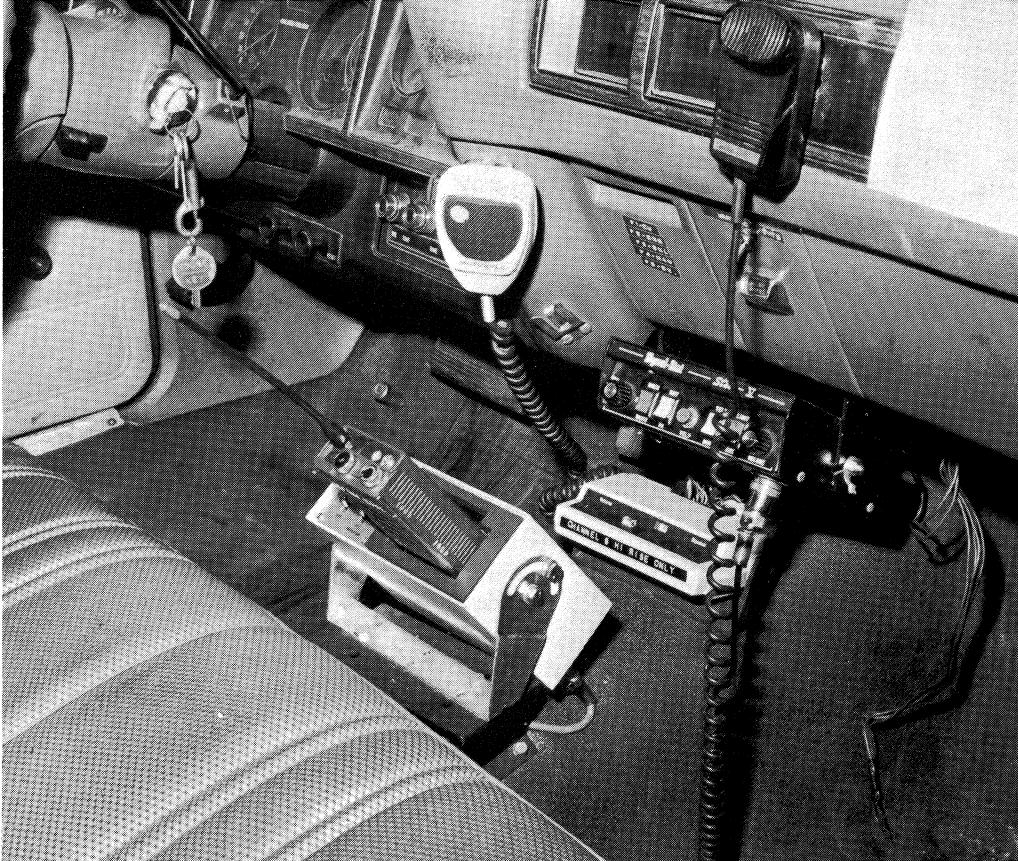
Fig. 5. UHF radio in charging pocket, with VHF repeater ahead of it.
