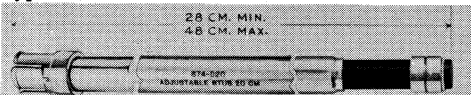
One 874-D20 Adjustable Stub For matching or tuning, and use as a reactive element. Coaxial lines with sliding short-circuit moved by bakelite tube. Reference marker for use as wave meter with scale. Maximum travel of short-circuit is 20 cm. $10.50
