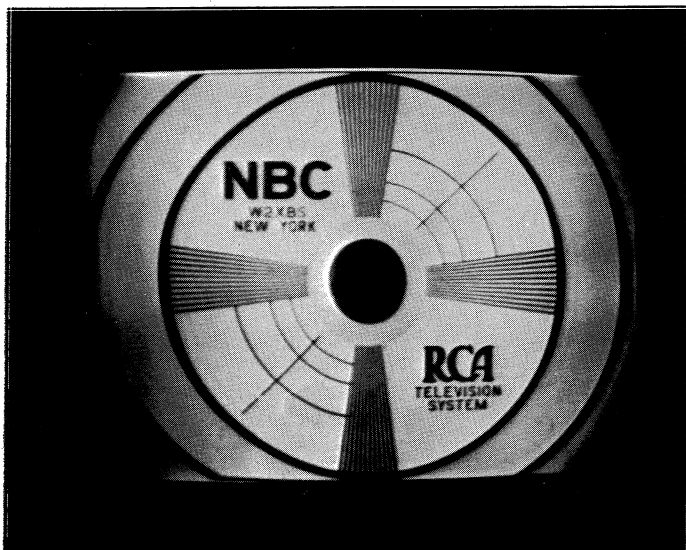
Fig. 4—Image received on typical amateur-built receiver with 1-millivolt r-f signal.
