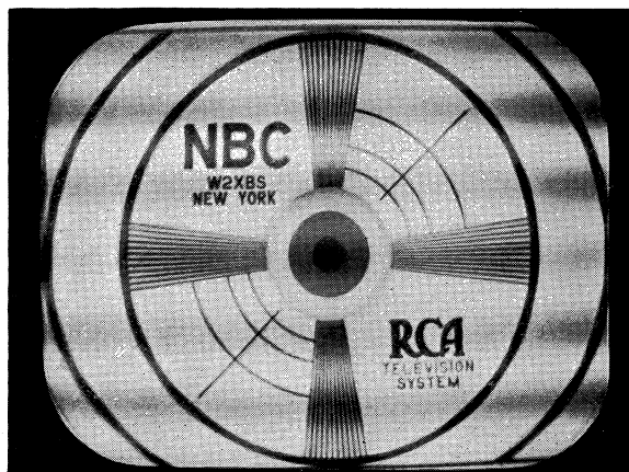
Fig. 17—Interference from audio frequencies in the signal circuit. May arise from cross-talk anywhere in transmission or reception system, but usually from inadequate trapping of sound intermediate frequencies at 8.25 or 14.25 Mc.
