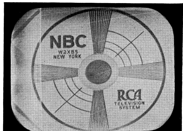
Fig. 12—Nonlinearity of horizontal scanning due to failure of the damping rectifier circuit.
