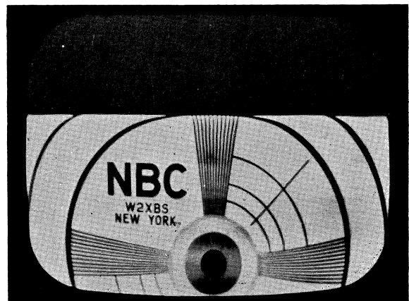
Fig. 6—Incorrect positioning due to excessive d-c component in vertical scanning circuit.
