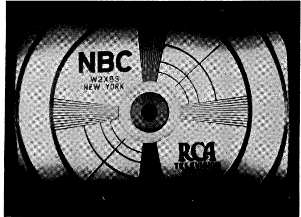
Fig. 10—60-c.p.s. hum in the video signal circuit.
