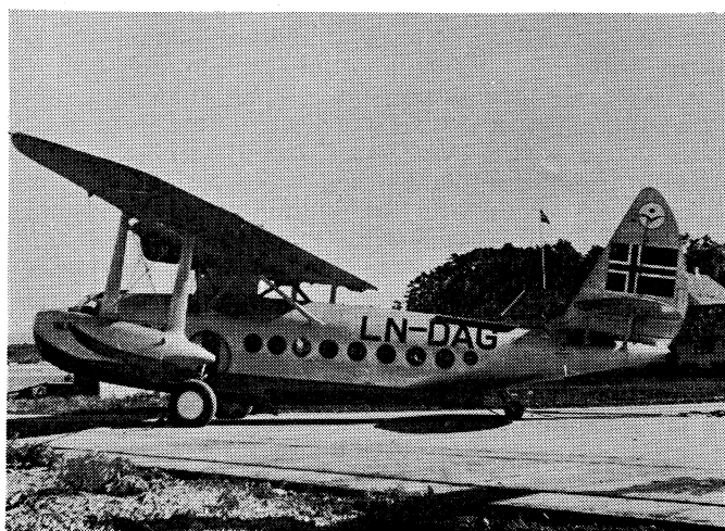
FIGURE 14 SIKORSKY S-43 EQUIPPED WITH R. C. 5 RADIO-COMPASS
