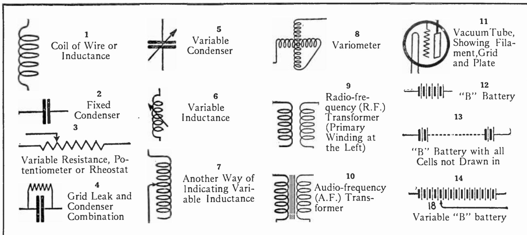
constant. The most common use in radio for a condenser of this type is in series with the grid lead of a detector tube, in which position it is known as the grid condenser, and its capacity is .0005 mfd. *This value, as well as other values indicated in the course of the articles, may be taken as standard and may be used in all circuits excepting those calling for special values which will always be specified.*
