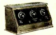
The Stewart-Warner Instrument shown is Model 305—a five tube set in which is incorporated the U. S. Navy Circuit. There are three tuning controls, mounted on a sloping front panel. The cabinet is finished in dark walnut.
