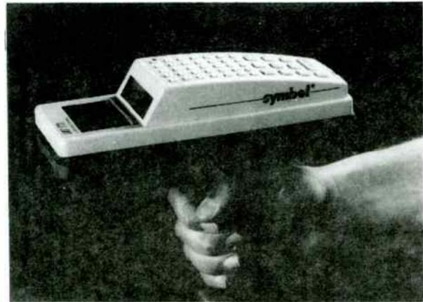
Figure 19 A Symbol Laser Radio Terminal
