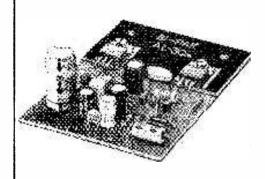
sistors attached to a small heatsink. The manufacturers recommend that for speech and music applications a total heatsink area of 10 sq.in. be used, and for higher power applications 15 sq.in. These figures are for mono use and should be doubled if two modules are used for stereo reproduction.
