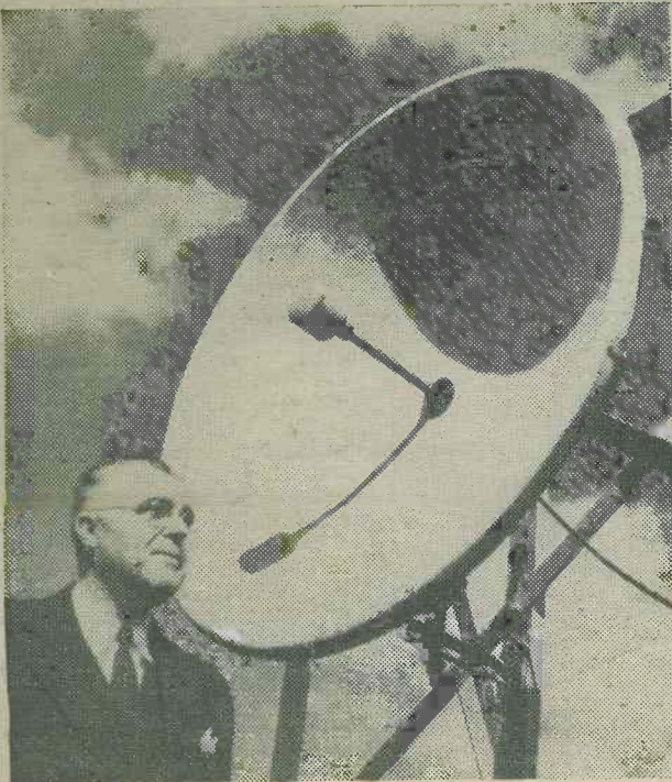
Radio relay towers are being used in a new communications system in the United States. Automatic, unattended radio towers are symbols of one of the most significant advances in communications in modern times. These towers may ultimately replace thousands of miles of telegraph and telephone lines in America. Our illustration shows a radio antenna of a tower on the roof of the 24-storey Western Union building.
