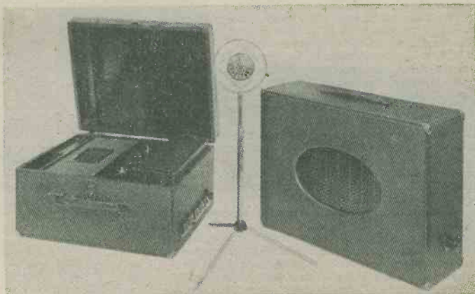
Fig. 1.—An A.C./D.C. portable amplifying equipment with transverse-current carbon microphone and cabinet loudspeaker, with carrying handle.
