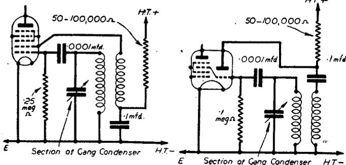
Fig. 1 (left).—The usual connections for an oscillator coil used with a pentagrid frequency-changer.
