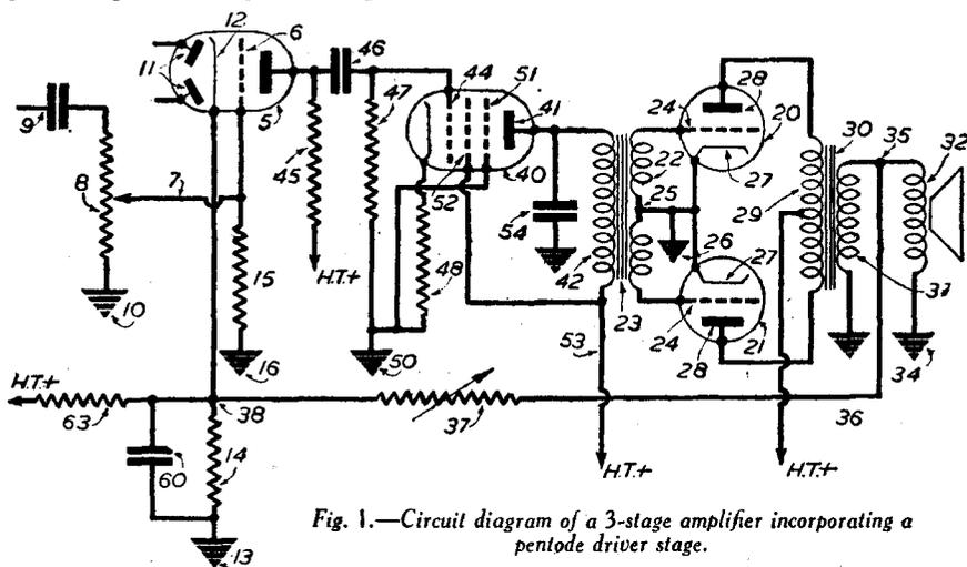
Fig. 1.—Circuit diagram of a 3-stage amplifier incorporating a pentode driver stage.
