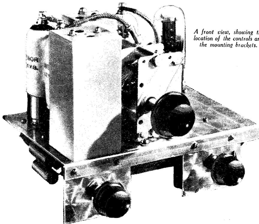
A front view, showing the location of the controls and the mounting brackets.
