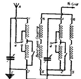
Fig. 9.—An inductive band-pass coupling using Lissen 5321's.
