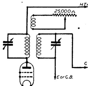
Fig. 4.—A variable-selectivity I.F. transformer of the type having a tertiary winding.
