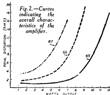
Fig. 2.—Curves indicating the overall characteristics of the amplifier.
