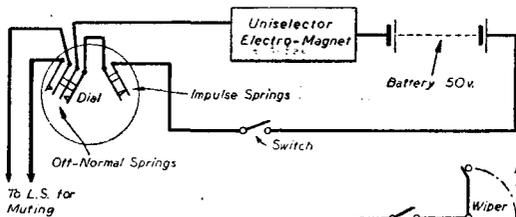
Fig. 1 (Left).—Circuit diagram showing the contact springs, and position of uni-selector unit.
