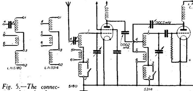
Fig. 5.—The connections for the Lissen coils L.N. 5180 and L.N. 5314. Fig. 6.—A suitable 3-valve circuit for the Lissen coils shown on left.
