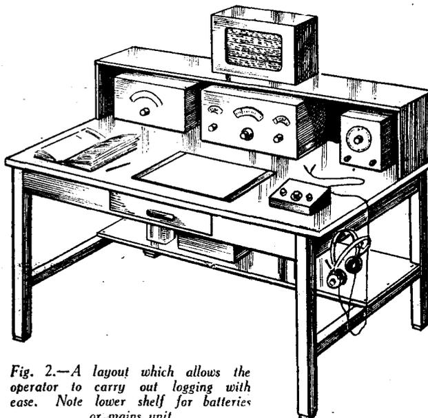
Fig. 2.—A layout which allows the operator to carry out logging with ease. Note lower shelf for batteries or mains unit.
