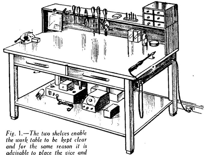
Fig. 1.—The two shelves enable the work table to be kept clear and for the same reason it is advisable to place the vice and soldering iron on opposite sides.
