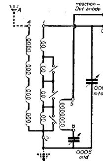
Fig. 11.—The connections of the Lissen Four-range coil are shown here. Some of these are still available.
