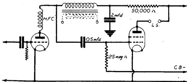
Fig. 5.—The secondary of an old L.F. transformer with burnt out primary makes a good L.F. choke for use in the detector anode circuit. The primary winding—shown in broken line—is not used.
