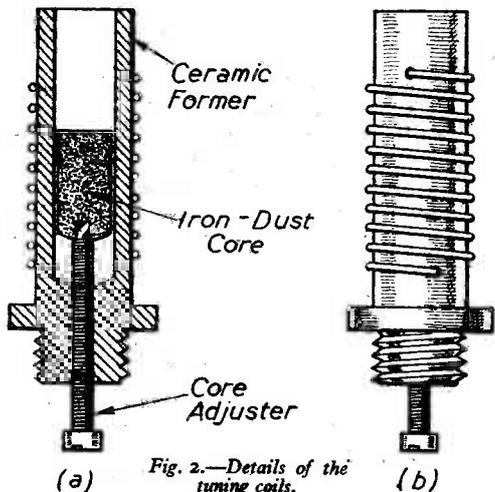
Fig. 2.—Details of the tuning coils.
