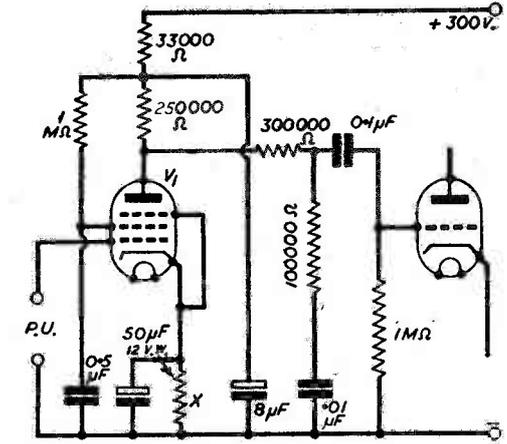
Fig. 8.—Bass boosting first stage (pentode).
