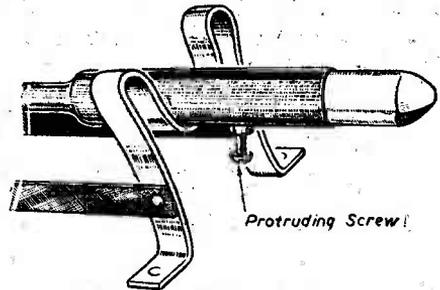
Keeping the soldering-iron in place.
