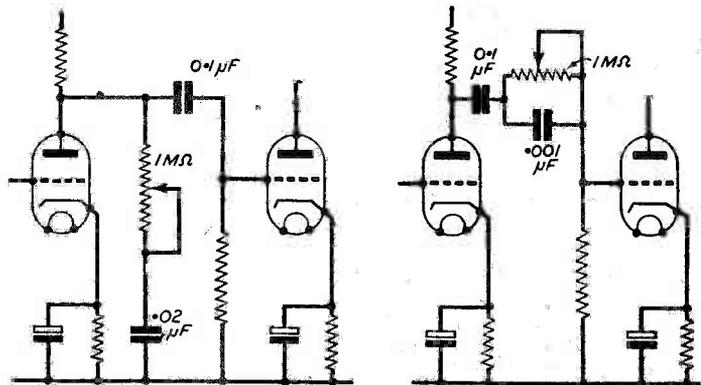
Fig. 3.—(a) Treble attenuator. (b)—right—Bass attenuator.
