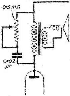
Fig. 12.—Simple treble attenuator.
