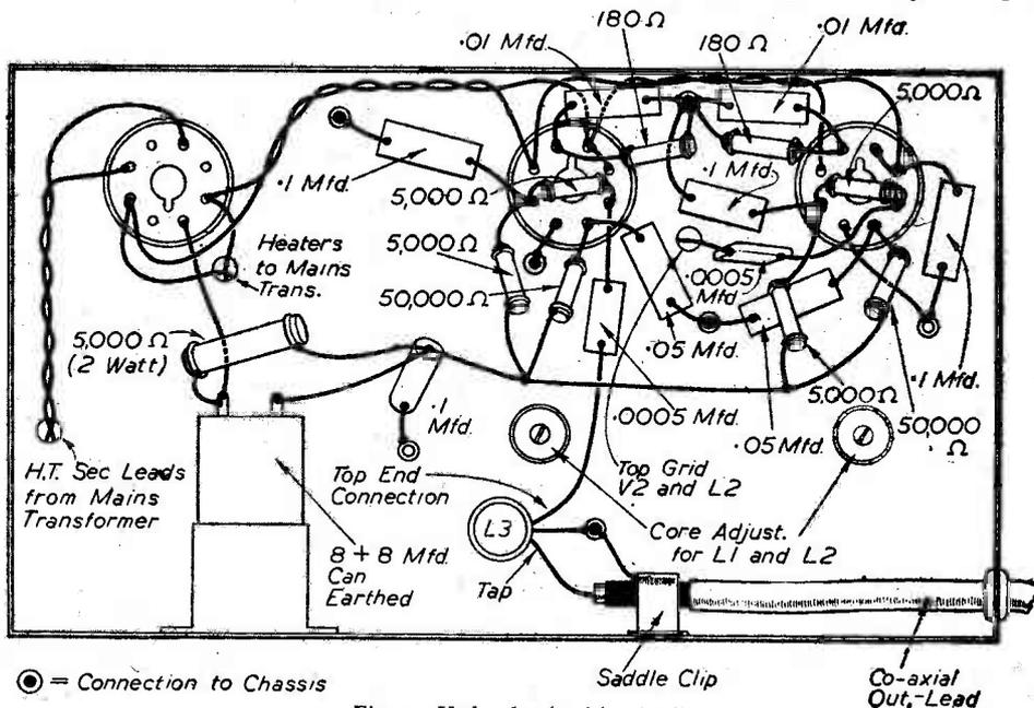
Fig. 4.—Under chassis wiring details.
