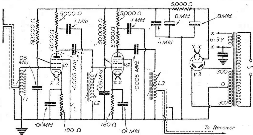
Fig. 1.—Theoretical circuit of the Pre-amplifier.
