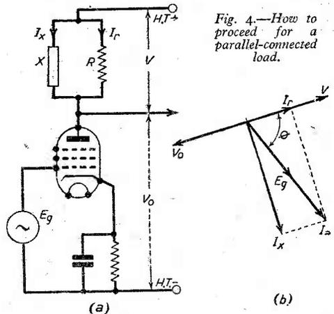
Fig. 4.—How to proceed for a parallel-connected load.
