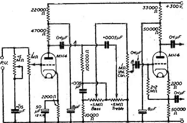
Fig. 9.—Remote tone and volume control circuit.
