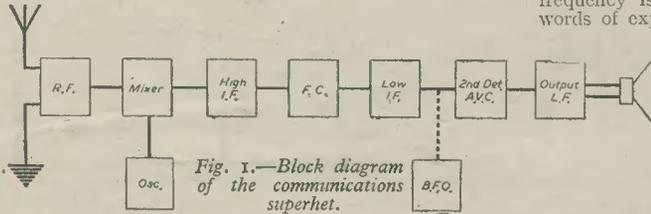
Fig. 1.—Block diagram of the communications superhet.
