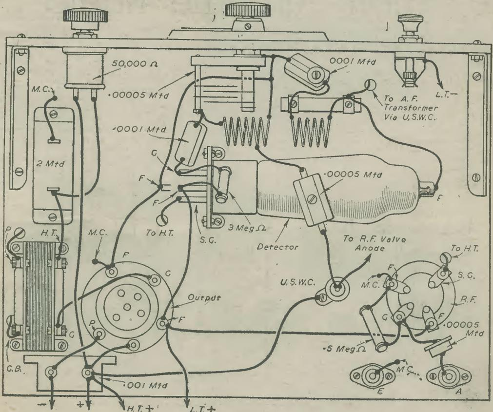
Fig. 3.—This shows the layout and wiring of the principal components of the U.S.W. Three.
