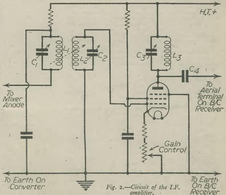
Fig. 2.—Circuit of the I.F. amplifier.
