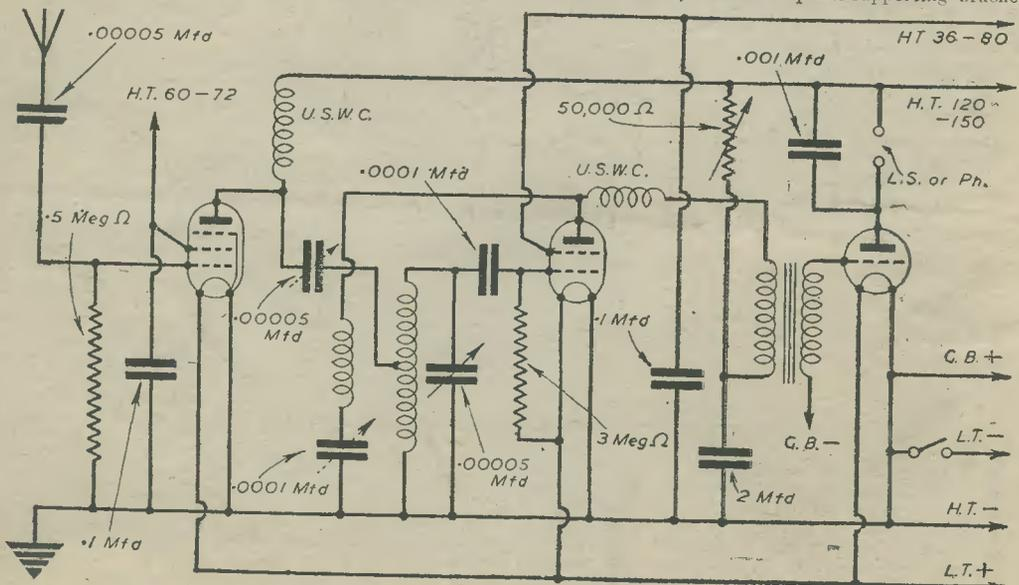
Fig. 1.—Theoretical circuit of the receiver.
