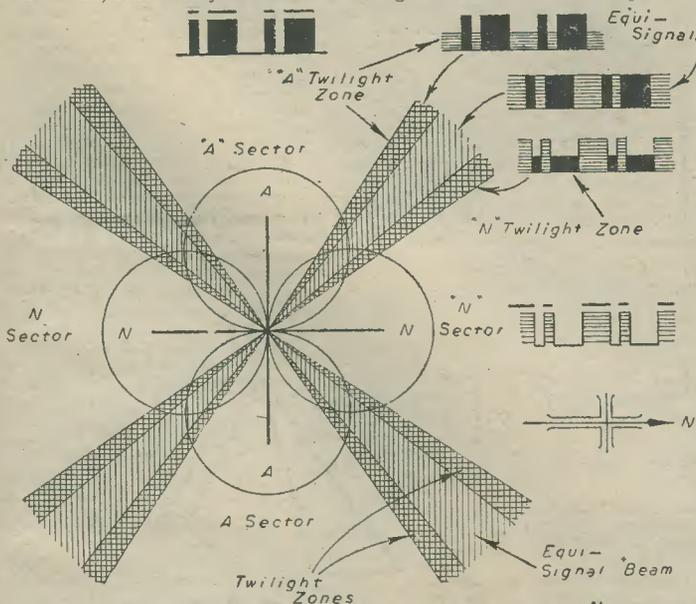
Fig. 1.—This diagram shows how the "A" and "N" sectors, and also the equi-signal "beams" of a radio range are obtained.
