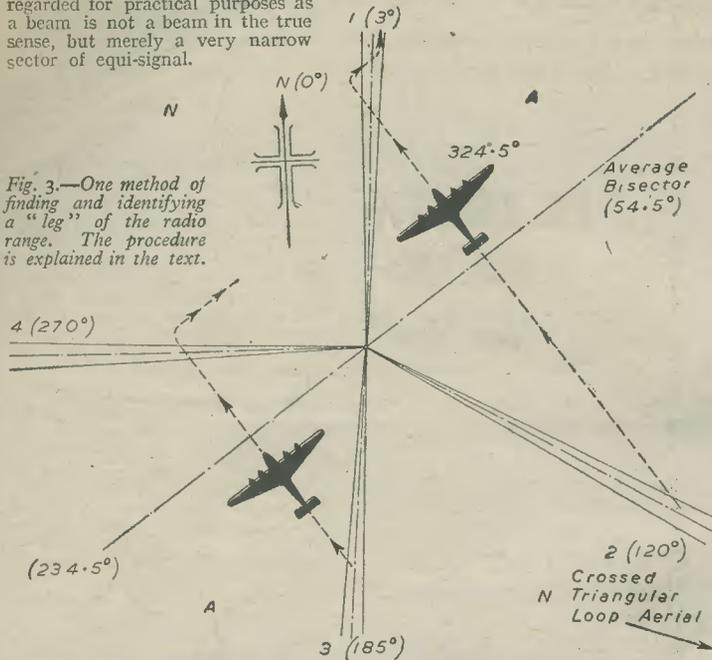
Fig. 3.—One method of finding and identifying a "leg" of the radio range. The procedure is explained in the text.
