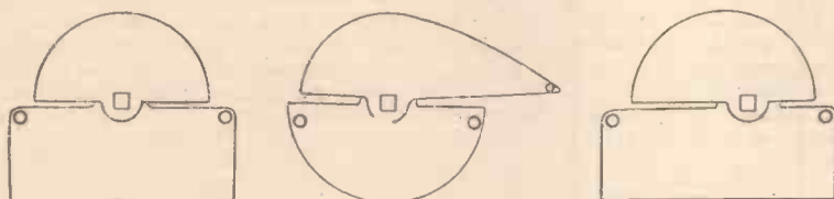
Fig. 1.—Condenser vanes have been produced with various shapes to follow special laws—as shown here.
