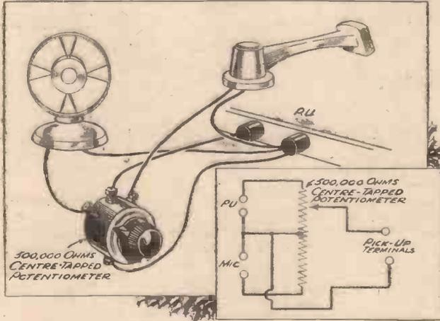
Fig. 5.—“Fader” connections, using a centre-tapped potentiometer.
