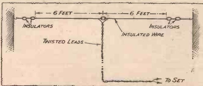
Fig. 2.—A suitable doublet aerial for use below 10 metres.
