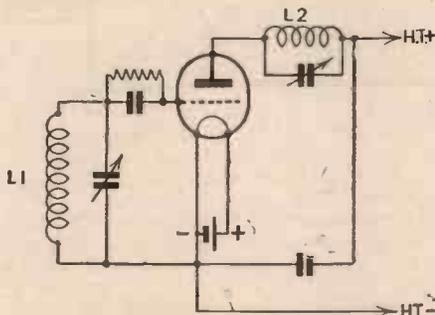
Fig. 5.—The circuit shown here is the tuned-plate tuned-grid arrangement.
