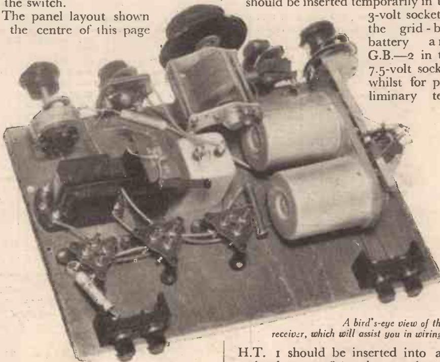
A bird's-eye view of the receiver, which will assist you in wiring.
