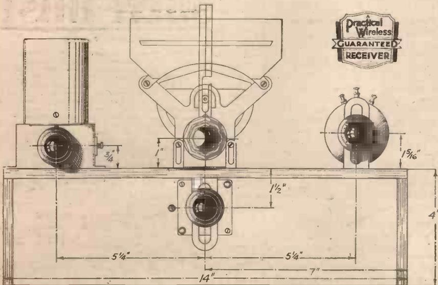
Layout of the controls, with dimensions for panel drilling.
