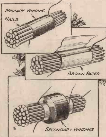
Fig. 1.—A quickly-made L.F. transformer.
