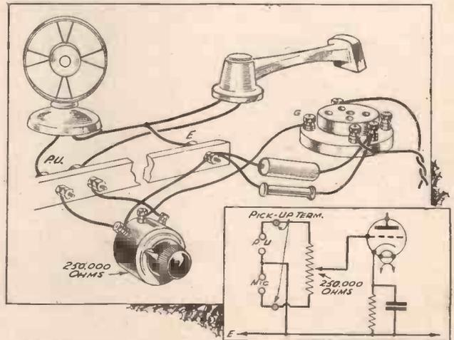
Fig. 4.—Connections similar to those in Fig. 3, but for a mains set.
