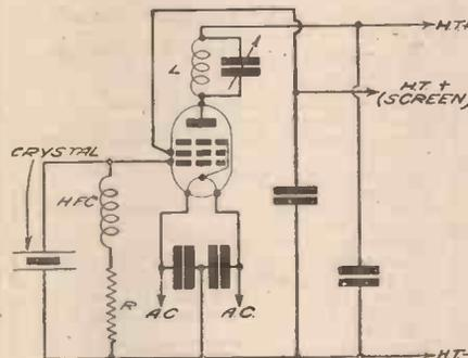
Fig. 5.—Pentode oscillator—crystal controlled.
