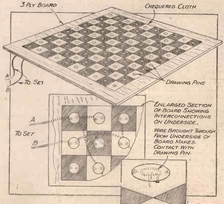
Fig. 2. An easily made electrical board which can be used with the wireless set to provide entertainment and amusement.
