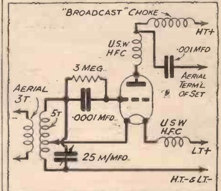
Fig. 3.—Circuit for an electron-coupled oscillator type of superhet converter.
