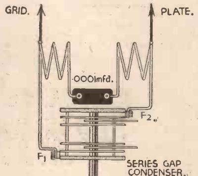
Fig. 3.—Practical arrangement of the Colpitts tuning circuit.
