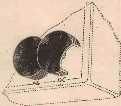
A safety device for two selector-switch controls.
