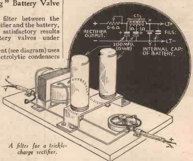
A filter for a trickle-charge rectifier.
