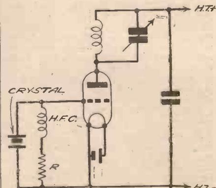
Fig. 4.—Simple triode crystal-controlled circuit
