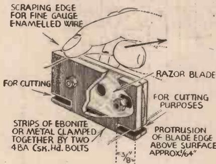
A handy wire-cutter and scraper made with an old razor blade.
