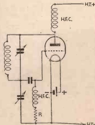
Fig. 4.—This is the Ultraudion circuit.
