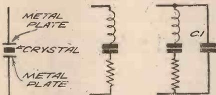
Fig. 1.—Theoretical symbol of the crystal with its electrical circuit equivalents.
