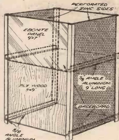
Fig. 8.—Containing case for the transmitter.
