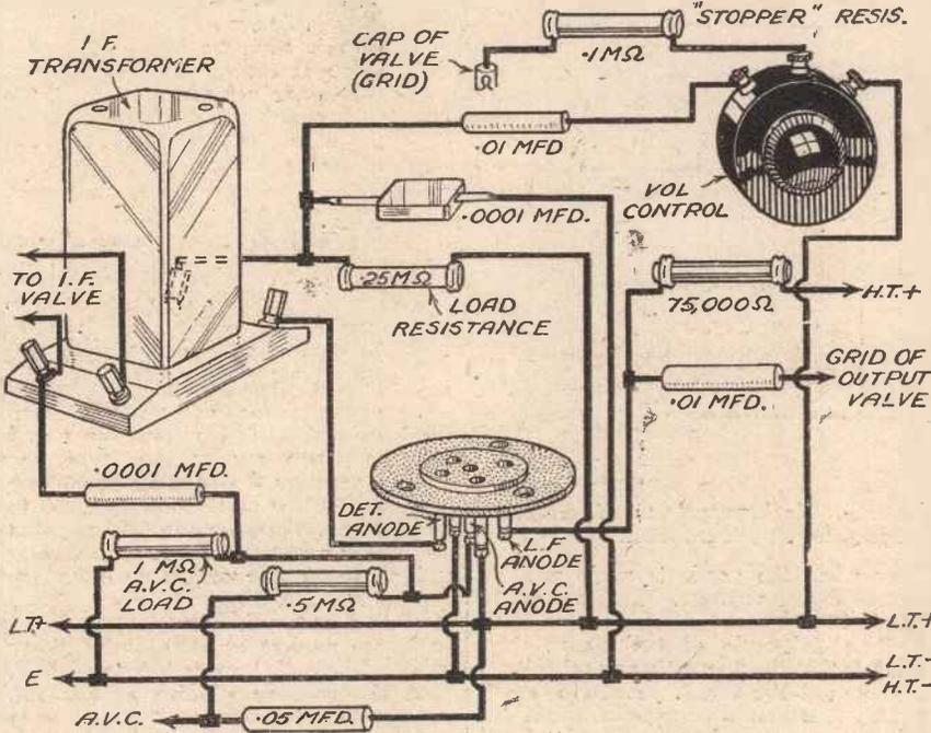
Fig. 3.—Connections for a double-diode-triode used as second detector, A.V.C., and first L.F. amplifier.
