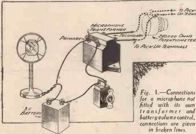
Fig. 1.—Connections for a microphone not fitted with its own transformer and battery volume control, connections are given in broken lines.
