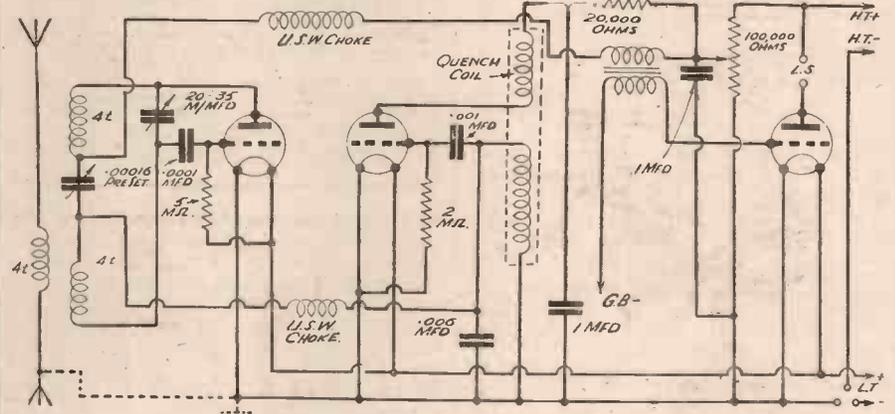
Fig. 4.—A three-valve super-regenerative receiver shown for use with a doublet aerial.
