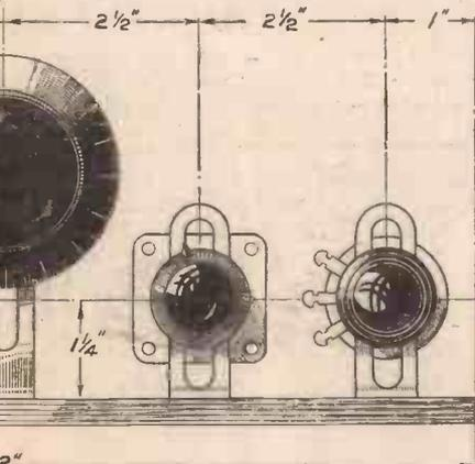
Positions and for drilling the panel or cabinet.
