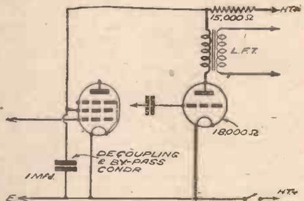
Fig. 4.—How the detector valve and its decoupling resistance can together be used as an S.G. potentiometer. The artificial potentiometer is shown in heavy lines.
