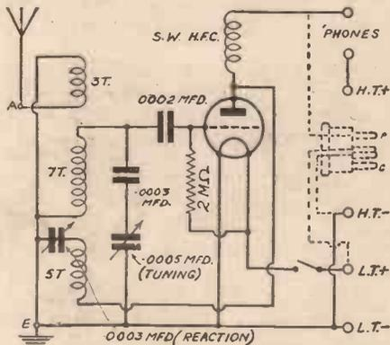
Fig. 1. Theoretical circuit of the simple one-valve set
