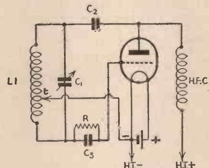
Fig. 1.—The standard Hartley circuit.
