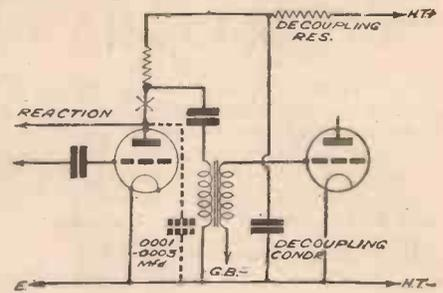
Fig. 2.—When a resistance-fed transformer is used as shown here, an H.F. choke is rarely essential, especially if a small by-pass condenser is connected as shown in broken lines. The H.F. choke, when used, is included at a point marked X.
