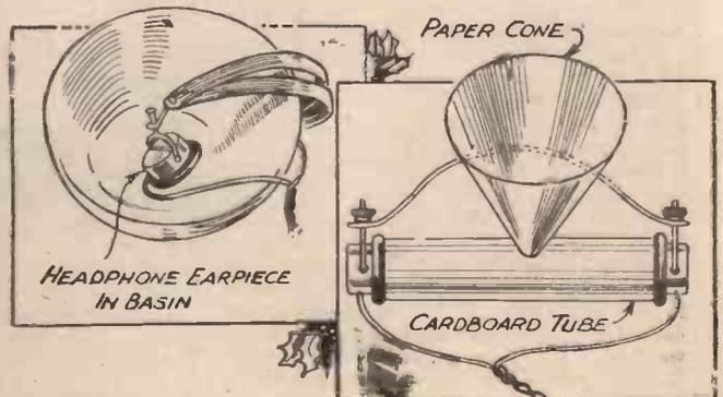
Fig. 3 right.—Improvvised loudspeakers in which ordinary headphones are employed.
