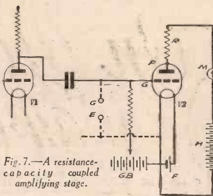
Fig. 7.—A resistance-capacity coupled amplifying stage.
