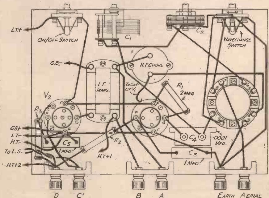
Fig. 2.—Wiring diagram of the receiver.
