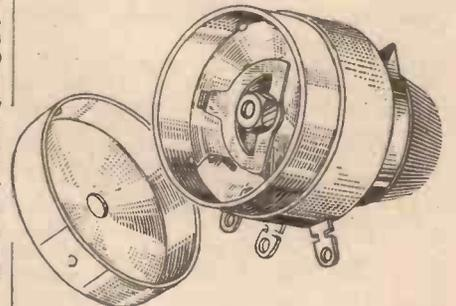
This illustration shows the construction of the Bulgin three-watt volume controls.
