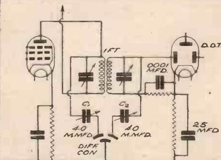
How a differential condenser can be incorporated in a circuit for variable selectivity purposes.
