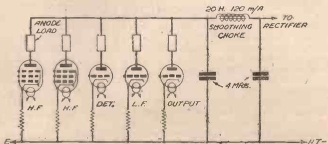
Fig. 5.—A single, expensive smoothing choke used to supply all the valves.
