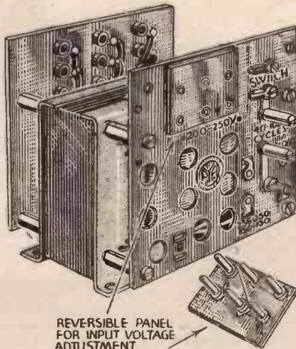
REVERSIBLE PANEL FOR INPUT VOLTAGE ADJUSTMENT.
