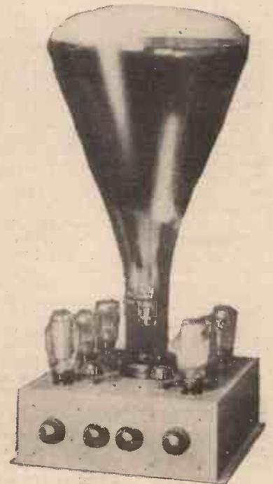
The time base unit with cathode-ray tube in position.
