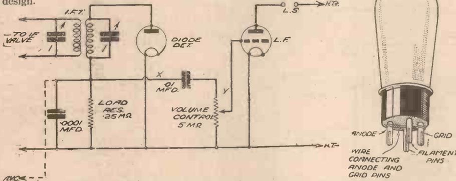
Fig. 1.—The simplest form of diode used as second detector. As shown in the pictorial diagram a triode can be used as a diode by joining together the grid and anode.
