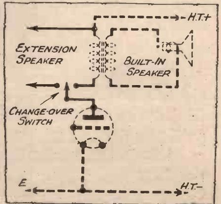
Fig. 4.—How a change-over switch can be used when employing the arrangement shown in Fig. 3.
