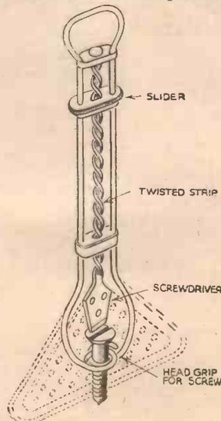
A handy screwdriver tool made from an old rotary whisk.
