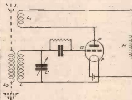
Fig. 8.—The simplest valve oscillator circuit.
