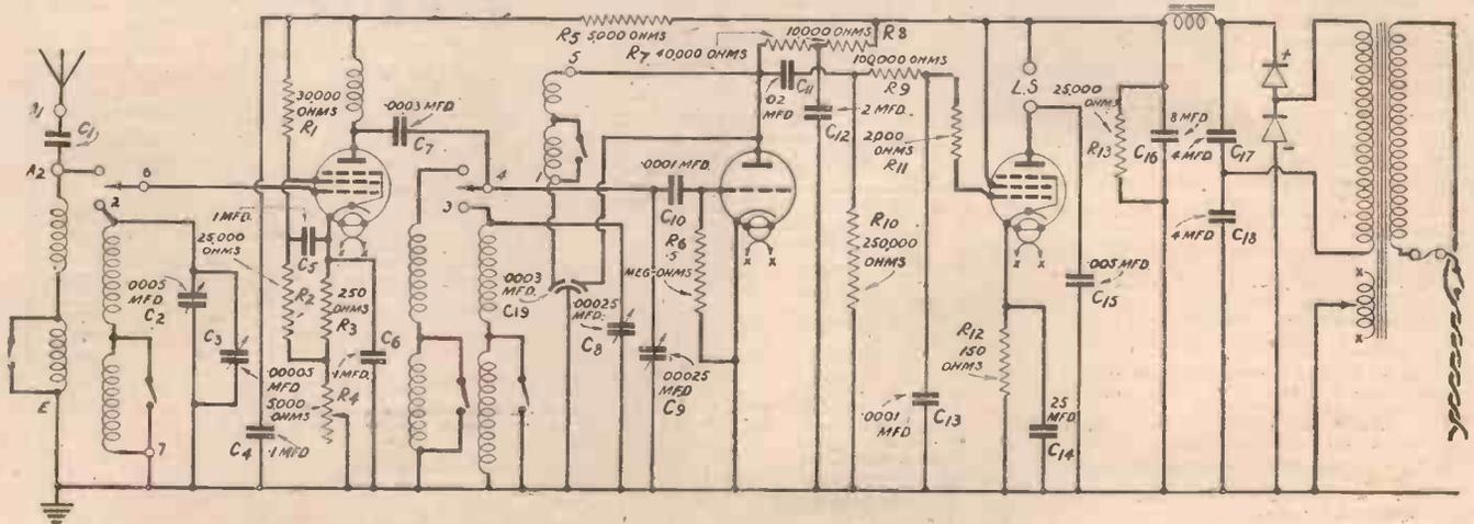
*The theoretical circuit diagram of the Mains Record All-wave Three.*
