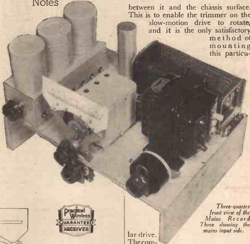
Three-quarter front view of the Mains Record Three showing the mains input side.
