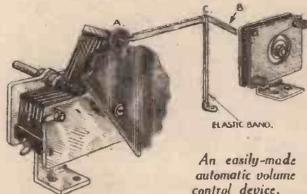
An easily-made automatic volume control device.
