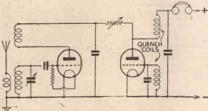
Fig. 1.—The simple super-regenerative receiver with separate quench valve.
