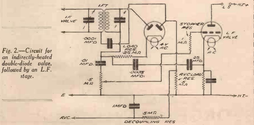
Fig. 2.—Circuit for an indirectly-heated double-diode valve, followed by an L.F. stage.
