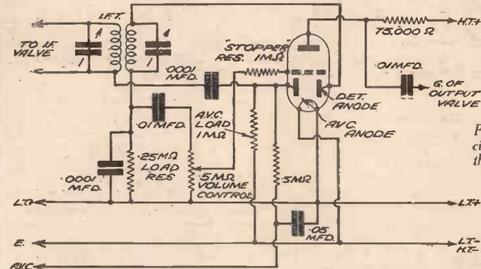
Fig. 4.—Theoretical circuit diagram of the arrangement shown in Fig. 3.
