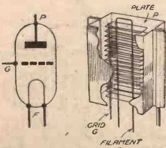
Figs. 4. & 5.—Theoretical and practical assembly of the triode valve.
