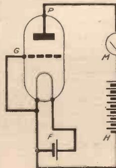
Fig. 6.—The complete circuit of a triode to show the flow of current as mentioned on the next page.
