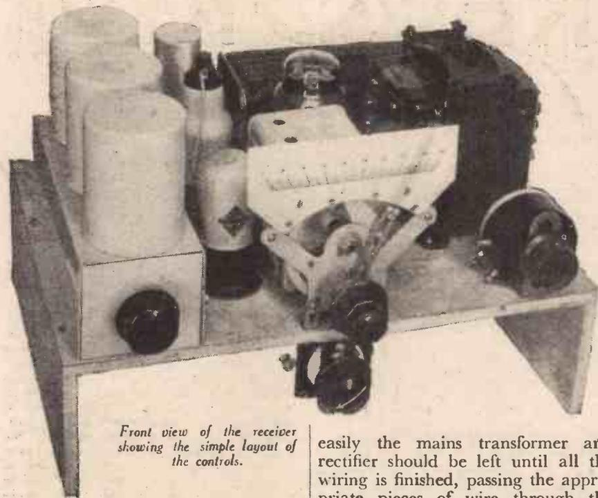
Front view of the receiver showing the simple layout of the controls.
