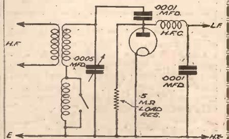
Fig. 5.—Connections for a diode in a "straight" circuit.
