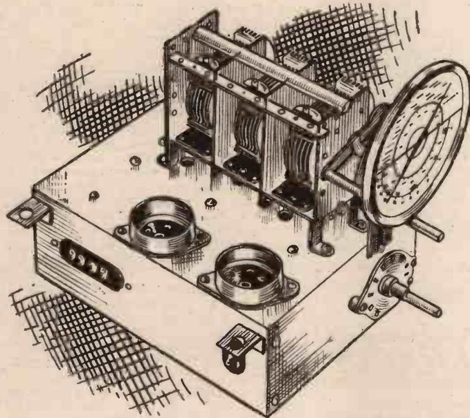
The Radio-Heart tuning unit, consisting of all components ready wired for the H.F. and frequency changing stage of a Superhet.
