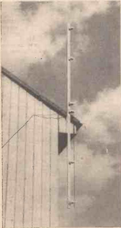
Fig. 1.—Ordinary batten fitted with simple stand-off insulators forms the basis of this dipole aerial arrangement.
