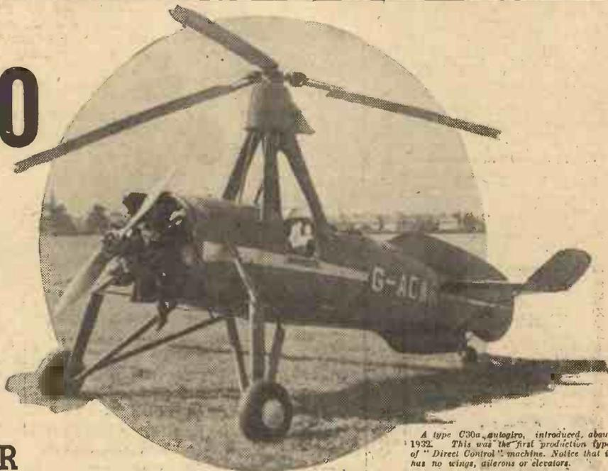
A type C300 autogiro, introduced about 1932. This was the first production type of "Direct Control" machine. Notice that it has no wings, ailerons or elevators.
