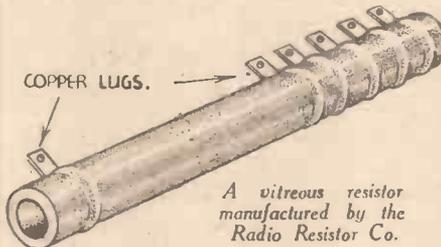
A vitreous resistor manufactured by the Radio Resistor Co.
