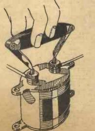
Fig. 2.—An ordinary pen-knife may be used as a temporary short-circuiting device.
