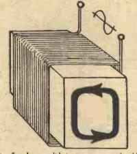
Fig. 3.—In a solid iron core, considerable eddy current losses are induced by the alternating magnetic field.
