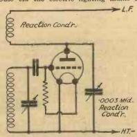
Fig. 2.—Series-fed reaction circuit.
