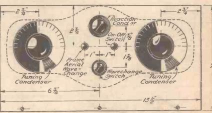
Fig. 1.—This sketch shows the disposition of the panel controls.
