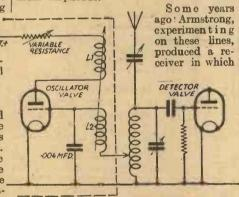
Fig. 1.—A simple regenerative arrangement.
