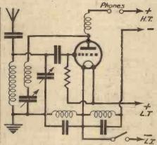
Fig. 6.—Circuit of the Armstrong Super-Regenerative single valver.
