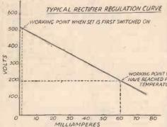
Fig. 1.—Typical rectifier regulation curve
