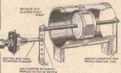
Fitting an adjustable reaction coil.
