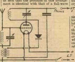
Fig. 4 .- An early form of valve-crystal reflex circuit.
