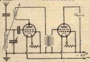
Fig. 8.—Circuit of a two-valve set—L.F. high-tension-less receiver.
