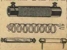
Fig. 2.—Above: Type of resistance which is Centre: How the wire is wound a non-inductive wire resistance, and Below: Two other non-inductive resistances.
