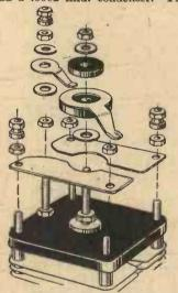
Fig. 1.—Component parts showing order of assembly for reaction switch.
