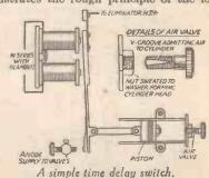
The cylinder can be copper tube with a washer sweated on one end, and a nut sweated over the hole in the washer. A terminal screw with a tapering V-groove filed in, controls the amount of air entering the dashpot, and therefore the time delay. The piston may be made of wood with a
