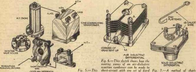
.0003 MHJ DIFFERENTIAL CONDENSER diagram shows the practical wiring details for the arrangement shown in Fig. 4.
