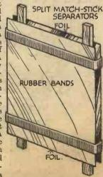
accomplished Fig. 4.—An assembly (Ctd. on page 594) electrolytic cell elements.
