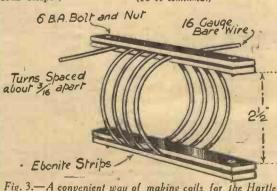
made by using proportionately Fig. 3.—A convenient way of making coils for the Hartley circuit.
