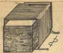
Fig. 6.—A combination of the two methods, arranging a mixture of iron particles and insulating material in very thin layers on an insulating material.
