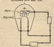
Fig. 5.—This diagram explains the principle of the two-electrode valve.
