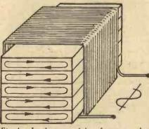
Fig. 4.—In the case of low frequency, these eddy current losses can effectively be avoided by building up the core of many sheet iron laminations. As the eddy current losses are increasing with the square of the frequency this method cannot be transferred to high frequency.
