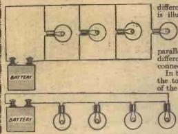
Fig. 3.- Above: Shows a set of lamps connected Fig. 3.—Above: Shows a set of lamps connected the same, but the voltage across in parallel. Below is shown the series arrangement. each one depends on its resistance See Parallel Connections.
