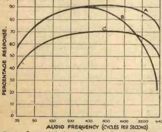
Fig. 1.—Curves which show the response of a receiver to various and Tone Control, audio-frequencies; they are fully explained in the text.
