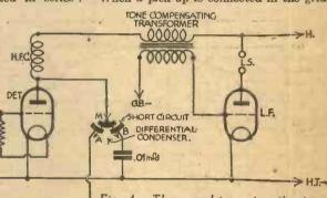
Fig. 4 .- The complete automatic tonecompensating circuit described on this page.
