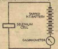
Fig. 5.—A simple selenium cell circuit.
