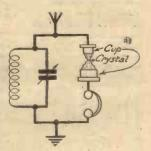
been in use for Fig. 4.—Simple circuit using some time a crystal detector.
