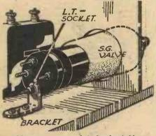
Mounting a screened-grid valve holder.
