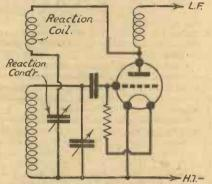
Fig. 1.—Parallel-fed reaction circuit.
