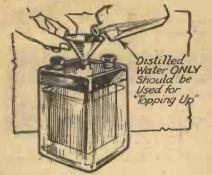
Fig. 4.—Never add acid when "topping" up accumulators.
