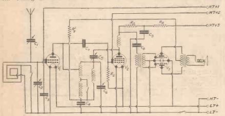
Fig. 3.—Circuit diagram of the Arcady Portable Three. The values of components are as follow:—C1, .0003 mfd. pre-set; C2, .0005 mfd. variable; C3, 1 mfd.; C4, 1 mfd.; C5, .0002 mfd. variable; C6, .0005 mfd. variable; C7, .0002 mfd.; C8, 1 mfd.; C9, 2 mfd.; C1, .0002 mfd.; C8, 1 mfd.; C9, 2 mfd.; C1, .0002 mfd.; C2, 2 mfd.; C3, 2 mfd.; C4, 2
