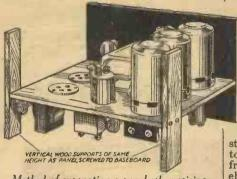
Method of supporting a panel when wiring.
