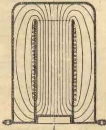
Fig. 1.—An air coil has a weak magnetic field, the lines of force are strayed out and many turns of wire are required to attain certain amount of inductance.
