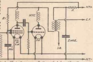
Fig. 1.—Illustrating a very effective method of providing the screeninggrid potentials for an S.G. or V.-M. valve. The detector valve and its anode feed resistance form two "arms" of a potentiameter.
