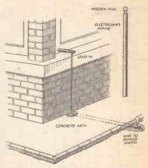
Method of installing an earth lead.
