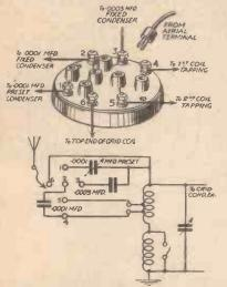
A selectivity adjuster made from a 6-pin base.
