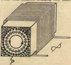
Fig. 5.—A core made of iron particles mixed with insulating material. It is impossible absolutely to insulate the particles and prevent eddy current losses in this way, as there are forming dielectric displacement currents due to capacitive coupling between the particles.
