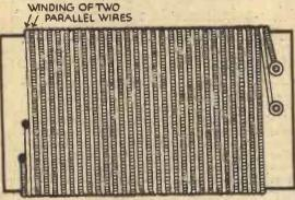
FREE ENDS WAXED Fig 1.—A cell ready to receive IN POSMION. its selenium coating.
