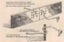
Securing battery leads without terminals.
