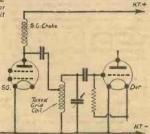
Fig. 3.—The choke used in the anode circuit of an S.G. valve must have a much higher inductance than an ordinary "reaction" choke.
