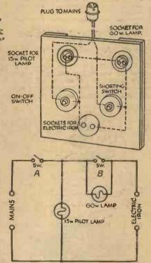
Switchboard arrangement for protecting an electric soldering iron.
