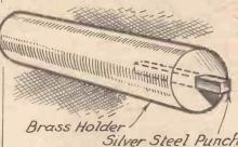
Fig. 4.—Punch for making the holes.
