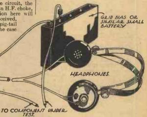
Fig. 4.—Testing components for continuity
