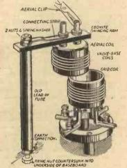
An efficient inductive coupling device.
