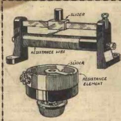
Fig. 3.—Above, a simple form of potentiometer, and below, the more usual type.
