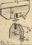
Method of fixing fibre pieces for holding the wire.
