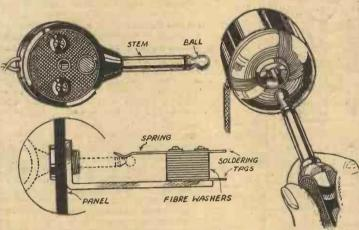
Fig. 1.—Plugs and jacks, showing how the tip and stem of the plug makes contact. known, as
