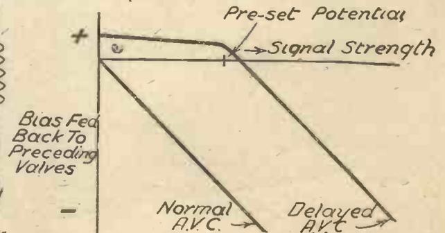
Fig. 5.—How the delayed automatic volume control differs from normal A.V.C.
