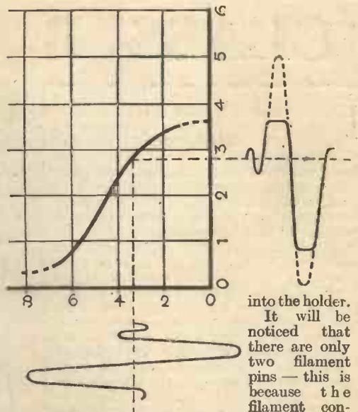
Fig. 2—The effect of grid current shown in diagrammatic form.
