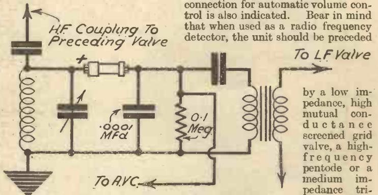
Fig. 2.—A Westector arranged as an R.F. detector.
