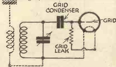
Fig. 4.—This diagram shows the complete grid circuit of the first valve.
