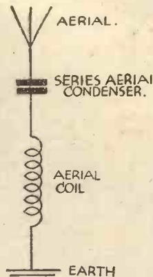
Fig. 2.—The aerial-earth circuit.
