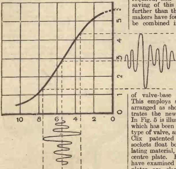
Fig. 1—The curve of a valve biased to give even amplification. The lower line gives grid volts, and the right-hand line gives anode current.
