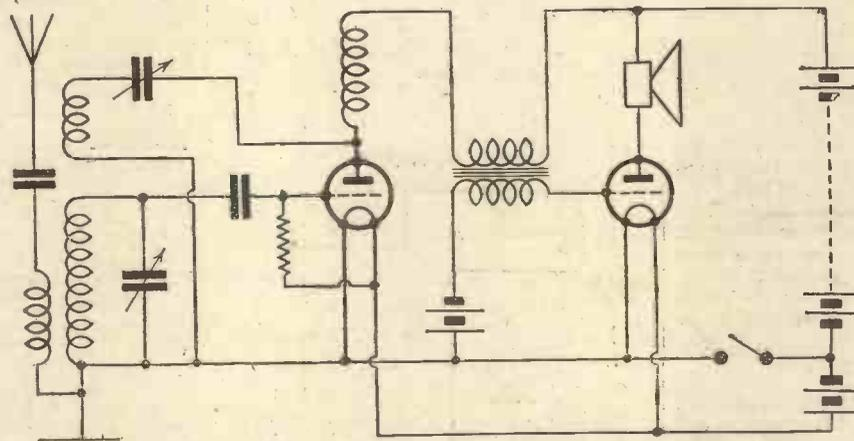
Fig. 1.—The complete circuit of a simple two-valve receiver having detector and low-frequency valves.
