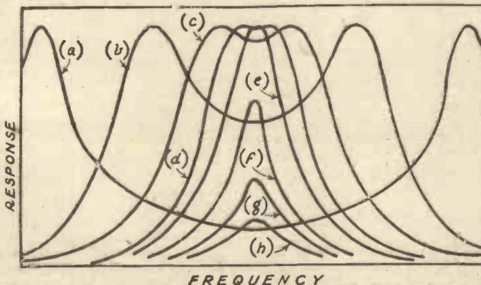
Fig. 1.—Resonance curves of a coupled circuit with various degrees of coupling.
