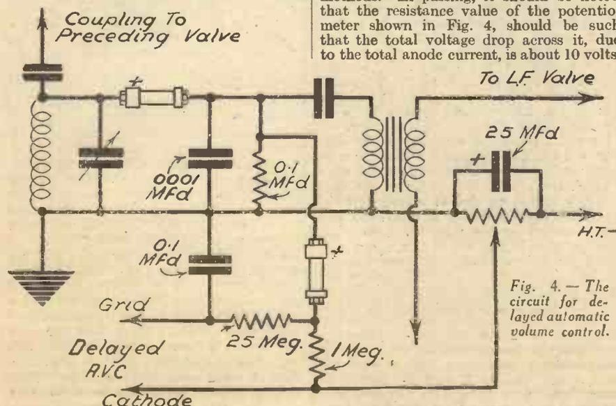
Fig. 4.—The circuit for delayed automatic volume control.
