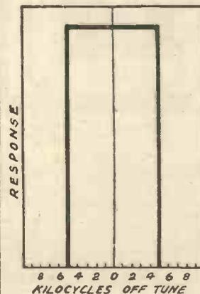
Fig. 2.—Ideal "curve" for a band-pass tuner.
