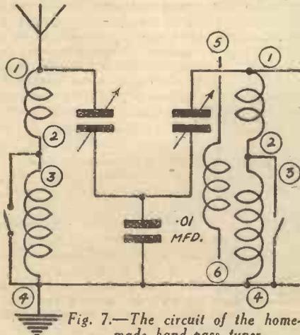
Fig. 7.—The circuit of the home-made band-pass tuner.
