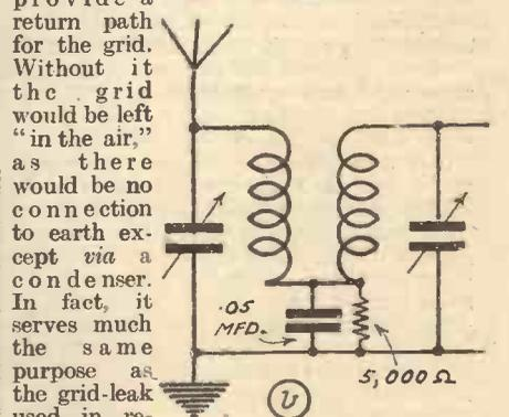
Fig. 5.—Various arrangements for capacitive coupling. (Continued on page 82.)
