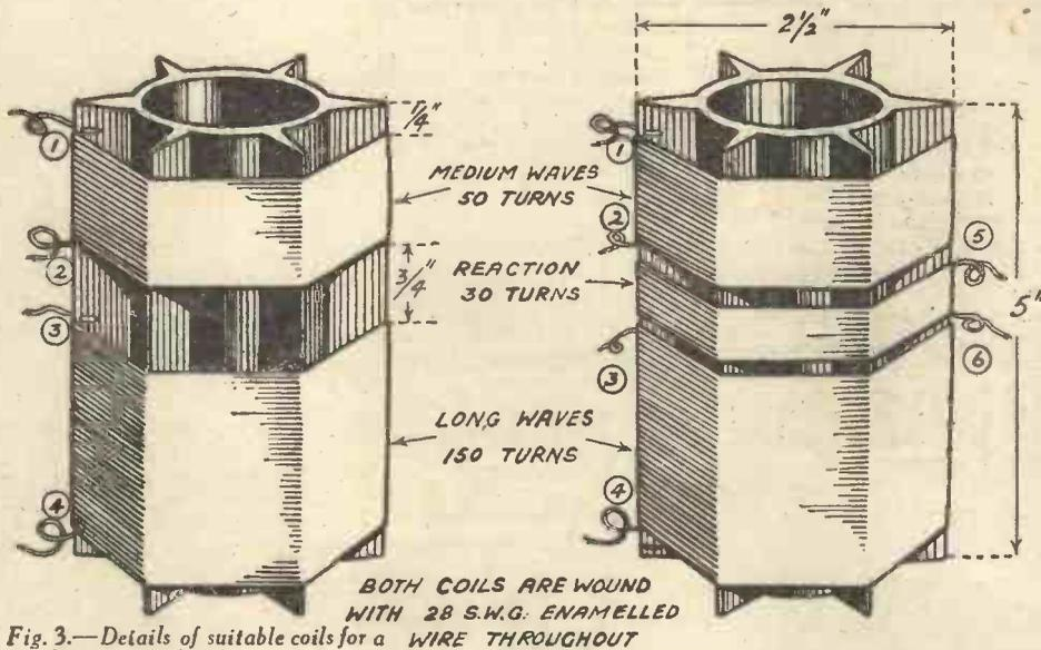
Fig. 3.—Details of suitable coils for a home-made band-pass tuner.
