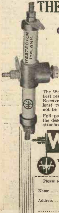
The advent of the Westector brings the ideal detector a step nearer. This development of the Westinghouse Metal Rectifier enables the rectification of radi-frequency currents to be obtained by the use of a copper-oxide detector, which requires no anode or filament current and which is no bigger than a grid leak.
