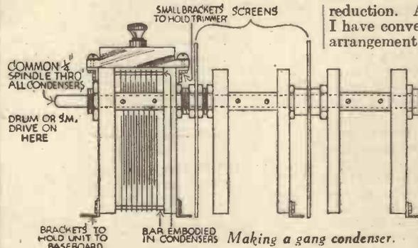
pre-set type of .00001 to .000005 mfd. capacity. I have made a number of these units and the maximum error between any two condensers has never exceeded two degrees on the tuning scale. The trimmers have always proved quite ample to give excellent matching with all rotors set in line. Screws are easily inserted as shown in sketch.—C. J. R. (Birmingham).
