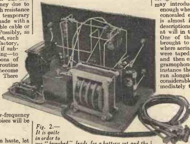
Fig. 2.—It is quite in order to use "bunched" leads for a battery set and the neat effect is shown here.
