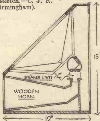
Fig. 2.—Sectional view of speaker.
