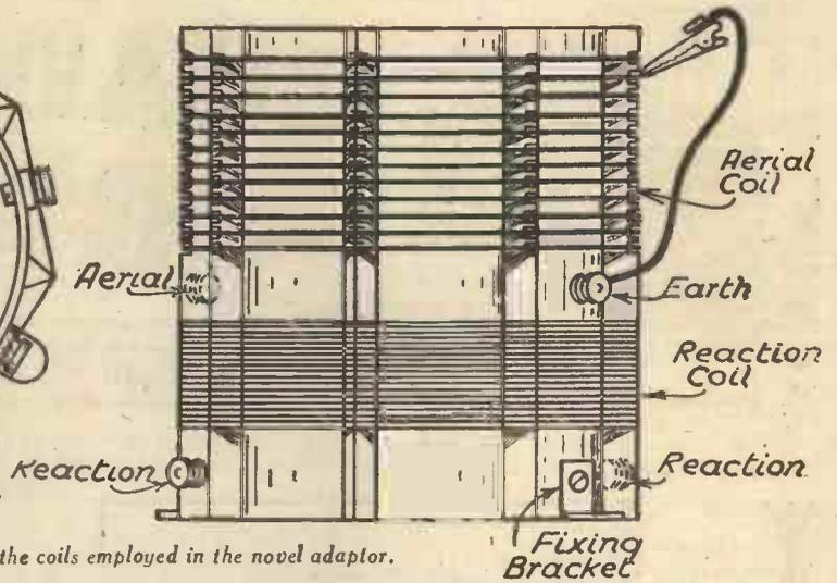
Fig. 3.—Details of the coils employed in the novel adaptor.
