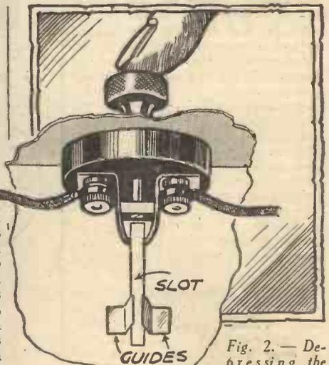
Fig. 2.—Depressing the plunger to release coin and break the circuit.
