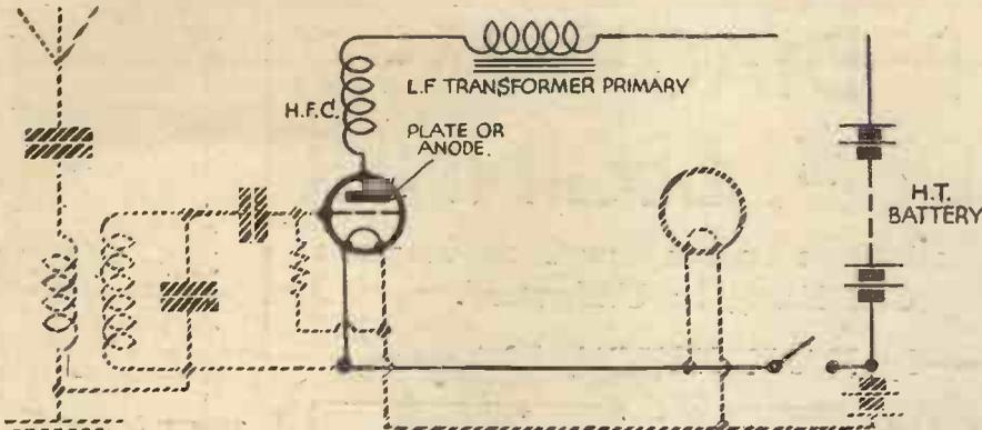
Fig. 6.—The anode and H.F. circuits of the detector valve; notice that the H.T. circuit "overlaps" the filament circuit.
