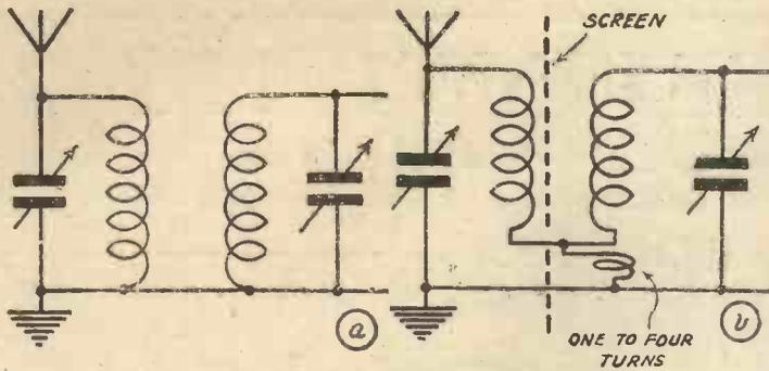
Fig. 4.—Two methods of inductively coupling two circuits.
