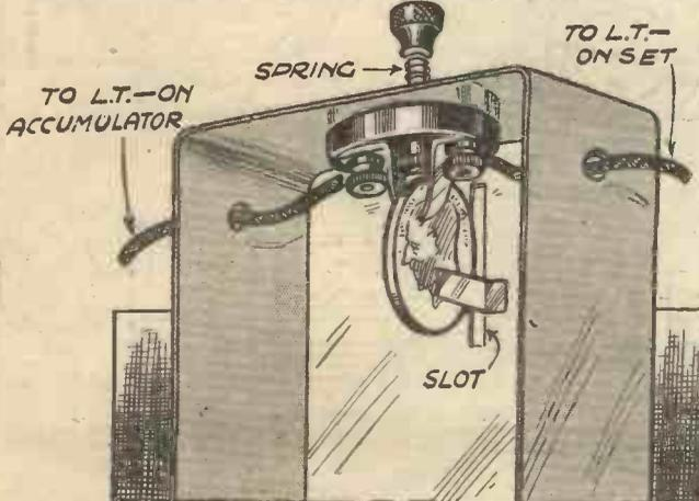
Fig. 1.—A simple coin-operated radio switch showing how a penny completes the circuit.
