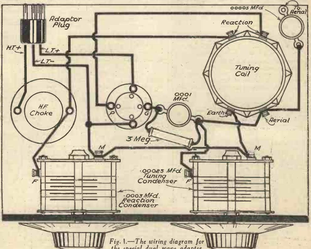
Fig. 1.—The wiring diagram for the special dual wave adaptor.
