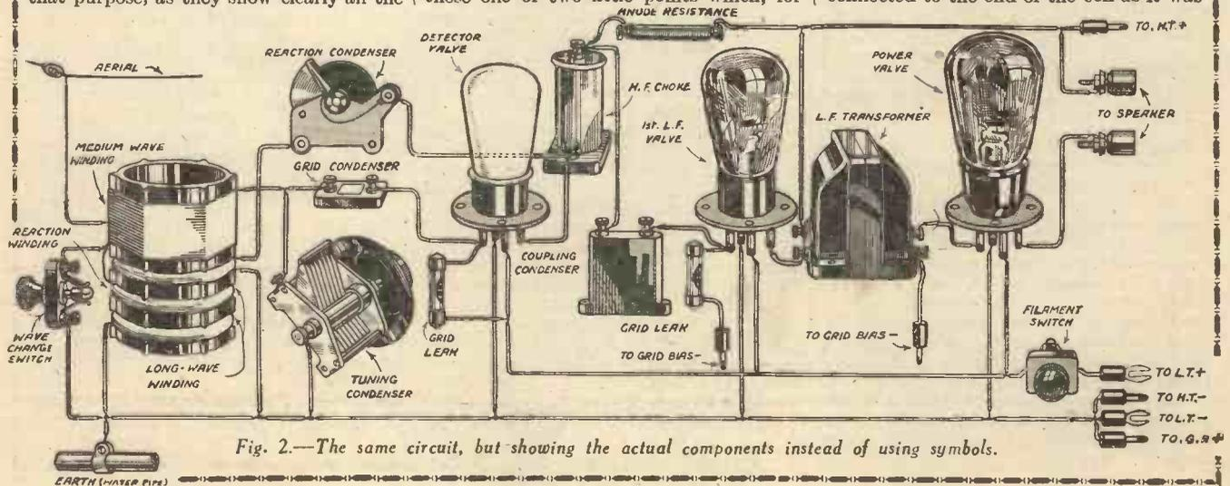
Fig. 2.—The same circuit, but showing the actual components instead of using symbols.
