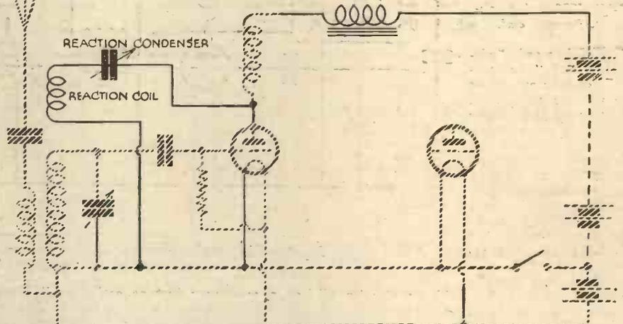
Fig. 7.—Here we see the path of the high-frequency currents which provide reaction.
