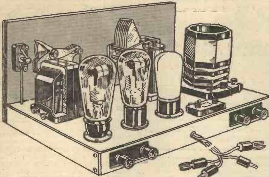
Fig. 3.—How the various parts are mounted on the "chassis" to form the complete receiver.
