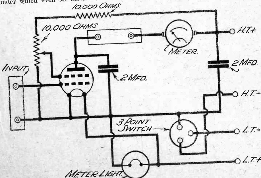
Fig. 2.—Theoretical circuit of the valve voltmeter.
