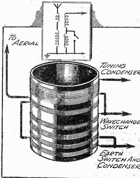
Fig. 1.—Showing aerial transformer coupling.
