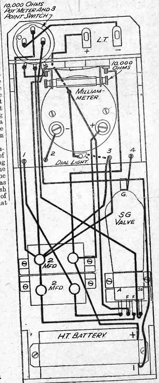
Fig. 3.—Wiring diagram showing all the connections.
