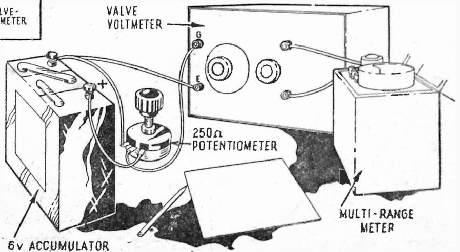
Fig. 2.—Adjusting the zero reading.
