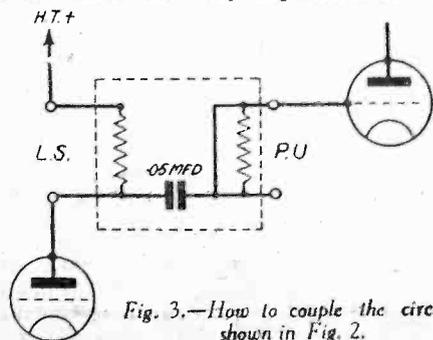
Fig. 3.—How to couple the circuits shown in Fig. 2.
