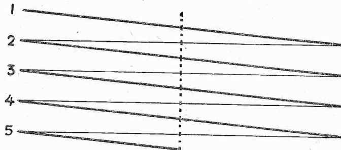
Fig. 2.—Showing how the first section of an intercalated scan is built up in a similar manner to the orthodox, or sequential, system.
