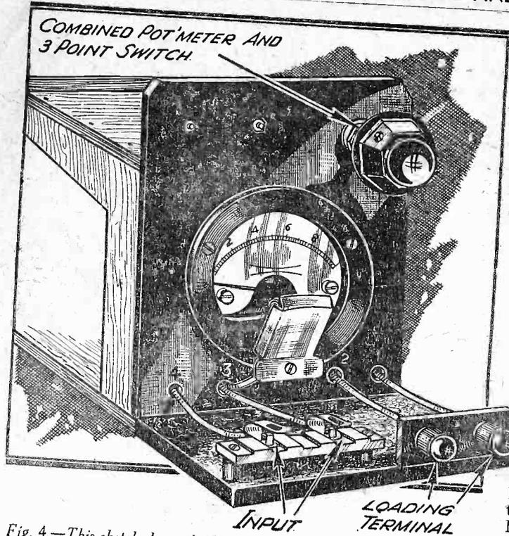
Fig. 4.—This sketch shows the front of the instrument and the connections to the input and loading terminals.
